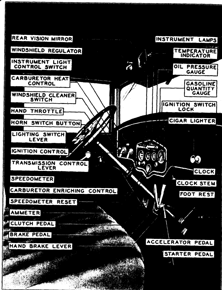
Figure 1. The new driver should familiarize himself with the instruments and controls before attempting to drive.
