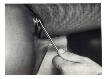
Fig. 409 - Removing rear seat back rest.
