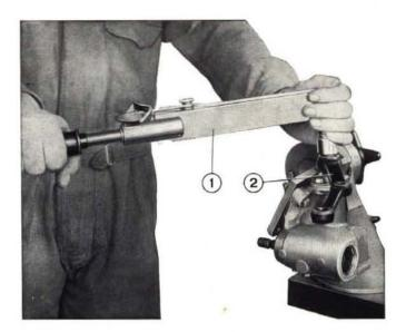
Fig. 283 - Installing pitman arm. 1. Torque wrench. - 2. Pitman arm.
