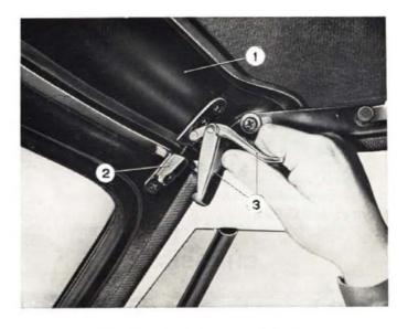
Fig. 518 - Fastening top at front. 1. Top front cross rail. - 2. Top front catch. - 3. Top front catch clamp and lever.
