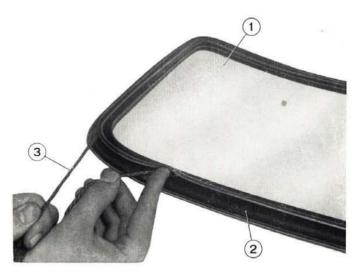
Fig. 406 - Arranging draw cord, preparatory to windshield glass installation.
