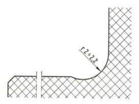
Fig. 67 - Fillet radii for flywheel end main bearing journal shoulder.
