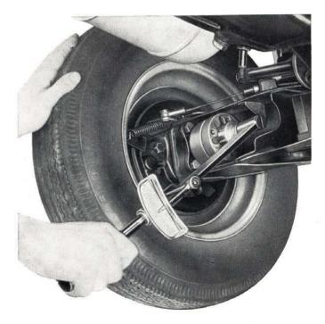
Fig. 261 - Tightening flexible joint mounting nut. The wheel is on for more ease in tightening.
