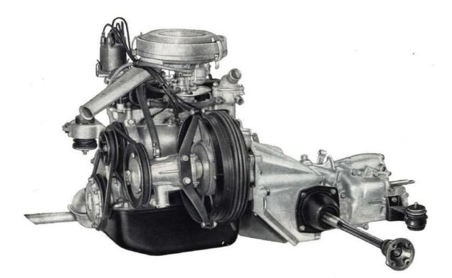
Fig. 141 - Engine transmission and differential assembly.
