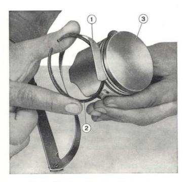
Fig. 47 - Checking piston ring side clearance. 1. Feeler gauge A. 95316. - 2. Piston ring. - 3. Piston.
