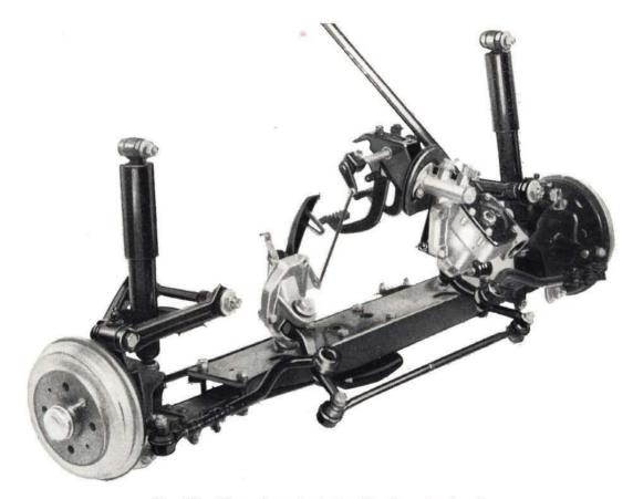
Fig. 240 - View of mechanical units of car front end.
