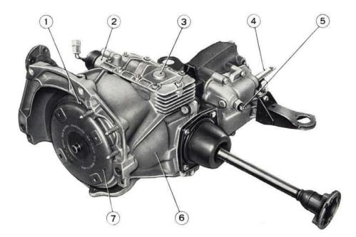
Fig. 562 - Transmission with hydraulic torque converter - right hand view.
