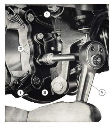
Fig. 457 - Fitting brake caliper.
