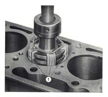
Fig. 30 - Honing cylinder barrels. 1. Hone abrasive stones.
