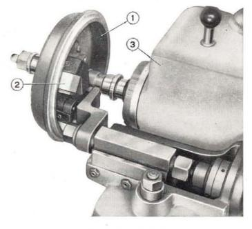
Fig. 296 - Lapping brake drum.
