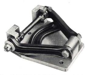
Fig. 218 - Control arm installed on fixture A. 74135.
