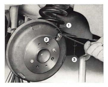
Fig. 541 - Checking shoe-to-drum clearance at right side rear wheel. 1. Brake drum. - 2. Brake shoe with lining. - 3. Feeler gauge A. 95316.
