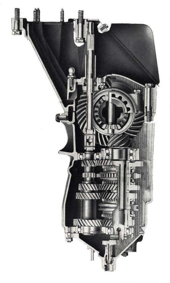
Fig. 163 - Side sectional view of transmission-differential assembly.
