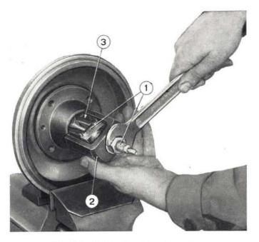
Fig. 224 - Pulling inner bearing cup. 1. Puller A. 47026/1. - 2. Puller bell A. 47026/2. - 3. Bearing cup.
