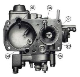
Fig. 149 - Interior view of Solex carburetor body. 2. Air correction jet. - 23. Venturi. - 34. Power pump nozzle. -41. Power pump inlet valve. - 58. Choke jet. - 59. Choke plunger.
