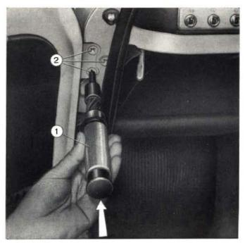
Fig. 398 - Door alignment. 1. Ram screwdriver A. 81011. - 2. Door hinge screws.
