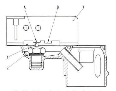
Fig. 151 - Solex carburetor: checking float level. 1. Gauge A. 95126. - 2. Needle valve. - 3. Valve needle. - A-B. Gauge dowels.
