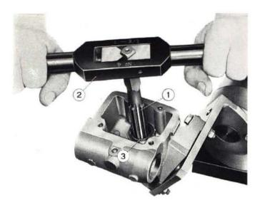
Fig. 281 - Reaming eccentric bushing. 1. Reamer A. 90330/20. - 2. Reamer handle. - 3. Eccentric bushing.
