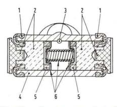
Fig. 289 - Side section view across wheel cylinder.
