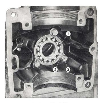
Fig. 192 - Drive pinion ball bearing. 1. Bearing. - 2. Bearing lock plate. - 3. Lock plate screw.
