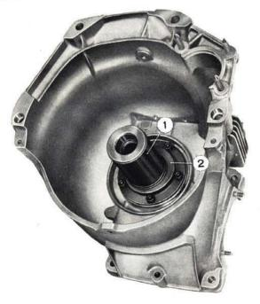
Fig. 580 - Fitting pump oil seal. 1. Service tool A. 70142 for pump seal fitting. - 2. Pump body.
