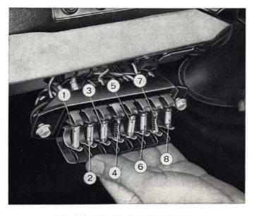
Fig. 369 - Electrical system fuses. 1. Fuse No. 15/54. - 2. Fuse No. 30. - 3. Fuse No. 56/b 1. - 4. Fuse No. 56/b 2. - 5. Fuse No. 56/a 1. - 6. Fuse No. 56/a 2. - 7. Fuse No. 58/1. - 8. Fuse No. 58/2.
