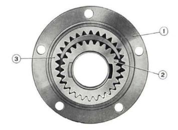
Fig. 578 - Gear type oil pump. 1. Pump body. - 2. Drive gear. - 3. Driven gear.
