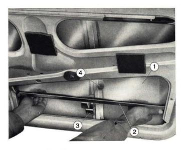
Fig. 393 - Removing drop glass. 1. Glass pane. - 2. Glass bottom channel. - 3. Regulator cable clip. -4. Buffer.
