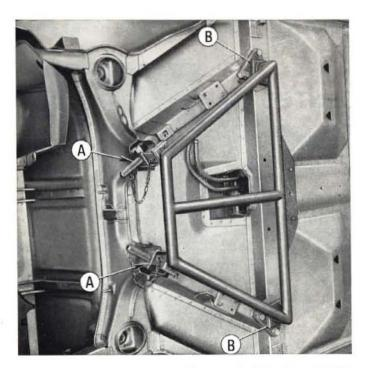
Fig. 413 - Detail showing use of gauge A. 74141 for checking underbody rear.
