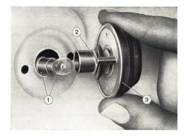
Fig. 364 - Removing side direction signal lamps. 1. Bulb and bulb holder. - 2. Lamp mounting studs. - 3. Lamp.
