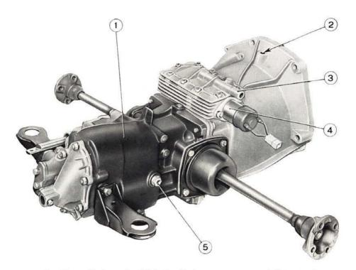
Fig. 561 - Transmission unit with hydraulic torque converter - left hand view. 1. Gearbox. - 2. Seat of guarantee seal. - 3. Oil inlet. - 4. Solenoid. - 5. Gearbox oil level indicator plug.
