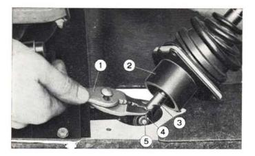
Fig. 207 - Disassembling gearshift lever. 1. Flat-nose pliers. - 2. Gearshift lever support. - 3. Gearshift lever. -4. Gearshift lever pin fastener. - 5. Gearshift lever pin.
