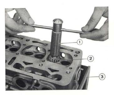
Fig. 94 - Using 75° cutter to narrow valve seats. 1. Spindle A. 94058. - 2. 75° cutter. - 3. Cylinder head holding tool A. 60041.
