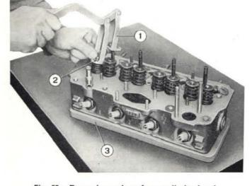
Fig. 85 - Removing valves from cylinder head. 1. Spring compressor A. 60084. - 2. Valve locks. - 3. Supporting plate A. 60283.
