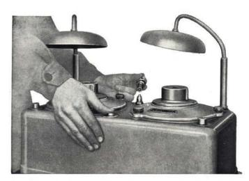
Fig. 356 - Blowing a spark plug after sanding and washing.
