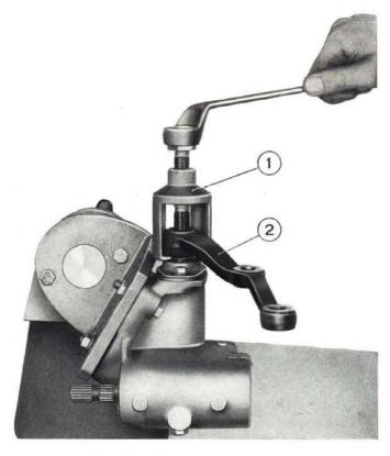
Fig. 276 - Removing pitman arm. 1. Tool A. 47033. - 2. Pitman arm.
