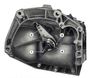
Fig. 158 - Detail of clutch throwout control mechanism.
