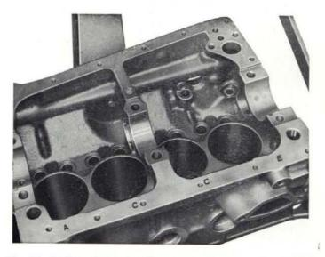
Fig. 29 - Letters showing cylinder bore classes on lower face of cylinder block.
