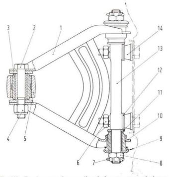
Fig. 219 - Front suspension: sectional view across control arm.
