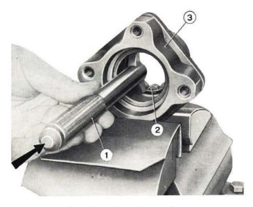
Fig. 247 - Removing roller bearing cup. 1. Driver A. 74034. - 2. Roller bearing cup. - 3. Rear wheel hub.
