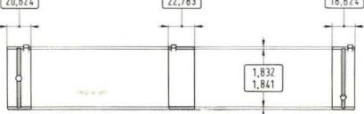
Fig. 75 - Critical dimensions (metric) of crankshaft and main bearing inserts.
