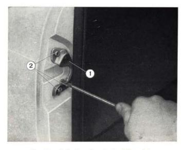
Fig. 399 - Adjusting door lock striker plate. 1. Striker plate. - 2. Striker plate mounting screws.
