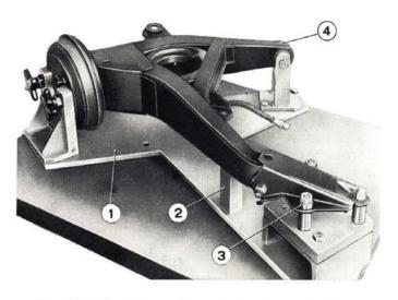
Fig. 249 - Checking control arm and drum assembly. 1. Fixture A. 74142. - 2. Fixture dowel. - 3. Shims, arm to fixture. -4. Control arm.
