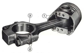
Fig. 54 - Position of piston to connecting rod. 1. Piston skirt class letter and piston boss division number. -2. Connecting rod number. - 3. Oil hole.
