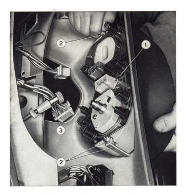
Fig. 469 - Removing instrument cluster. 1. Instrument cluster. - 2. Cluster holding nuts and clamps. -3. Speedo cable.
