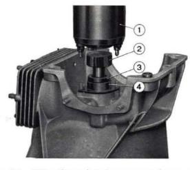
Fig. 577 - Fitting the seal on torque converter support. 1. Press. - 2. Seal centraliser. - 3. Seal. - 4. Torque converter support-
