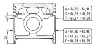
Fig. 421 - Skirt diameter (metric) of 100GC.000 engine measured at class grading points. 5 = .197" - 20 = .787"
