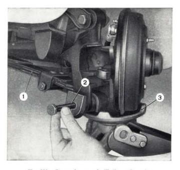
Fig. 211 - Removing semi-elliptic spring pin. 1. Semi-elliptic spring. - 2. Semi-elliptic spring pin. - 3. Hydraulic jack.
