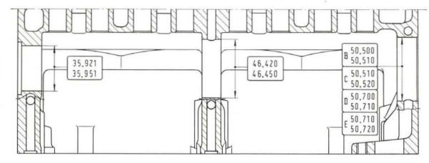
On assembly note the class of the seat and install a bushing belonging to the same class.
