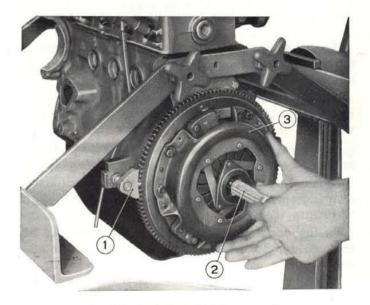
Fig. 25 - Installing clutch assembly. 1. Tool A. 60282. - 2. Guide pin A. 70085. - 3. Clutch assembly.
