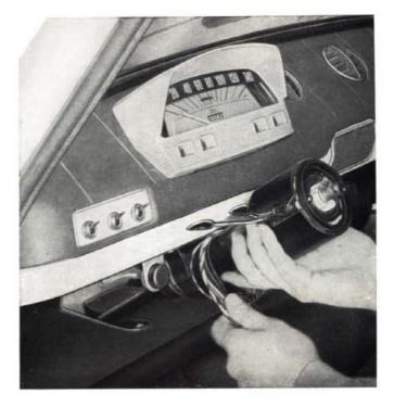
Fig. 374 - Removing direction signal and outer lighting selector switch.
