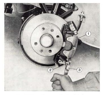
Fig. 450 - Tipping caliper mounting bracket clamps. 1. Brake caliper. - 2. Caliper mounting bracket. - 3. Tool A. 72238.
