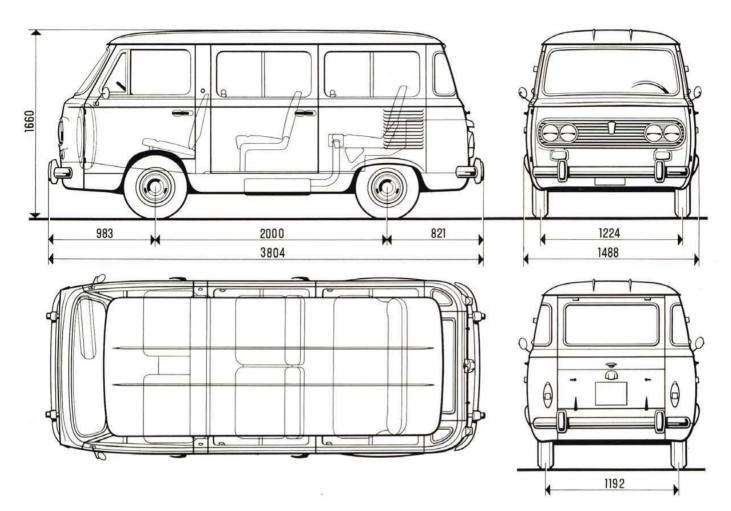
Fig. 521 - Leading dimensions. Overall height applies to an unloaded vehicle.
