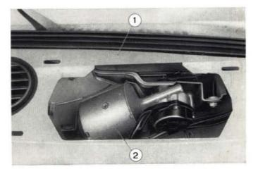
Fig. 375 - Arrangement of windshield wiper. 1. Instrument panel. - 2. Wiper motor.
