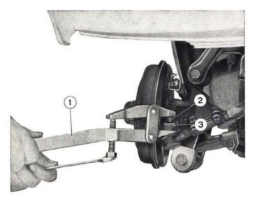
Fig. 210 - Tying off tie rod from knuckle arm. 1. Tool A. 47035. - 2. Rod end ball stud. - 3. Knuckle arm.
