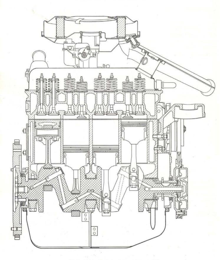
Fig. 26 - Side sectional view of engine across cylinders.
