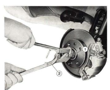
Fig. 458 - Staking wheel hub nut. 1. Hub nut. - 2. Nut staking tool.
