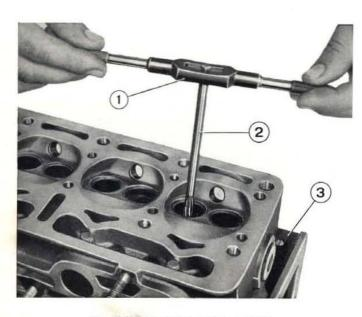
Fig. 104 - Reaming valve guides. 1. Reamer handle. - 2. Reamer A. 90313. - 3. Head holding tool A. 60041.
