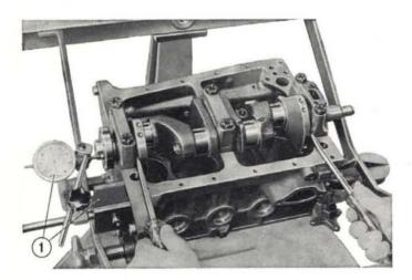
Fig. 80 - Checking crankshaft end play. 1. Magnetic dial indicator.
