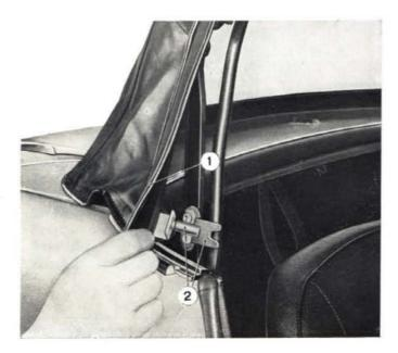
Fig. 517 - Securing canvas top on sides. 1. Top. - 2. Lock pin and plate holding top side.
