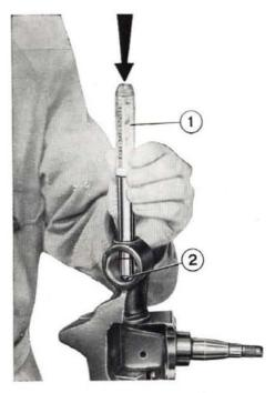
Fig. 226 - Installing kingpin. 1. Driver A. 74014. - 2. Kingpin.
