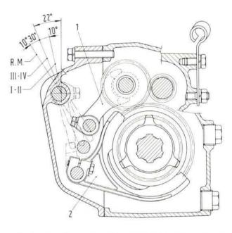
Fig. 185 - End sectional view of transmission across shifter rail. 1. Reverse shifter fork. - 2. First and second shifter fork. R.M. = Reverse.
