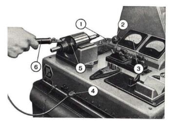
Fig. 324 - Testing generator armature for open coils. 1. Armature tester throw-in switch. - 2. Tester warning light. -3. Ammeter. - 4. Ammeter plug. - 5. Armature. - 6. Twin contact insulated grip. In correspondence with an open coil the ammeter reading will be zero.
