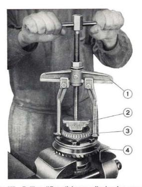
Fig. 187 - Pulling differential cage roller bearing cones. 1. Puller A. 40005/2/6. - 2. Puller item /20 B. - 3. Roller bearing cone. - 4. Ring gear.
