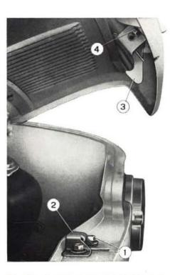
Fig. 402 - Engine compartment lid catch.
