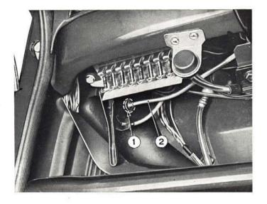
Fig. 382 - Detail showing the arrangement of the antenna cable in car interior.
