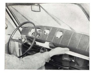
Fig. 410 - Removing instrument panel lining.
