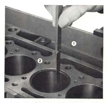
Fig. 48 - Checking end gap of piston rings in cylinder. 1. Feeler gauge A. 95118. - 2. Piston ring.
