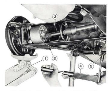
Fig. 255 - Securing rear control arm to body shell.
