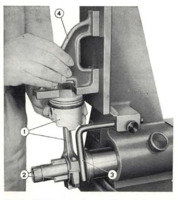
Fig. 59 - Checking connecting rod-piston and pin assembly for misalignment.
