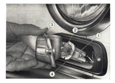
Fig. 363 - Opening front parking lamp. 1. Bulb holder. - 2. Bulb. - 3. Lens. - 4. Gasket.
