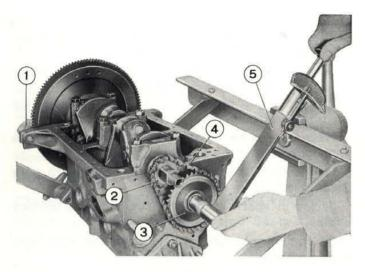
Fig. 19 - Tightening camshaft driven sprocket screw. 1. Tool A. 60282. - 2. Drive sprocket. - 3. Driven sprocket. - 4. Timing chain. - 5. Torque wrench.
