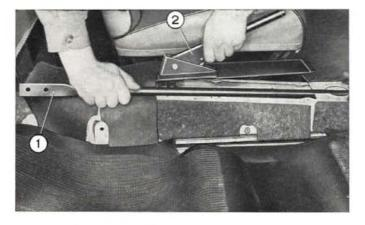
Fig. 208 - Removing selector lever rod. 1. Selector lever rod. - 2. Handbrake ratchet lever and support.
