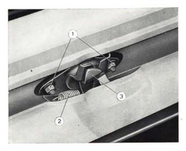
Fig. 400 - Front compartment lid catch. 1. Catch mounting nuts. - 2. Catch hook return spring. - 3. Catch hook.
