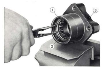
Fig. 252 - Installing roller bearing snap ring. 1. Bearing cup. - 2. Bearing snap ring. - 3. Rear wheel hub.
