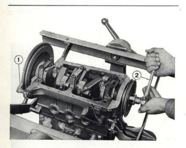
Fig. 13 - Backing out hub-pulley lock screw. 1. Flywheel stop A. 60282. - 2. Ratchet wrench A. 89854.
