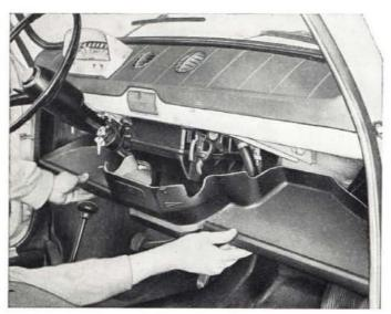
Fig. 306 - Withdrawing utility shelf.
