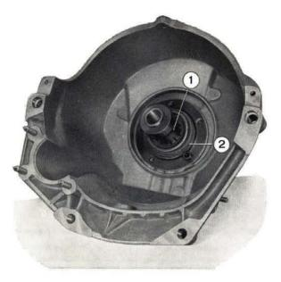
Fig. 579 - Centralising the oil pump. 1. Oil pump centraliser tool A. 70145. - 2. Pump body.
