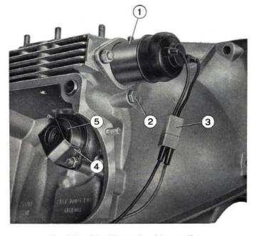
Fig. 585 - Checking solenoid operation.
