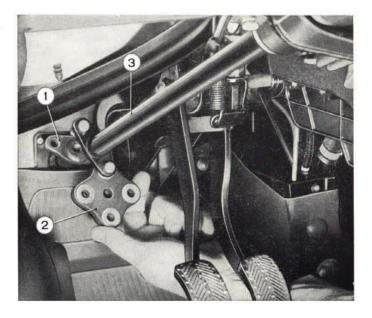
Fig. 446 - Removing steering column joint. 1. Lower steering shaft. - 2. Flexible joint. - 3. Upper steering shaft.
