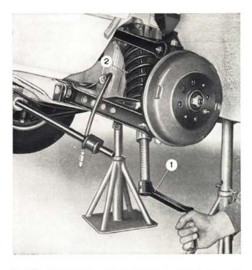
Fig. 526 - Compressing coil spring as a preparatory step to suspension removal.
