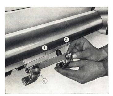
Fig. 366 - Removing license plate lamp. 1. Lamp frame. - 2. Bulb. - 3. Bulb holder.
