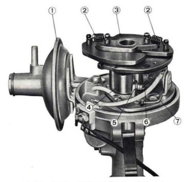
Fig. 352 - Ignition distributor with cover removed.
