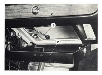
Fig. 514 - Close-up view of utility compartment. 1. Engine compartment lid release control. - 2. Utility drawer, drop type.
