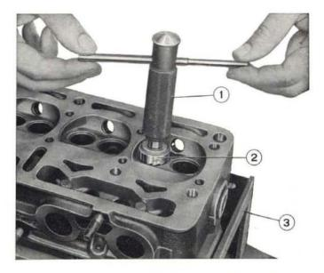
Fig. 93 - Using 20° cutter to narrow valve seats. 1. Spindle A. 94058. - 2. 20° cutter. - 3. Cylinder head holding tool A. 60041.
