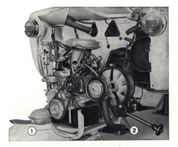
Fig. 10 - Removing engine and transmission assembly. 1. Adapter A. 60531. - 2. Hydraulic jack.
