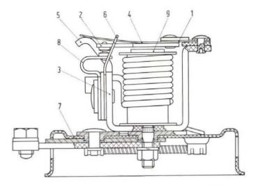
Fig. 335 - Cutout relay for regulator assembly GN 2/12/16. 1. Bi-metallic hinge-spring. - 2. Armature. - 3. Body. - 4. Adjusting spring. - 5. Setting arm. - 6. Armature stop. - 7. Base. - 8. Stationary contact blade spring. - 9. Core.
