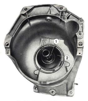
Fig. 582 - Fitting the dust cover. 1. Torque converter support. - 2. Dust cover.
