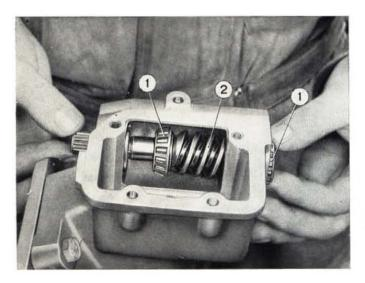
Fig. 282 - Installing steering worm and bearings. 1. Roller bearing cones. - 2. Worm.
