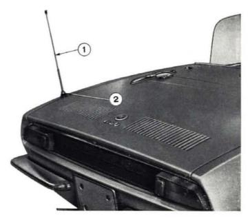
Fig. 504 - Antenna installed on rear fender. 1. Antenna. - 2. Nut, antenna trimmer setting.
