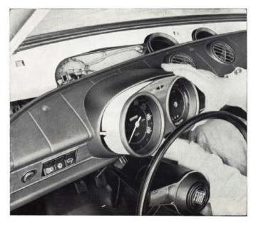
Fig. 471 - Withdrawing instrument cluster from panel lining.
