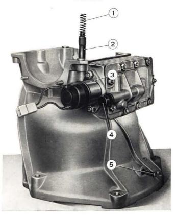
Fig. 592 - Refitting guarantee seal pin. 1. Spring for torque converter output shaft. - 2. Torque converter output shaft. - 3. Solenoid. - 4. Plug. - 5. Pin.
