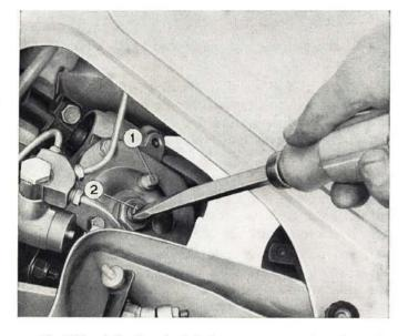
Fig. 279 - Adjusting lash between worm and sector. 1. Oil filler plug. - 2. Sector adjusting screw.
