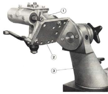
Fig. 275 - Steering gear on service fixture. 1. Steering gear. - 2. Adapter A. 74076/2. - 3. Service fixture A. 74076.
