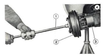
Fig. 259 - Taking wheel shaft part way out. 1. Ram puller A. 47017. - 2. Brake drum. - 3. Flexible joint. - 4. Flexible joint mounting nut.
