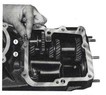
Fig. 178 - Fitting the reverse shaft and gear lock pin. 1. Lock pin. - 2. Reverse shaft and gear.
