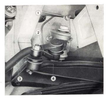
Fig. 284 - Idler arm and support. 1. Idler arm support. - 2. Idler arm. - 3. Track rod. - 4. Link rod.
