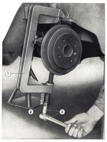
Fig. 264 - Installing coil spring compressor. 1. Tool A. 74052 for coil spring compression. - 2. Reference marks to be indexed. - 3. Ratchet wrench A. 89854.
