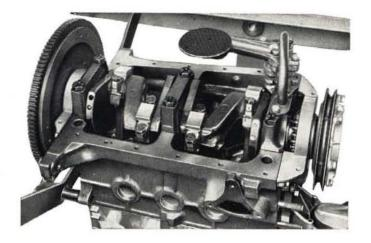
Fig. 125 - Oil pump in place in crankcase.
