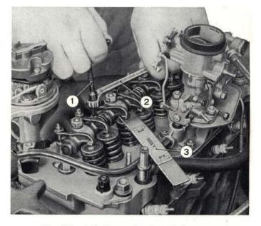
Fig. 119 - Adjusting valve tappet clearance. 1. «T» wrench A. 50006. - 2. Box wrench. - 3. Feeler A. 95111.
