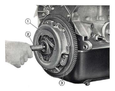
Fig. 162 - Using tool A. 70085 to align the driven plate. 1. Clutch assembly. - 2. Tool A. 70085. - 3. Flywheel.
