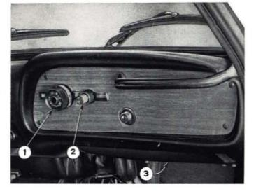
Fig. 505 - Radio receiver installed on car. 1. Tuning control knob. - 2. On-off and volume control knob. -3. Loudspeaker.
