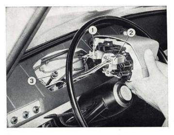
Fig. 367 - Removing instrument cluster for replacement of bulbs.
