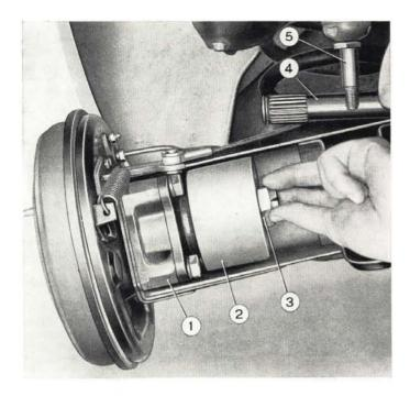
Fig. 258 - Loosening wheel shaft flexible joint mounting nut. 1. Wheel hub. - 2. Flexible joint. - 3. Joint mounting nut. - 4. Axle shaft. - 5. Shock absorber.
