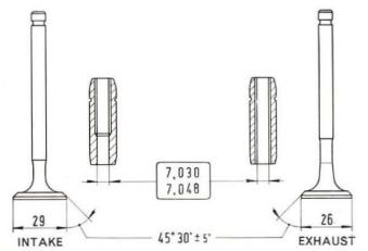
Fig. 425 - Critical dimensions (metric) of intake and exhaust valves and valve guides.
