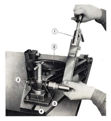
Fig. 528 - Installing lower control arm self-threading bushings. 1. Torque wrench. - 2. Coil spring housing. - 3. Fixture A. 74023. -4. Location marks to be indexed. - 5. Self-threading bushings.
