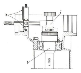
Fig. 194 - Diagram showing use of tools for figuring pinion shim thickness.
