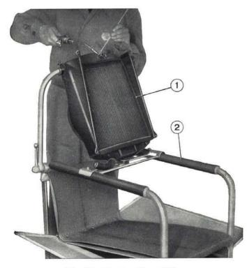
Fig. 134 - Tinning the radiator. 1. Radiator. - 2. Radiator service stand Arr. 22239.
