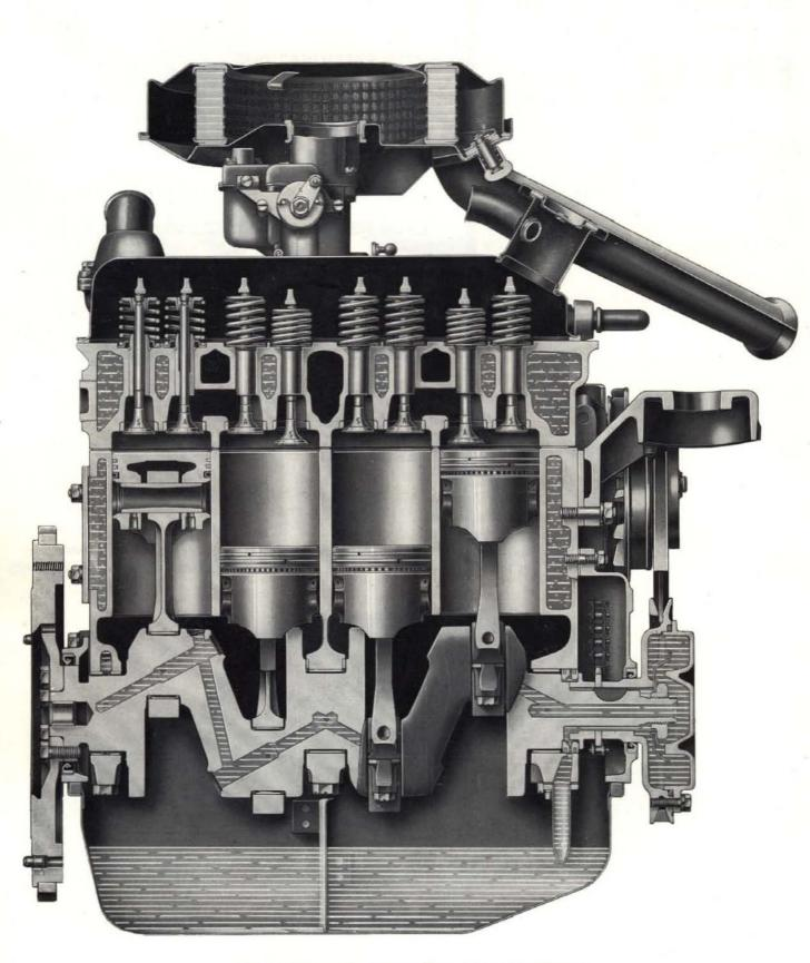
Fig. 6 - Side sectional view of engine across cylinders.
