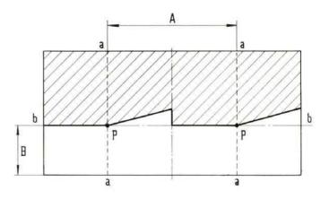
Fig. 495 - Headlight aiming diagram.  $A = 38^{7}/_{32}$ '' (971 mm) - B = C  $-\frac{25}{32}$ '' (20 mm) - C = Ground clearance of headlight center.
