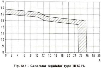
Fig. 547 - Generator regulator type IR 50 H. Volt/Amp regulating pattern at  $122^{\circ} \pm 5^{\circ}$  F ( $50^{\circ} \pm 3^{\circ}$  C). Generator speed: 5,000 r. p. m.
