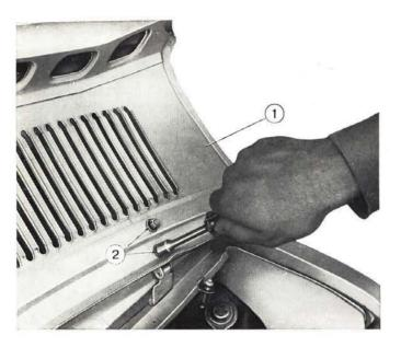
Fig. 403 - Repositioning engine compartment lid. 1. Lid. - 2. Lid hinge nuts.
