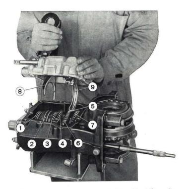
Fig. 172 - Removing side cover, complete with shifter rails and forks.
