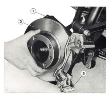
Fig. 454 - Removing brake disc. 1. Brake disc splash shield. - 2. Brake disc. - 3. Caliper bracket clamps.
