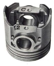
Fig. 42. Piston upside down, showing pin boss base.
