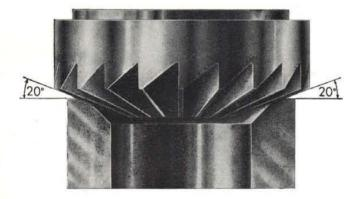
Fig. 96 - Narrowing valve seat at top with 20° cutter.
