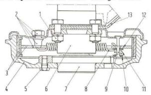
Fig. 291 - Sectional view of right side rear wheel. (Up to car with No. for spare 802091).
