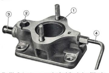
Fig. 154 - Carburetor spacer and recirculation device of blow-by gases and oil vapours. 1. Spacer. - 2. Breather valve. - 3. Recirculation pipe connector. -4. Fuel overflow drain pipe.
