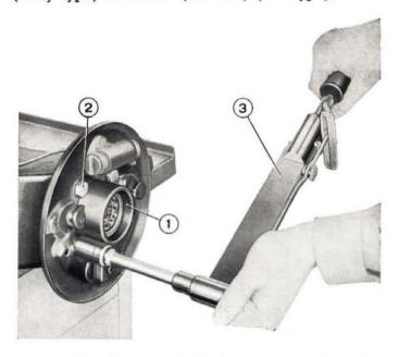
Fig. 253 - Securing rear wheel hub and brake backing plate to control arm.
