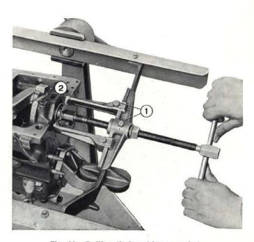
Fig. 14 - Pulling timing drive sprocket. 1. Puller A. 40005/2/5. - 2. Timing drive sprocket.
