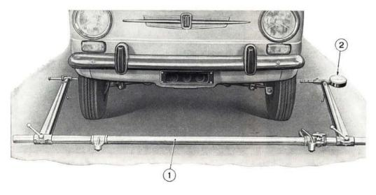
Fig. 286. Checking front wheel toe-in. 1. Gauge Ap. 5107. - 2. Toe-in gauge dial indicator.
