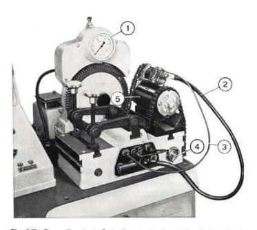
Fig. 345 - Operation test of starting motor, loaded and at no-load. 1. Drag torque dial indicator. - 2-3. Power cords. - 4. Starter switch. -5. Starting motor.
