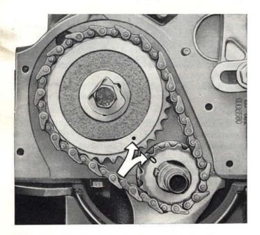
Fig. 117 - Timing marks on drive and driven sprockets. Chain stretchers should always be turned outward, as shown in figure.
