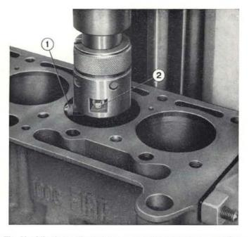
Fig. 31 - Aligning cylinder bore, preparatory to boring operation. 1. Centering plunger. - 2. Micrometer caliper shoulder setting screw.
