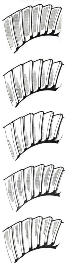
Fig. 201. Correct tooth contact.
