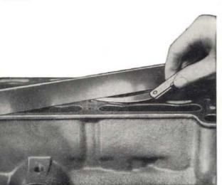
Fig. 34 - Checking lower face of crankcase.
