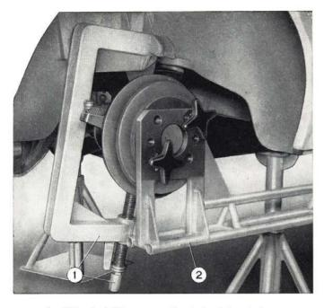
Fig. 266 - Installing rear wheel checking fixture.
