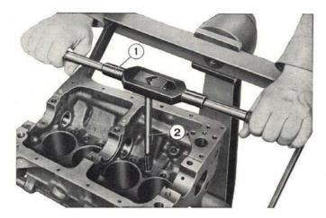
Fig. 116 - Reaming tappet seats in crankcase. 1. Reamer handle. - 2. Reamer A. 90318/1.
