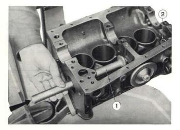
Fig. 114 - Fitting intermediate camshaft bushing. 1. Driver A. 60292. - 2. Flywheel end bushing.
