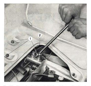
Fig. 300 - Removing brake and clutch pedal mounting board. 1. Screws, board to body. - 2. Brake and clutch pedal mounting board.
