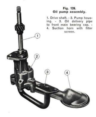
Clearance between drive gear shaft and seat must not be greater than .006" (0.15 mm); fit of new parts .0005" to .0020" (0.013 to 0.050 mm).
