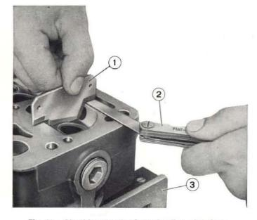
Fig. 89 - Checking depth of combustion chambers. 1. Gauge A. 95650. - 2, Feeler A. 95113. - 3. Head holding fixture A. 60041.
