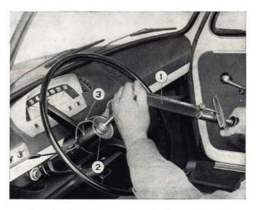
Fig. 272 - Tightening steering wheel mounting nut. 1. Torque wrench. - 2. Wheel mounting nut. - 3. Horn button wire.
