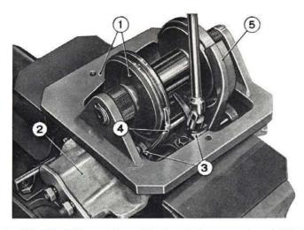
Fig. 182 - Installing and positioning first - second and third fourth shifter forks.
