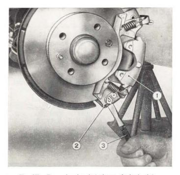
Fig. 449 - Removing bracket clamp pin lock plate. 1. Brake caliper. - 2. Lock plate. - 3. All-purpose plier.
