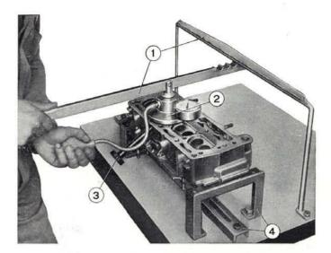
Fig. 102 - Valve seal test. 1. Tool A. 60041/2. - 2. Tester A. 60148. - 3. Tool A. 60018. - 4. Head holding tool A. 60041.
