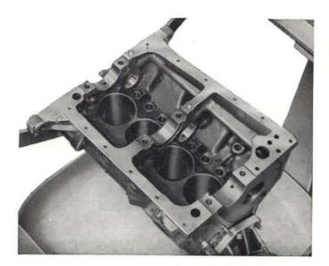
Fig. 36 - Bottom view of crankcase.
