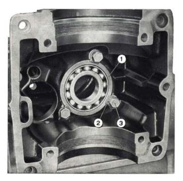
Fig. 177 - Drive pinion bearing in place in transmission case. 1. Ball bearing. - 2. Lock plate. - 3. Bearing screw.
