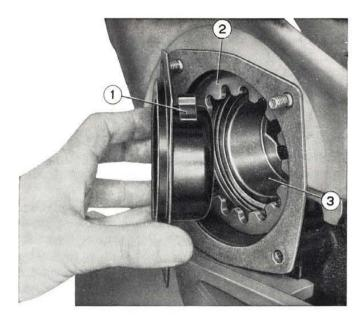
Fig. 190 - Fitting bearing adjuster stop plate. 1. Lug. - 2. Bearing adjuster. - 3. Roller bearing.
