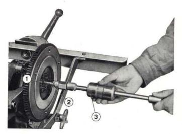
Fig. 82 - Pulling clutch shaft pilot bushing.
