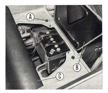
Fig. 314 - Arrangement of battery in car. A. Battery recess cover hold-down nut. - B. Battery recess cover. -C. Front compartment floor mat.
