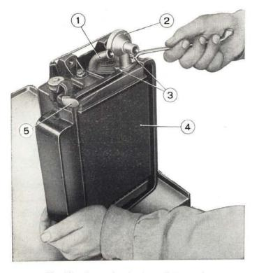
Fig. 310 - Removing heater radiator cock.
