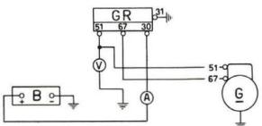
Fig. 330 - Wiring diagram for checking the reverse current of cutout.
