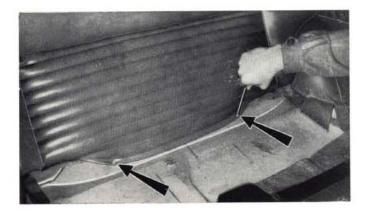
Fig. 475 - Removing rear seat back rest. Arrows point to back rest holding screws.
