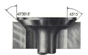
Fig. 95 - Inclination angles of valve seats in head and valve faces.
