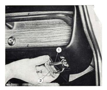
Fig. 500 - Disassembling interior lamps. 1. Inner lamp. - 2. Lamp lens.
