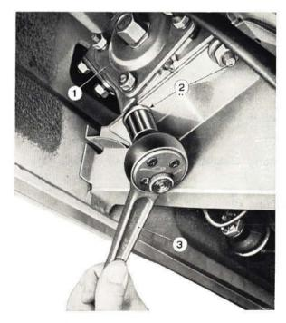
Fig. 534 - Removing steering gear.
