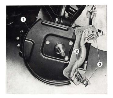
Fig. 456 - Detail showing caliper mounting bracket and disc splash shield.
