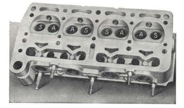
Fig. 99 - View of valve seats in head. A. Intake valve seat. - B. Exhaust valve seat.
