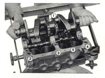
Fig. 15 - Lifting out crankshaft.
