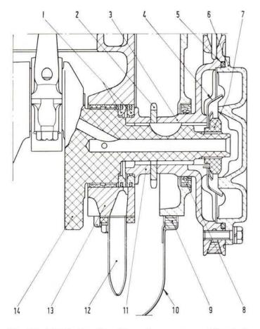
Fig. 127 - Detail of engine side section across centrifugal oil filter.
