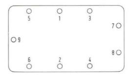
Fig. 589 - Tightening reference for cover retaining nuts.
