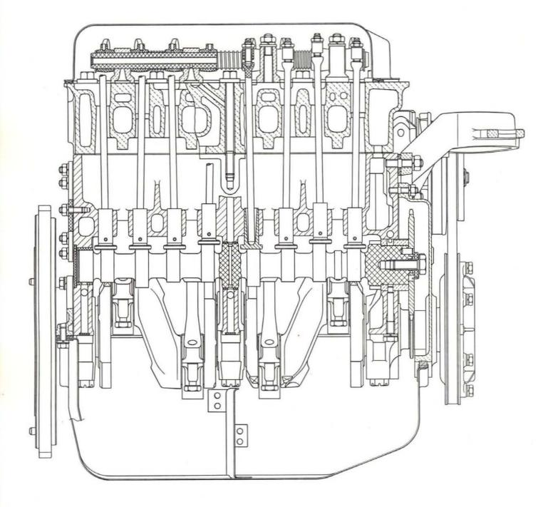
Fig. 83 - Side sectional view of engine across valve mechanism.
