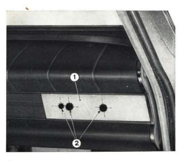
Fig. 465 - Fitting templet to drill radio receiver mounting holes. 1. Templet. - 2. Radio receiver mounting holes on instrument panel.
