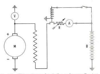
Fig. 343 - Wiring diagram for starting motor operation test. M. Starting motor. - V. Voltmeter, 15 V scale. - A. Ammeter, 1,000 A scale. - B. Battery, 50 A/h - 12 V. - R. Rheostat, 800 A capacity.
