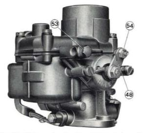
Fig. 148 - Solex carburetor viewed from choke end. 48. Choke control lever. - 53. Cable housing lock screw. - 54. Choke cable end clamp.
