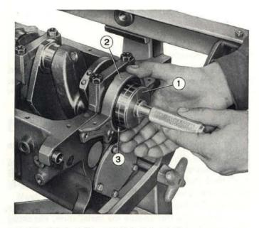
Fig. 20 - Installing crankshaft front oil seal cover. 1. Inserter A. 60281. - 2. Crankshaft front oil seal cover. - 3. Oil seal.
