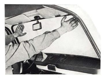
Fig. 405 - Removing windshield glass.
