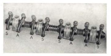
Fig. 108 - Rocker, shaft and support assembly. A. Intake valve rockers. - S. Exhaust valve rockers.
