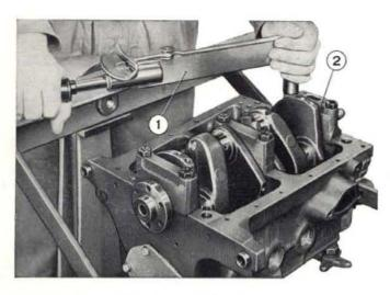
Fig. 79 - Tightening main bearing cap screws. 1. Torque wrench. - 2. Main bearing cap.
