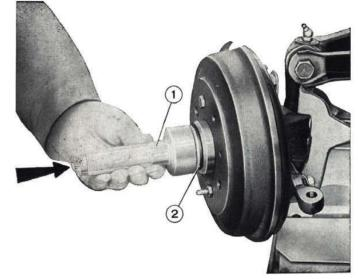
Fig. 230 - Installing wheel hub cap. 1. Driver A. 74088. - 2. Wheel hub cap.
