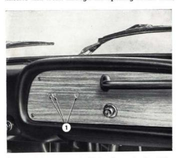
Fig. 503 - Instrument panel with location marks for drilling radio receiver mounting holes. 1. Location marks for drilling receiver mounting holes.
