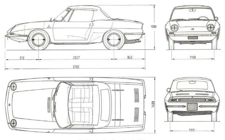
Fig. 482 - Leading dimensions (metric). Overall height applies to an unloaded car. Overall height for cars fitted with hard top is 47.44" (1,205 mm).
