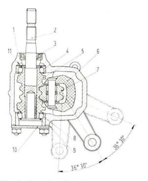
Fig. 535 - Sectional view of steering gear at worm-to-roller shaft meshing plane.
