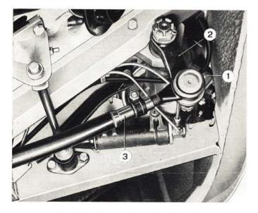
Fig. 533 - Detail of steering linkage. 1. Steering gear. - 2. Pitman arm. - 3. Drag link.
