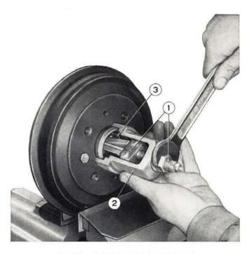
Fig. 222 - Pulling outer bearing cup. 1. Puller A. 47026/1. - 2. Puller bell. - 3. Bearing cup.
