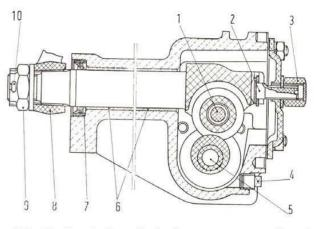
Fig. 536 - Sectional view of steering gear across roller shaft and pitman arm.
