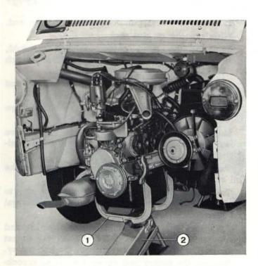
Fig. 8 - Removing engine. 1. Adapter A. 60534. - 2. Hydraulic jack.
