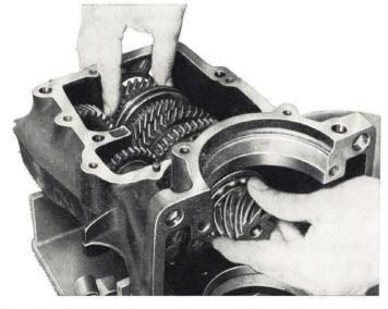
Fig. 179 - Installing the counter gear train and the countershaft-drive pinion.
