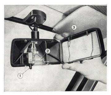
Fig. 368 - Removing map light bulb. 1. Toggle switch. - 2. Bulb. - 3. Mirror clip.
