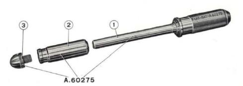
Fig. 52 - Tool A. 60275 for piston pin removal and installation. 1. Arbor, - 2. Guide pin, - 3. Stop screw. Use care to turn in the pin screw just a fraction to avoid that it may be overtightened as a result of piston pin expanding in touch with a hot connecting rod.
