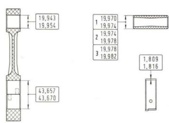
Fig. 58 - Critical dimensions (metric) of connecting rod, rod bearing insert and piston pin. (Early type)
