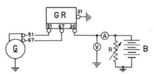
Fig. 331 - Wiring diagram for checking the current and voltage regulators.
