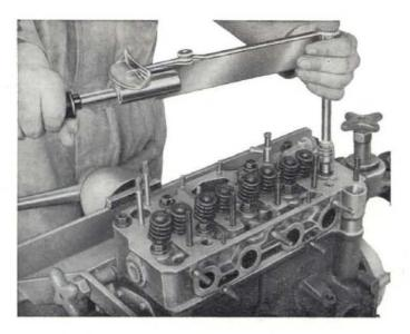
Fig. 86 - Tightening head screws by means of torque wrench.
