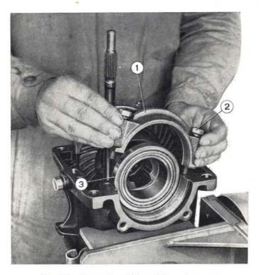
Fig. 188 - Removing differential carrier caps. 1. Cap. - 2. Cap screw. - 3. Roller bearing.
