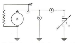
Fig. 320 - Wiring diagram for plotting the ampere-revolution output curve at a steady 12 V voltage (68° F - 20° C).
