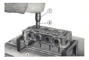
Fig. 87 - Decoking and cleaning combustion chambers. 1. Drill. - 2. Wire brush. - 3. Head holding fixture A. 60041.
