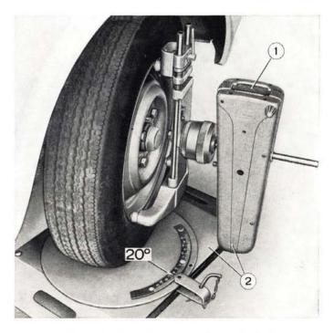
Fig. 237 - Checking caster (second step). 1. « Caster » angle. - 2. Fixture Ap. 5106. The wheel should be steered 20° in.
