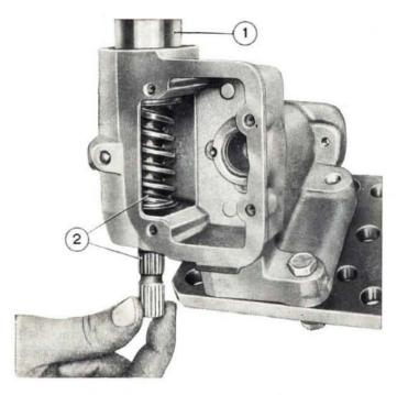
Fig. 277 - Adjusting worm bearings. 1. Wrench A. 57003 for bearing adjuster nut. - 2. Worm.
