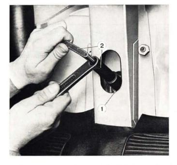
Fig. 524 - Disconnecting shock absorber at top end. 1. Shock absorber. - 2. Wrench A. 57035.
