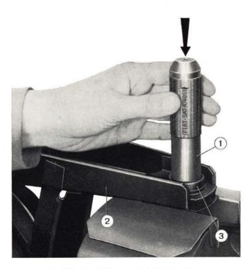
Fig. 248 - Installing control arm bushing. 1. Driver A. 74053. - 2. Control arm. - 3. Resilient bushing.
