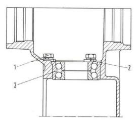
Fig. 193 - Placing drive pinion rear bearing into transmissiondifferential case.
