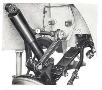
Fig. 233 - Fitting camber and caster adjusting shims. 1. Shims at rear screw. - 2. Shims at front screw.
