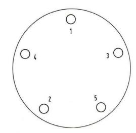
Fig. 581 - Tightening diagram for pump body retaining screws.
