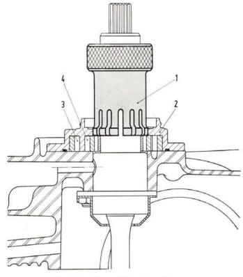
Fig. 593 - Centralising the oil pump.
