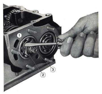
Fig. 173 - Prying out countershaft-drive pinion nut lock ring. 1. Lock ring. - 2. Nut. - 3. Speedo drive driving gear.
