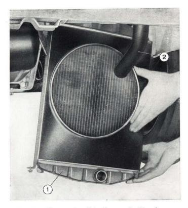
Fig. 133 - Lifting out radiator from underside of car. 1. Radiator. - 2. Coolant inlet hose.
