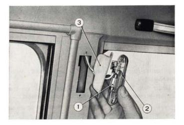
Fig. 554 - Removing dome light. 1. Cylindrical bulb. - 2. Lens. - 3. Lamp shield.
