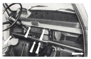
Fig. 305 - Removing utility shelf. Arrows point to shelf mounting screws.
