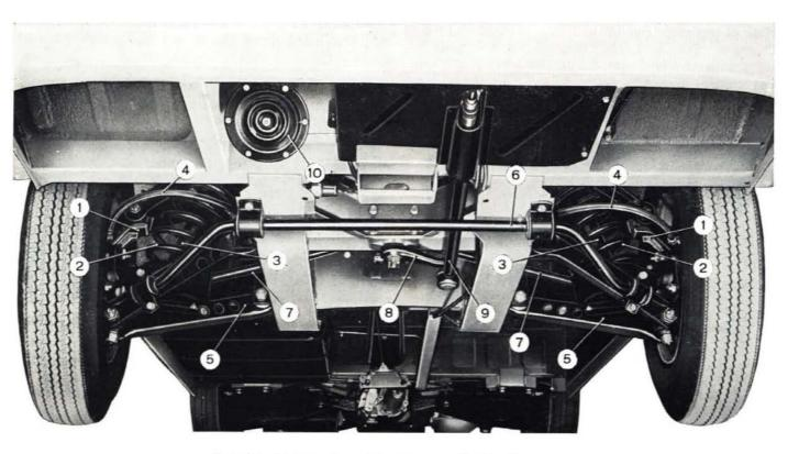
Fig. 523 - Bottom view of front suspension in place on car. 1. Kingpins. - 2. Coil springs. - 3. Shock absorbers. - 4. Front brake hoses. - 5. Lower control arms. - 6. Front sway bar. - 7. Tie rods. -8. Idler arm. - 9. Drag link. - 10. Horn.
