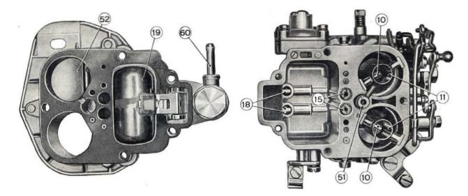
Fig. 436 - Inner view of carburetor body and cover.
