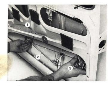
Fig. 391 - Taking down door lock and control. 1. Door remote control. - 2. Control link. - 3. Lock assembly.
