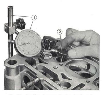
Fig. 100 - Checking clearance of valve stem in guide. 1. Magnetic dial indicator. - 2. Valve part way out.
