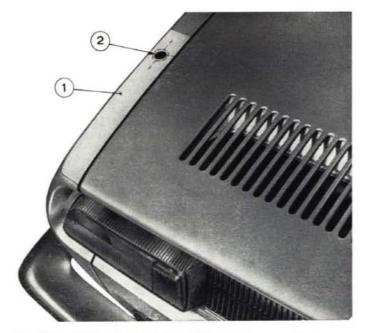
Fig. 502 - Fitting templet for drilling antenna rod passage opening.
