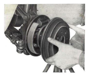
Fig. 292 - Removing brake drum.
