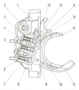
Fig. 176 - Cross sectional view of transmission side cover assembly.
