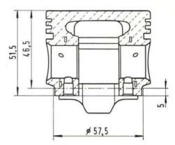
Fig. 46 - Milling diagram of piston to equalize the set weight.  $\varnothing$  57,5 = 2  $\frac{1}{4''}$  diam. - 5 =  $\frac{3}{16''}$  - 51,5 = 2  $\frac{1}{32''}$  - 46,5 = 1  $\frac{25}{32''}$ .
