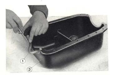
Fig. 23 - Fitting oil sump gasket. 1. Gasket. - 2. Oil sump.
