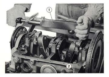
Fig. 63 - Securing connecting rod bearing caps. 1. Torque wrench. - 2. Con rod bearing cap.
