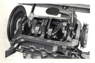
Fig. 12 - Crankcase without oil sump.
