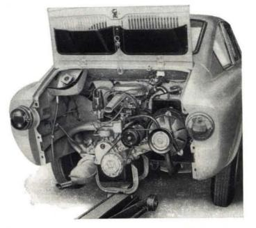
Fig. 416 - Using hydraulic jack and adapter A. 60534 to remove engine.
