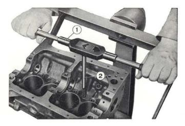
Fig. 38 - Reaming tappet seats on crankcase. 1. Reamer handle. - 2. Tappet seat reamer A. 90318/1.
