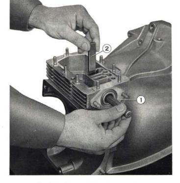
Fig. 584 - Reassembling plunger valve.
