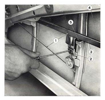
Fig. 395 - Adjusting drop glass travel. 1. Window regulator cable. - 2. Cable stop plate. - 3. Glass bottom channel. - 4. Glass pane. - 5. Buffer.
