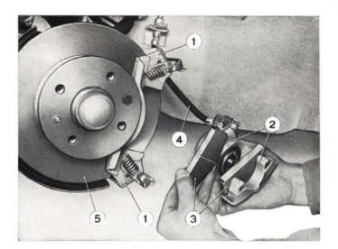
Fig. 453 - Replacing lining pads. 1. Caliper bracket clamps. - 2. Brake caliper. - 8. Lining pads. -4. Brake fluid hose. - 5. Brake disc.
