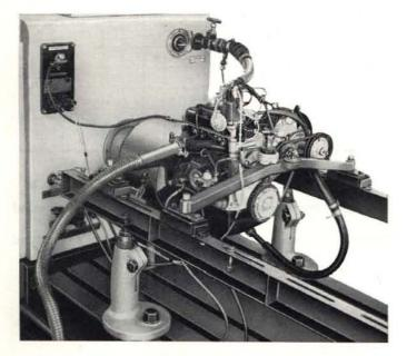
Fig. 120 - Detail of engine on test bench.
