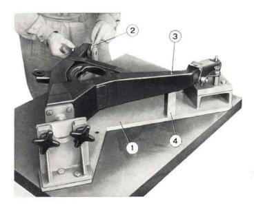
Fig. 250 - Adjusting rear control arm. 1. Fixture A. 74142. - 2. Shims. - 3. Control arm. - 4. Fixture dowel.
