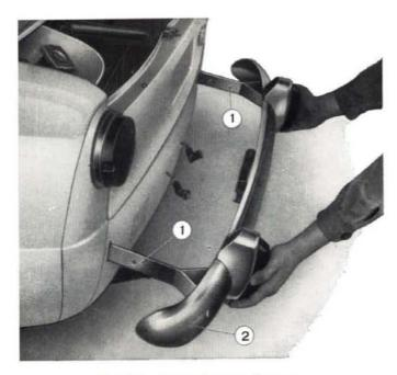
Fig. 408 - Removing rear bumper. 1. Bumper brackets. - 2. Bumper.
