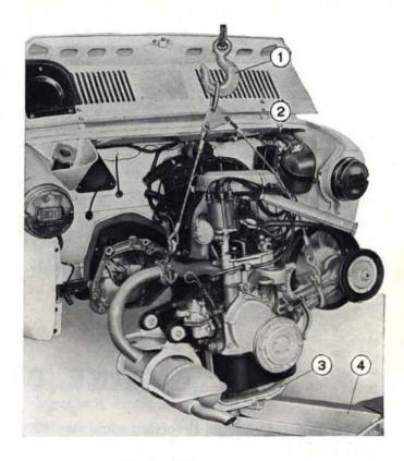
Fig. 9 - Lifting out engine.
