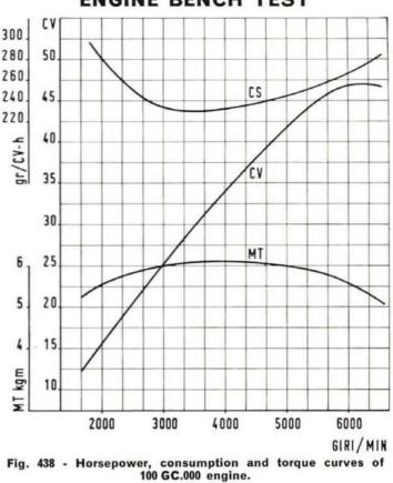
Corrected horsepower curve shown in figure refers to a rebuilt and run-in engine with fan, air cleaner and muffler.
