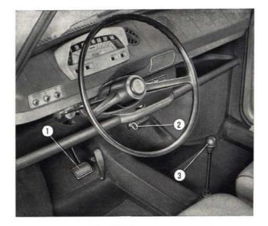
Fig. 572 - Car controls. 1. Brake pedal. - 2. Accelerator hand control. - 3. Gear selector lever with integral knob switch.
