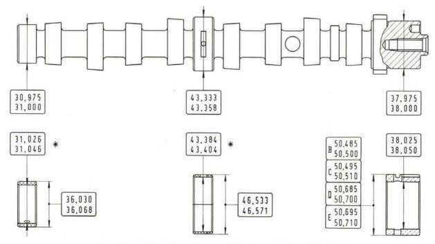
Fig. 112 - Critical dimensions (metric) of camshaft and bushings.
