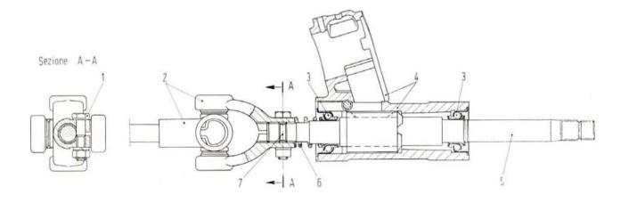
Fig. 487 - Section view of the steering column and mounting bracket.
