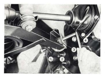
Fig. 256 - Securing rear control arm to body shell. 1. Control arm rear lock pin. - 2. Control arm. - 3. Shims. - 4. Tool A. 74143.
