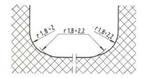
Fig. 68 - Fillet radii for intermediate main bearing journal shoulder. r 1,8÷2 = .071'' to .079'' - r 1,8÷2,2 = .071'' to .087''
