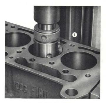
Fig. 33 - Reboring cylinders. 1. Cutting tool.
