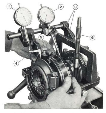
Fig. 199 - Checking ring gear-to-pinion backlash.
