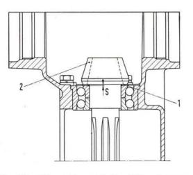
Fig. 195 - Drive pinion and shim fitting diagram.1. Drive pinion shim. - 2. Drive pinion. - S. Shim thickness.
