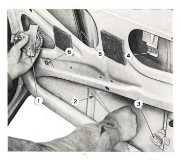
Fig. 392 - Taking down window regulator assembly.
