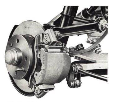
Fig. 448 - Left side front wheel disc brake assembly.
