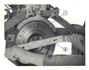
Fig. 24 - Affixing sector scale. 1. Sector scale A. 95694. - 2. Flywheel crank A. 60186.
