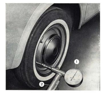
Fig. 285 - Detail showing the arrangement of front wheel toe-in gauge.
