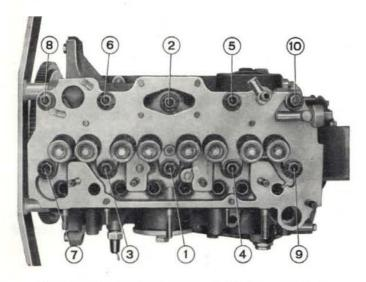
Fig. 84 - Cylinder head screws tightening sequence. 1st pass: torque to some 21.7 ft.lbs (3 kgm). - 2nd pass: torque to 28.9 to 36.2 ft.lbs (4 to 5 kgm).
