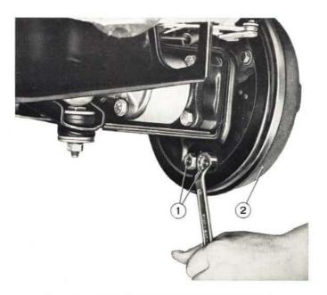
Fig. 542 - Loosening lower anchor campin nuts. 1. Campin nuts. - 2. Brake drum.
