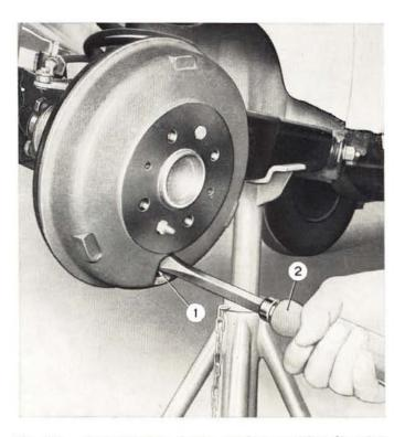
Fig. 543 - Repositioning lower anchor campins for shoe clearance adjustment. 1. Anchor campins. - 2. Screwdriver for campin lock.
