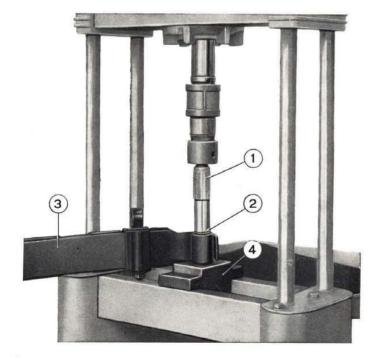
Fig. 216 - Press fitting resilient bushing into semi-elliptic spring end eye.
