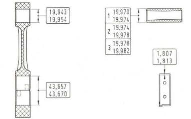
Fig. 60 - Critical dimensions (metric) of connecting rod, rod bearing insert and piston pin. (Late type)
