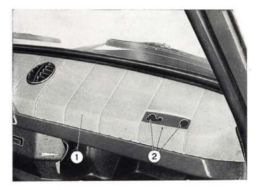
Fig. 380 - Fitting the templet for cutting out the instrument panel lining and fashioning the panel holes, preparatory to the radio set installation.
