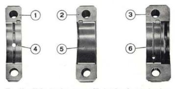
Fig. 74 - Main bearing caps with bearing inserts in place. 1. Front cap. - 2. Intermediate cap. - 3. Rear cap. - 4, 5, 6. Bearing inserts.
