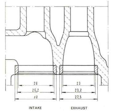
Fig. 428 - Diameters of intake and exhaust valve seats in head. 26 = 1.024'' - 26,2 = 1.031'' - 30 = 1.181'' - 23 = .905'' - 23,2 = .913'' -27,5 = 1.083''.
