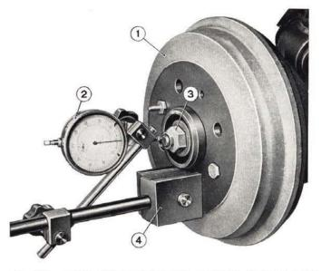
Fig. 239 - Using dial indicator with magnetic base to check wheel hub end play.
