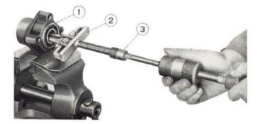
Fig. 246 - Pulling rear wheel ball bearing. 1. Rear wheel hub. - 2. Tool A. 40005/4. - 3. Ram puller A. 40006/1.
