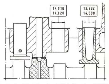
Fig. 37 - Critical dimensions (metric) of tappets and tappet seats on crankcase.
