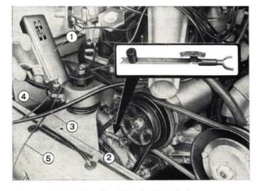
Fig. 357 - Checking ignition timing. 1. Strobe lamp. - 2. Plate Ap. 5030/9. - 3. Lamp power cord. - 4. Spark plug cable. - 5. Ground cable.
