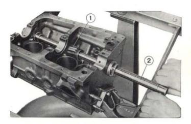
Fig. 115 - Reaming intermediate camshaft bushing. 1. Reamer. - 2. Tool A. 90326.
