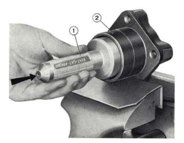
Fig. 251 - Installing roller bearing cup. 1. Driver A. 74088. - 2. Rear wheel hub.
