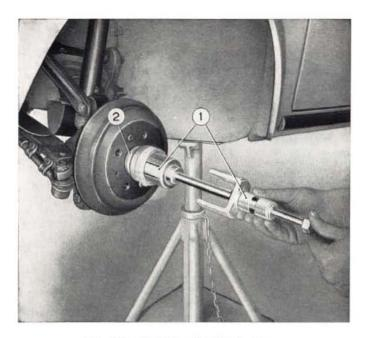
Fig. 212 - Pulling wheel hub cap. 1. Ram puller A. 47014. - 2. Wheel hub cap.
