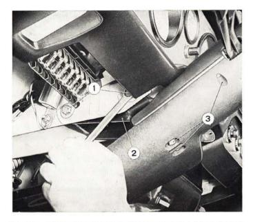
Fig. 488 - Removing steering column mounting bracket from instrument panel.
