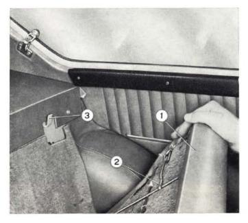
Fig. 476 - Removing rear seat back rest. 1. Back rest. - 2. Back rest hooking strut. - 3. Back rest clamp.
