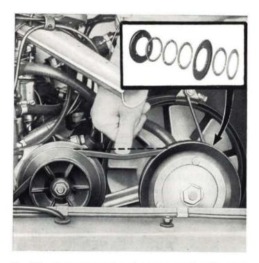
Fig. 137 - Checking tension of generator and water pump drive belts. The inset shows the correct position of shims.
