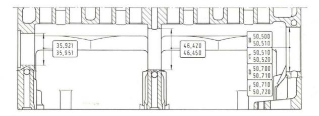
Fig. 35 - Critical dimensions (metric) of camshaft bushing seats. Timing end bushing seating bore is graded into four classes.
