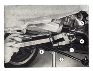
Fig. 274 - Removing steering rods. 1. Tool A. 47035. - 2. Link rod. - 3. Pitman arm. - 4. Rod end ball stud. - 5. Track rod.
