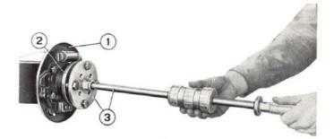
Fig. 245 - Pulling rear wheel hub.
