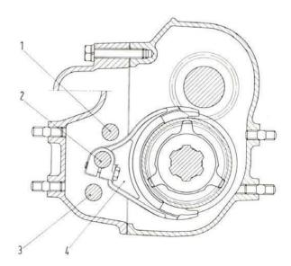
Fig. 181 - End sectional view of transmission across shifter rails.
