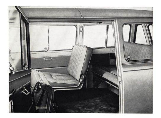
Fig. 558 - Interior view of 850 Family with one intermediate seat section in collapsed position.
