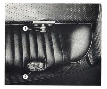
Fig. 511 - Detail showing seat squab adjusting device. 1. Squab adjuster push rod and nut. - 2. Push rod backing plate.
