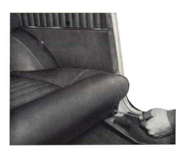
Fig. 474 - Removing rear seat cushion.
