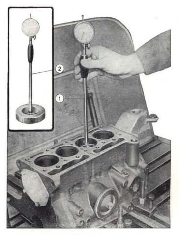
Fig. 28 - Using dial indicator to measure cylinder bores. 1. Dial indicator. - 2. Zero setting indicator with master gauge A. 95647\*
