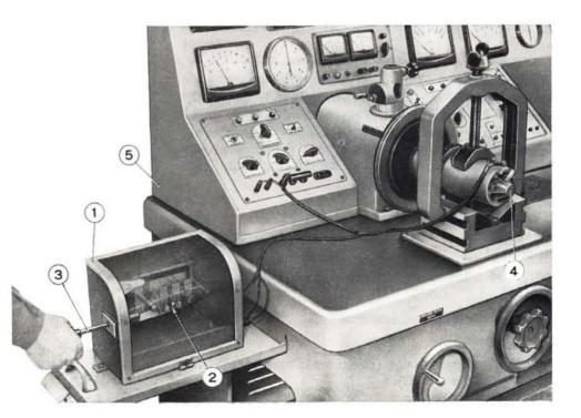
Fig. 336. Adjusting generator regulator in thermostat oven Ap. 5014 for temperature stabilization.
