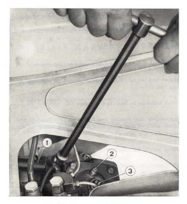
Fig. 273 - Removing steering gear. 1. Steering shaft. - 2. Oil filler plug. - 3. Sector adjusting screw.
