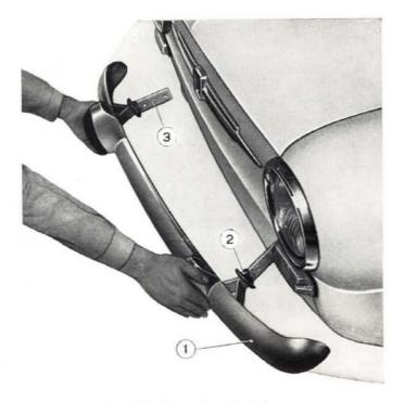
Fig. 407 - Removing front bumper. 1. Bumper. - 2. Bracket gasket. - 3. Bumper bracket.
