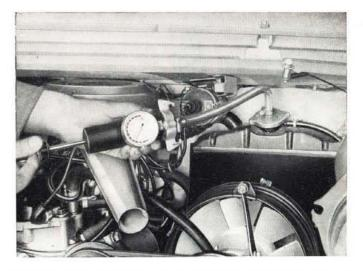
Fig. 129 - Checking leakage of cooling system by means of tester Ap. 5066.
