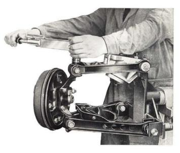
Fig. 531 - Tightening kingpin screw to upper control arm with unit on fixture A. 22229.
