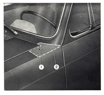
Fig. 379 - Fitting the templet for drilling the antenna rod passage opening.
