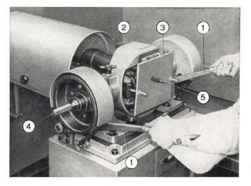
Fig. 200 - Bench testing differential unit.
