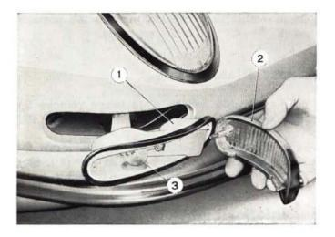
Fig. 496 - Disassembling front corner parking and direction signal lamp.
