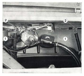
Fig. 135 - Detail showing radiator mounting. 1. Supporting springs. - 2. Spring hangers.
