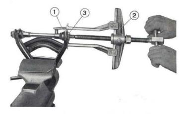
Fig. 213 - Pulling upper control arm bushings. 1. Tool A. 74116. - 2. All-purpose puller A. 40005. - 3. Resilient bushing.
