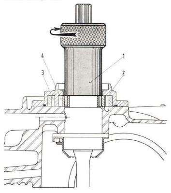
Fig. 594 - Checking pump gear rotation.
