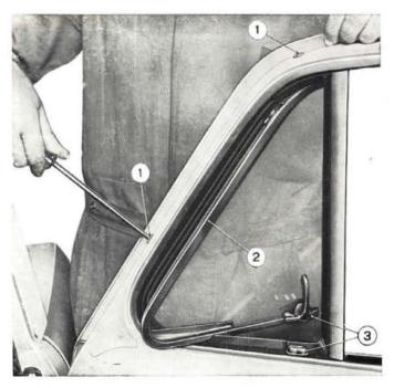
Fig. 389 - Removing ventilator window.
