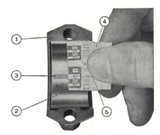
Fig. 64 - Comparing the width of the flattened « Plastigage » with the envelope graduation scale to check connecting rod bearing insert-to-journal clearance.
