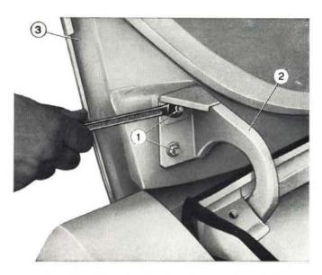
Fig. 401 - Repositioning front compartment lid. 1. Lid hinge stud nuts. - 2. Lid hinge. - 3. Front compartment lid.
