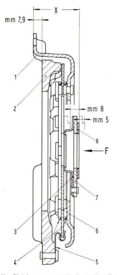
Fig. 161 - Clutch cover assembly inspecting diagram.
