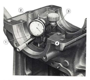
Fig. 196 - Step for figuring the thickness of drive pinion shim.
