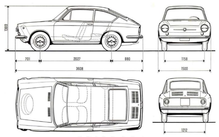
Fig. 418 - Leading dimensions (in mm). Overall height applies to an unloaded vehicle.
