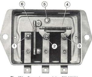
Fig. 334 - Generator regulator GN 2/12/16. Bottom view.
