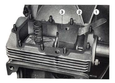
Fig. 588 - Assembling the valve cover.
