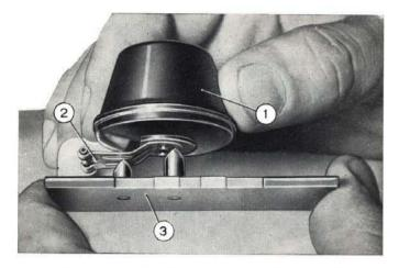
Fig. 150 - Solex carburetor: checking float arm. 1. Float. - 2. Float arm. - 3. Gauge A. 95126.
