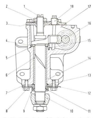
Fig. 278 - Sectional view of the steering gear at sector. 1. Sector adjusting screw. - 2. Lock nut. - 3. Plain washer. - 4. Thrust washer. - 5. Shims. - 6. Eccentric bushing. - 7. Bushing shim. -8. Shim screws. - 9. Seal cover. - 10. Pitman arm. - 11. Oil seal. -12. Shim packing. - 13. Upper oil seal. - 14. Steering housing. -15. Washer (4) location dowel. - 16. Worm. - 17. Cover. - 18. Oil filler plug.
