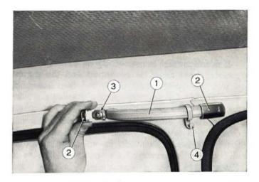
Fig. 411 - Removing strap hanger. 1. Strap hanger. - 2. Screw cap. - 3. Hanger mounting screw. -4. Dress hook.
