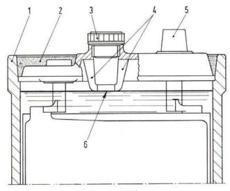
Fig. 313 - Side sectional view of battery at filler neck with electrolyte level sight.
