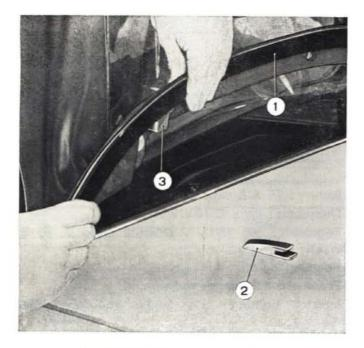
Fig. 516 - Hooking up canvas at rear. 1. Top rear cross rail. - 2. Cross rail hook. - 3. Hook seat.
