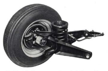
Fig. 257 - Left side rear suspension and wheel assembly.
