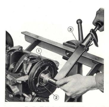
Fig. 21 - Tightening hub-pulley nut. 1. Hub-pulley - 2. Baffle ring. - 3. Torque wrench.
