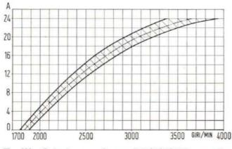
Fig. 321 - Output curve of warm D 90/12/16/3 CS generator. Steady 12 V Voltage. GIRI/MIN = R. P. M.
