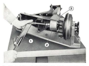
Fig. 254 - Installing wheel shaft flexible joint on work bench. 1. Torque wrench. - 2. Flexible joint. - 3. Rear control arm.
