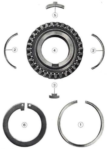
Fig. 167 - Third speed gear and synchronizer components. 1. Synchromesh ring. - 2. Synchronizer spreader springs. - 3. Stop plate. - 4. Third speed gear with toothed crown for synchromesh. -5. Thrust plate. - 6. Snap ring.
