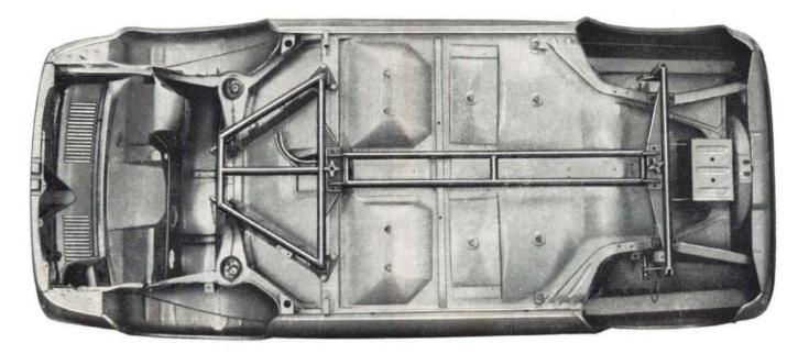
Fig. 412 - Checking underbody with gauge A. 74141.
