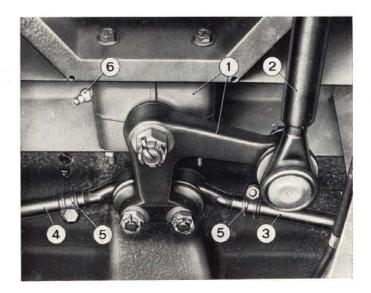
Fig. 537 - Detail of idler arm and support.
