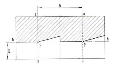
Fig. 461 - Headlight aiming diagram.  $A = 44^{23}/_{32}$  (1,136 mm). - B = C  $-\frac{25}/_{32}$  (20 mm). - C = Ground clearance of headlight center.
