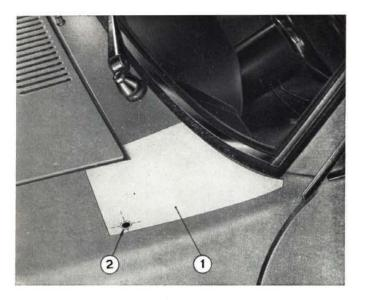
Fig. 464 - Fitting templet to drill antenna rod passage opening.
