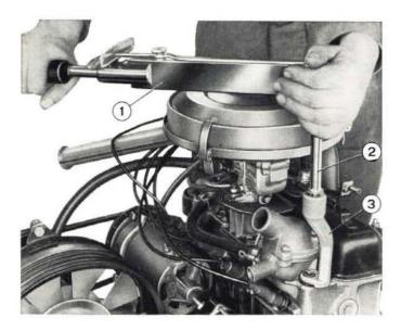
Fig. 136 - Fitting thermostat to engine. 1. Torque wrench. - 2. Torque wrench extension. - 3. Adapter socket A. 50111.
