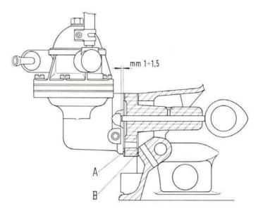
Fig. 140 - Setting fuel pump push rod projection. A. Gasket .0106'' to .0130'' (0.27 to 0.33 mm) thick. - B. Gasket .0276'' to .0315'' (0.7 to 0.8 mm) thick. Figure  $1\div1,5$  mm = .0394'' to .0591'' is jutting specified for the push rod.
