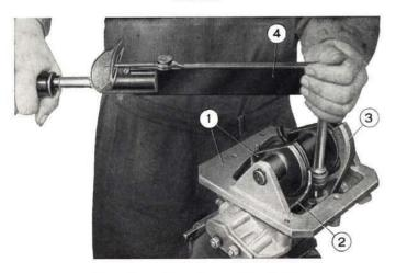
Fig. 184 - Tightening shifter forks. 1. Tool A. 70099. - 2. Third and fourth shifter fork. - 3. First and second shifter fork. - 4. Torque wrench.
