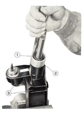
Fig. 491 - Removing steering column bracket bearing snap rings.
