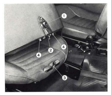
Fig. 477 - Front seat back rest catch device. 1. Catch release button. - 2. Catch hook. - 3. Catch striker. - 4. Catch mounting screws.
