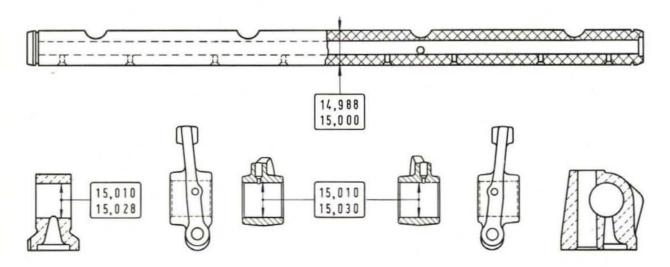
Fig. 110 - Critical dimensions (metric) of rockers, shaft and supports.
