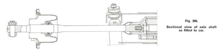
Observe the slip sleeve snap ring to make sure that it fits snugly in its groove in axle shaft.
