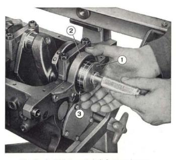
Fig. 81 - Installing crankshaft front seal cover. 1. Inserter A. 60281. - 2. Crankshaft front seal cover. - 3. Oil seal.
