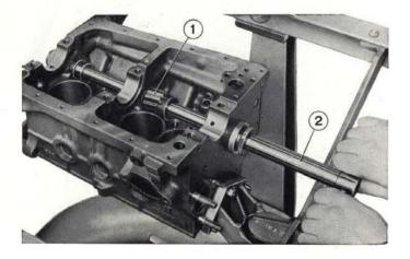
Fig. 17 - Reaming intermediate camshaft bushing. 1. Reamer for intermediate bushing. - 2. Reamer chuck A. 90326.
