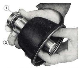
Fig. 191 - Fitting differential cage oil boot bushing. 1. Boot bushing. - 2. Tool A. 70103.
