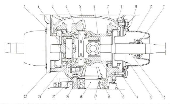
Fig. 186 - Side sectional view of transmission-differential across differential cage, final gear set and axle shaft slip joints.
