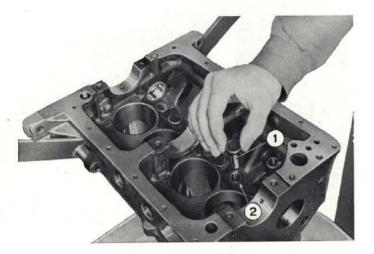
Fig. 16 - Fitting tappets. 1. Tappet. - 2. Tappet seat in crankcase.
