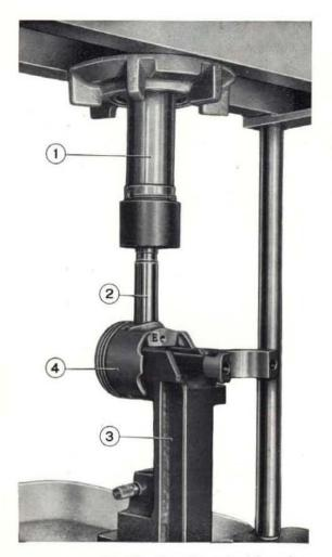
Fig. 49 - Pressing out piston pin. 1. Press arbor. - 2. Guide pin of tool A. 60285. - 3. Holder of tool A. 95605. - 4. Connecting rod-piston-pin assembly.
