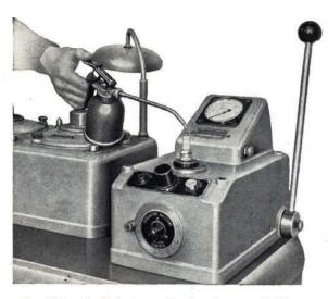
Fig. 355 - Testing a spark plug for gas tightness.
