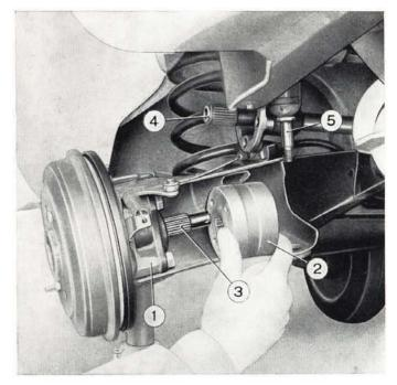
Fig. 260 - Removing flexible joint. 1. Wheel hub. - 2. Flexible joint. - 3. Wheel shaft. - 4. Axle shaft. -5. Shock absorber.
