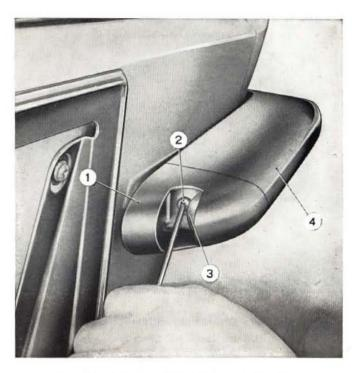
Fig. 498 - Disassembling license plate lamp. 1. Lamp shell. - 2. Screw, lamp shell-to-bumper. - 3. License plate light bulb. - 4. Bumper.
