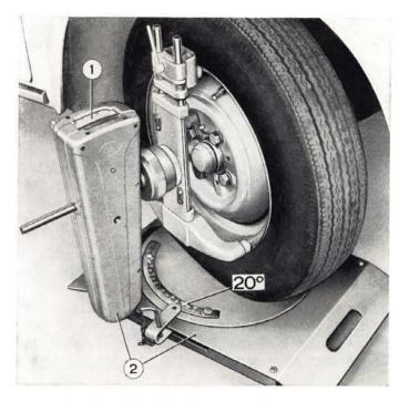
Fig. 236 - Checking caster (first step). 1. « Caster » scale, set at zero. - 2. Fixture Ap. 5106. The wheel should be steered 20° out.
