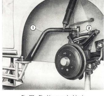
Fig. 267 - Checking rear wheel toe-in. 1. Clamp Ap. 5110/6 to be fitted to gauge Ap. 5110/1. - 2. Plunger for toe-in check.
