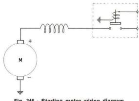
Fig. 346 - Starting motor wiring diagram.
