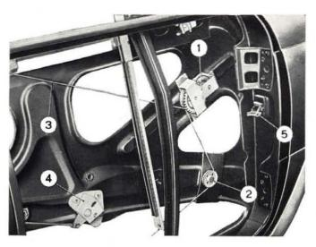
Fig. 397 - Door and window controls. 1. Regulator. - 2. Regulator cable sheave. - 3. Regulator cable. -4. Remote control. - 5. Door check strap.
