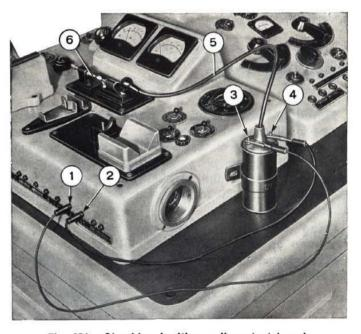
Fig. 354 - Checking ignition coil on test bench. 1. Breaker. - 2. 12 Volt power socket. - 3. Low tension cable ter-
