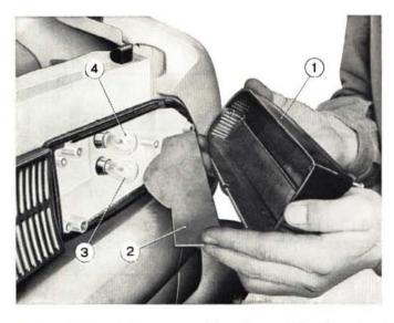
Fig. 497 - Disassembling rear parking stop and direction signal lamp.
