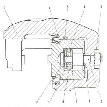
Fig. 451 - Side sectional view of the disc brake caliper.
