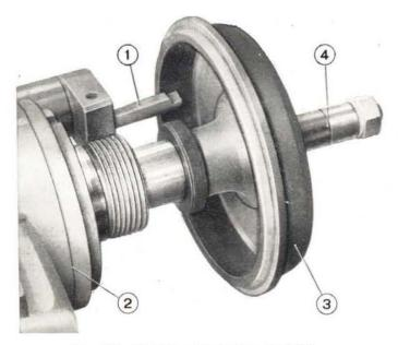
Fig. 295 - Turning brake drum on lathe. 1. Cutter. - 2. Lathe M. 1004. - 3. Brake drum. - 4. Drum holding spacer
