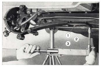
Fig. 231 - Securing semi-elliptic spring to body shell. 1. Semi-elliptic spring mounting screw. - 2. Torque wrench extension. - 3. Torque wrench.
