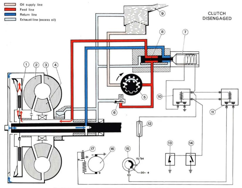
Fig. 568 Operating diagram of Idroconvert transmission with clutch disengaged.
