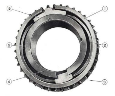
Fig. 166 - Third speed gear synchronizer in place in gear. 1. Synchromesh ring. - 2. Ring spreader springs. - 3. Stop plate. -4. Third speed gear. - 5. Thrust plate.
