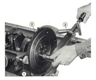
Fig. 72 - Tightening flywheel mounting nuts. 1. Tool A. 60282. - 2. Flywheel mounting nuts. - 3. Torque wrench.
