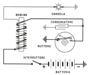
Fig. 348 - Ignition system wiring djagram.
