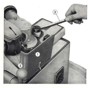
Fig. 101 - Grinding valve face. 1. Valve. - 2. Stone. - 3. Movable support actuating lever.
