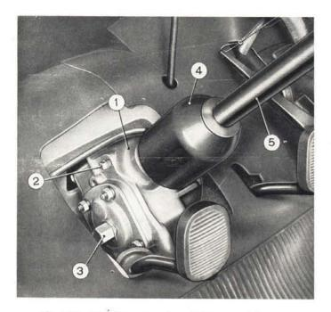
Fig. 532 - Steering gear viewed from car interior. 1. Steering gear. - 2. Oil filler plug. - 3. Roller shaft adjusting screw nut. - 4. Steering column flexible joint boot. - 5. Steering column.
