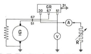
Fig. 322 - Wiring diagram for the generator heating test. G. Generator. - GR. Regulator. - V. Voltmeter, 15 V scale. - A. Ammeter, 20 A scale. - R. Carbon plate type rheostat, 100 A capacity, 0.2 to 20  $\Omega$  variable resistance.
