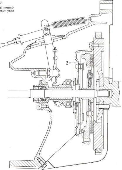
Fig. 160. Side sectional view of clutch and throwout mechanism.
