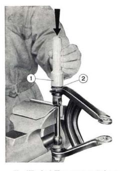
Fig. 227 - Installing upper control arm bushings. 1. Driver A. 74044. - 2. Resilient bushing.
