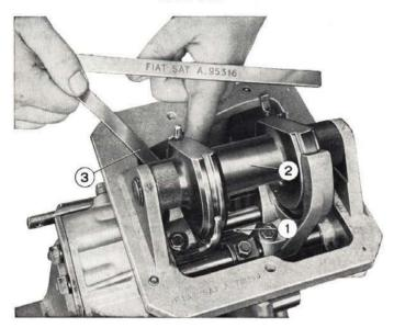
Fig. 183 - Checking clearance between first and second shifter rail dog and third and fourth shifter rail.
