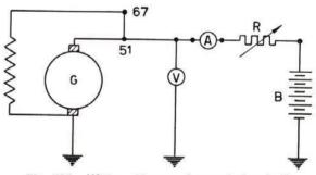
Fig. 319 - Wiring diagram for motoring test.
