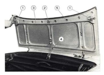
Fig. 519 - Removing folded top recess lid latch link. 1. Lid latches. - 2. Cam pin for latch control. - 3. Top recess lid. -4. Lid spring strut. - 5. Lid latch link.
