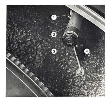
Fig. 381 - Detail of antenna mounting. 1. Cable, antenna to radio set. - 2. Antenna. - 3. Antenna mounting bracket. - 4. Bracket screw.
