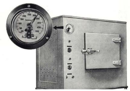
Fig. 51 - Electric oven for heating connecting rods. The thermostat, set at 608° F (320° C), is also shown in an enlarged view.
