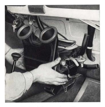
Fig. 308 - Withdrawing air conditioner.
