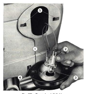
Fig. 365 - Removing tail light. 1. Stop light bulb holder. - 2. Direction signal light bulb holder. -3. Direction signal light bulb. - 4. Lamp complete with gasket. -5. Lamp locking plates to body.
