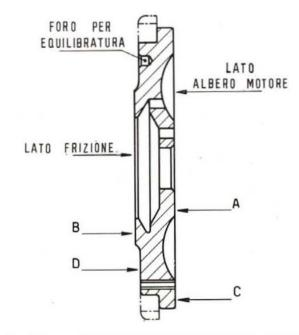
Fig. 71 - Diagram for checking flywheel mating faces to driven plate and crankshaft mounting flange.
