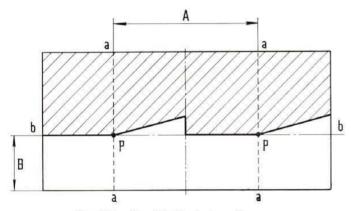
Fig. 362 - Headlight aiming diagram.
