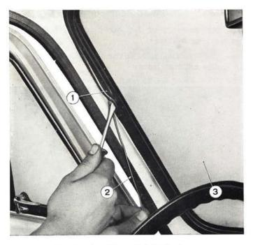
Fig. 404 - Installing windshield glass. 1. Rubber weatherstrip. - 2. Weatherstrip draw cord. - 3. Windshield glass.
