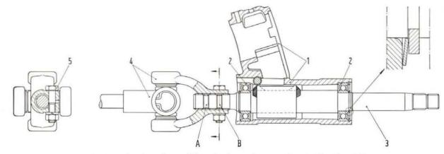
Fig. 485 - Section view of the steering column and mounting bracket.
