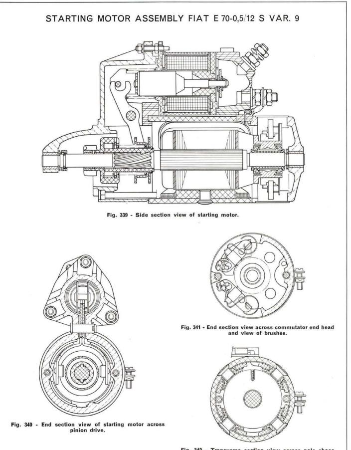
Fig. 342 - Transverse section view across pole shoes and field winding.
