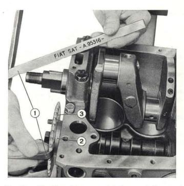
Fig. 18 - Checking driven sprocket - to - camshaft spacer clearance. 1. Feeler gauge A. 95316. - 2. Camshaft spacer. - 3. Driven sprocket.
