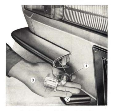
Fig. 499 - License plate lamp components. 1. License plate lamp bulb holder. - 2. License plate lamp bulb. -3. Lamp lens.
