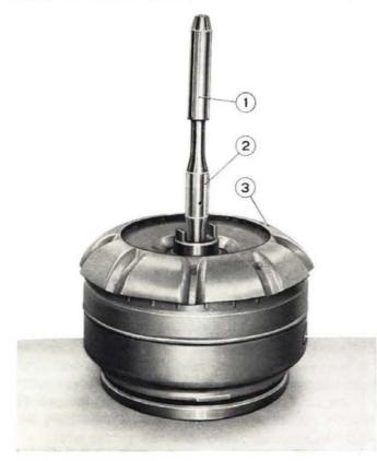
Fig. 590 - Torque converter assembly. 1. Service tool A. 70147 for protection of seals. - 2. Torque converter output shaft. - 3. Torque converter.
