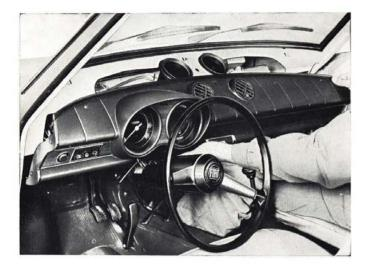
Fig. 468 - Removing instrument panel lining and cluster assembly.
