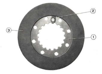
Fig. 567 - Clutch driven plate. 1. Driven plate. - 2. Partialising valve. - 3. Friction lining.
