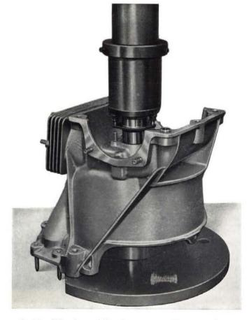
Fig. 576 - Assembling torque converter support.
