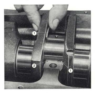
Fig. 78 - Fitting thrust ring halves. 1. Thrust ring halves. - 2. Intermediate main bearing insert.
