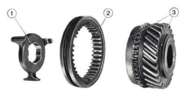
Fig. 165 - Transmission synchromesh gears. 1. Slip sleeve hub. - 2. Third and fourth slip sleeve. - 3. Third speed gear with synchronizer.
