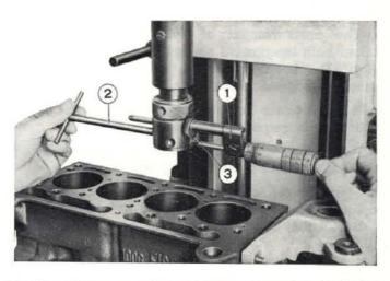
Fig. 32 - Measuring cutter projection, preparatory to boring operation. 1. Cutter setting device rod. - 2. Cutter setting wrench. - 3. Cutter-
