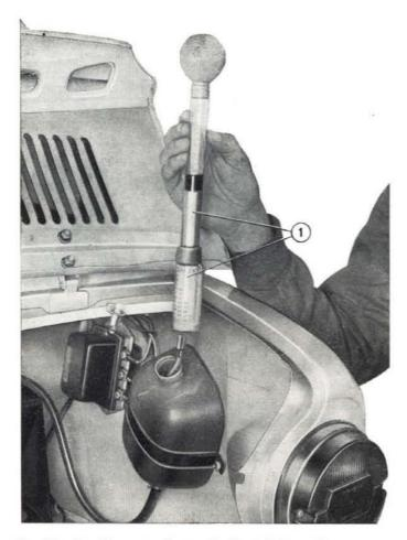
Fig. 131 - Checking rate of « Paraflu 11 » fluid in cooling system. 1. Device A. 95858 for checking « Paraflu 11 » rate.
