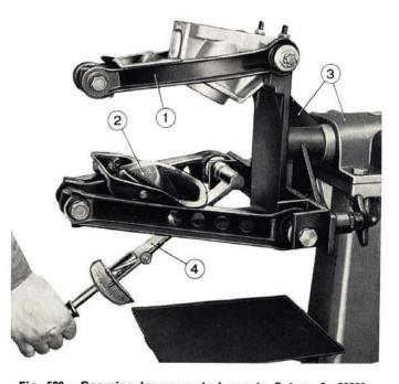
Fig. 529 - Securing lower control arm to fixture A. 22229. 1. Upper control arm. - 2. Coil spring housing. - 3. Fixture A. 22229. -4. Torque wrench.
