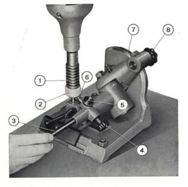
Fig. 92 - Dressing taper grindwheel A. 94084 on dressing machine Ap. 5050.
