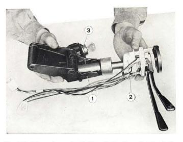
Fig. 490 - Removing outer light and direction signal selector switch from steering column.
