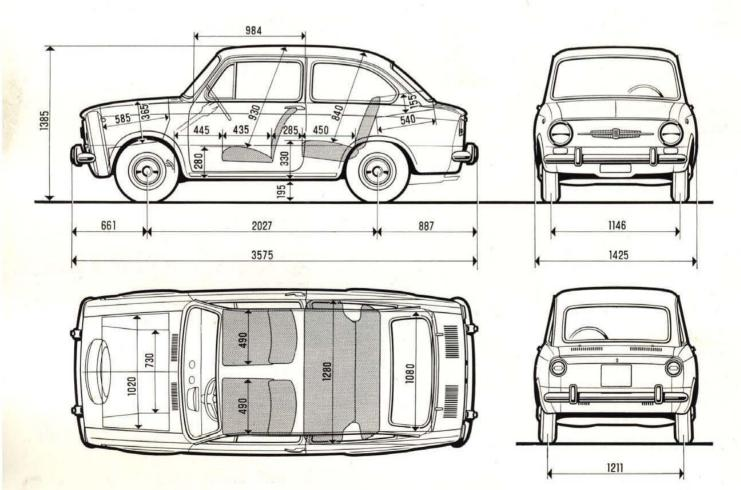
Fig. 2 - Leading dimensions of car (metric). Overall height applies to an unloaded vehicle.
