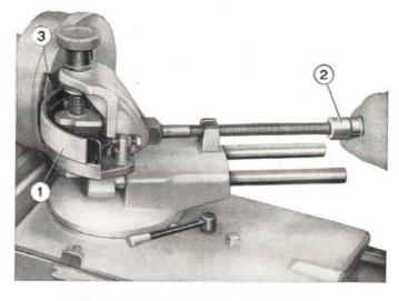
Fig. 297 - Refacing brake shoe linings. 1. Shoe lining. - 2. Carriage operating bar. - 3. Stone of refacer Ap. 5031.
