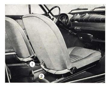
Fig. 420 - Detail of front seat back rest catch. 1. Catch release utton. - 2. Striker plate.
