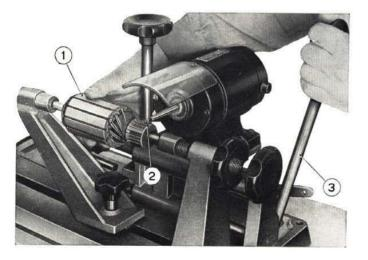
Fig. 323 - Undercutting mica between commutator bars using fixture Ap. 5015. 1. Armature. - 2. Cutter. - 3. Cutter arm actuating lever.
