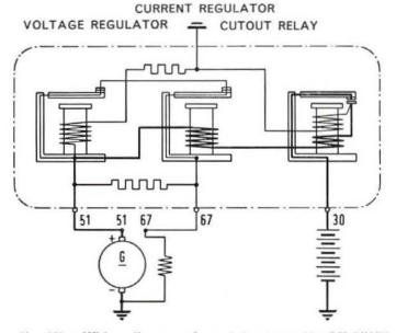
Fig. 332 - Wiring diagram of regulator assembly GN 2/12/16.
