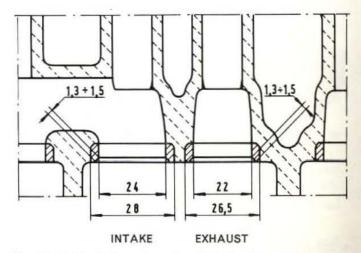
Fig. 90 - Critical dimensions (metric) of valve seats in head.
