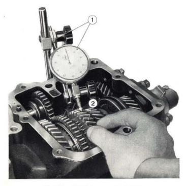
Fig. 175 - Checking gear backlash. 1. Magnetic dial indicator. - 2. Second driven gear.
