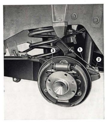
Fig. 301 - Handbrake components at left side rear wheel. 1. Handbrake control cable. - 2. Actuating lever return spring. -3. Shoe actuating segment, manually controlled.
