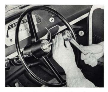
Fig. 271 - Backing out steering wheel mounting nut. 1. Ratchet wrench A. 89854. - 2. Horn button wire.
