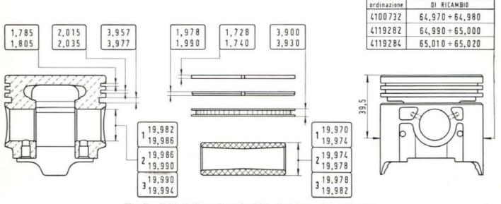
Fig. 43 - Critical dimensions (metric) of pistons, pins and rings.
