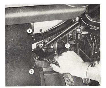
Fig. 445 - Removing steering column joint shield. 1. Steering column flexible joint. - 2. Joint shield. - 3. Upper steering shaft.
