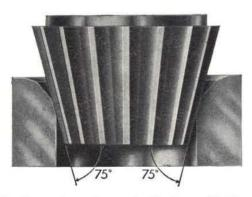
Fig. 97 - Narrowing valve seat at bottom with 75° cutter.
