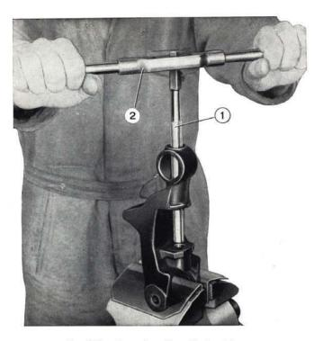
Fig. 221 - Reaming kingpin bushings. 1. Reamer A. 90316. - 2. Reamer handle.
