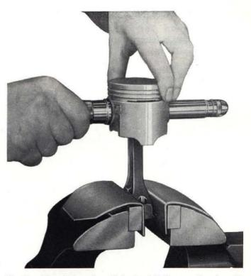
Fig. 55 - The piston pin will be installed correctly when the shoulder of tool A. 60275 abuts against the piston boss.
