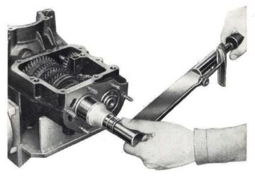
Fig. 180 - Using torque wrench to tighten the countershaftdrive pinion nut.
