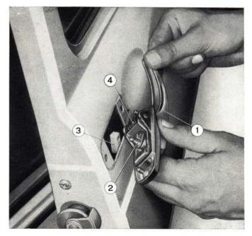
Fig. 394 - Removing door handle. 1. Handle. - 2. Control cable ball pin. - 3. Control cable adjustable end. - 4. Handle return spring.
