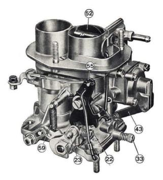
Fig. 432 - Carburetor viewed from the throttles control end. 22. Throttle stop screw. - 23. Throttles control lever. - 33. Idle volume control screw. - 43. Accelerator pump control lever. -52. Choke throttle valve. - 55. Choke control lever. - 59. Primary sector return spring.
