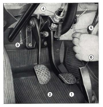
Fig. 159 - Removing clutch throwout yoke rod.
