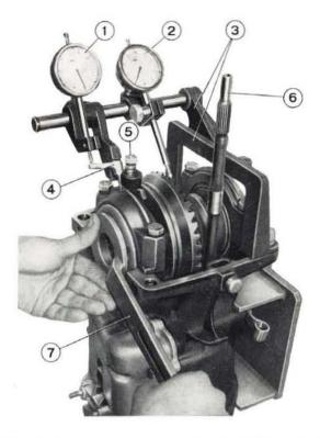
Fig. 197 - Setting differential cage bearing preload by means of fixture A. 95688.
