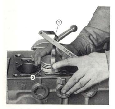
Fig. 40 - Checking piston clearance in cylinder bore. 1. Feeler gauge A. 95316. - 2. Piston.
