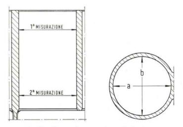
Fig. 27 - Diagram for measuring cylinder bores.  $1^a = First - 2^a = Second - Misurazione = Measurement$
