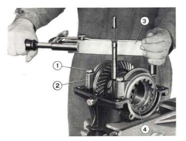
Fig. 189 - Tightening differential carrier cap screws. 1. Cap screw. - 2. Cap. - 3. Torque wrench. - 4. Roller bearing adjuster.
