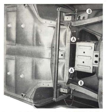
Fig. 414 - Detail showing use of gauge A. 74141 for checking underbody front.
