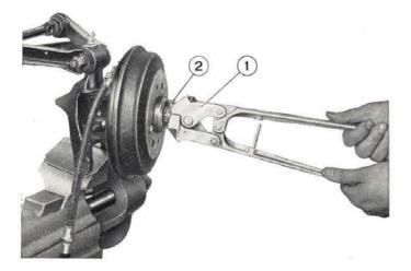
Fig. 229 - Staking steering knuckle nut. 1. Nut staking pliers A. 74128. - 2. Steering knuckle nut.
