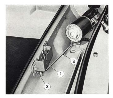
Fig. 515 - Close-up view of engine compartment lid catch and release control.
