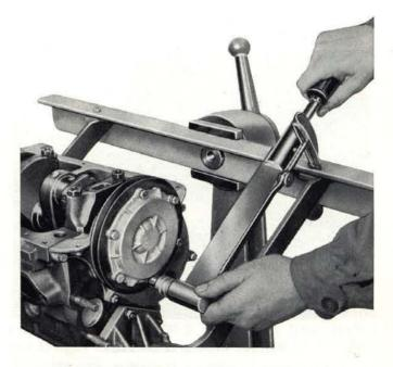
Fig. 22 - Tightening centrifugal oil filter cover.
