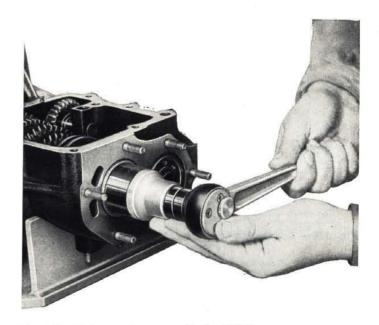
Fig. 174 - Using ratchet wrench A. 89854 to remove countershaft nut.
