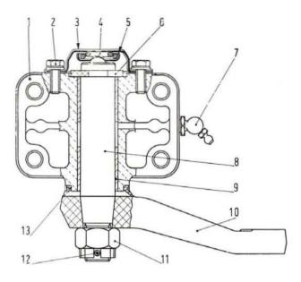
Fig. 538 - Sectional view of idler arm and support assembly.
