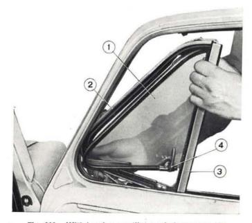
Fig. 390 - Withdrawing ventilator window assembly. 1. Ventilator window pane. - 2. Ventilator window frame. - 3. Division bar. - 4. Ventilator stop handle.
