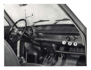
Fig. 467 - Radio assembly installed on car.
