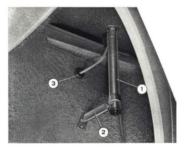
Fig. 466 - Detail showing antenna mounting. 1. Antenna. - 2. Antenna mounting bracket. - 3. Antenna-to-radio receiver cable.
