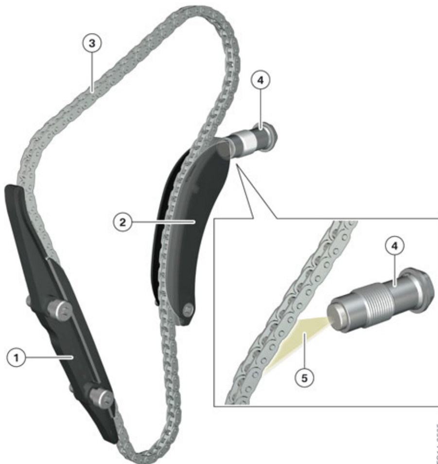
Lubrication of top chain drive, B46 engine
