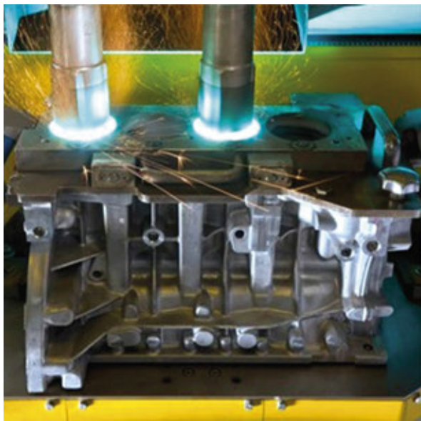
Electric arc wire spraying method, Bx8 engine
