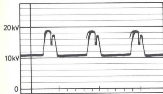
Break at one exciter diode.
