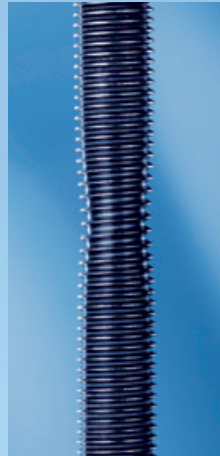
Plastically elongated and tapered cylinder-head bolt
