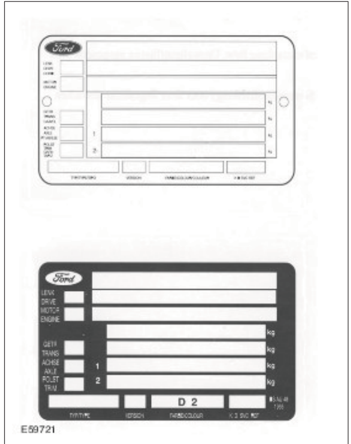
On the newer type plates, the color code is given in the left-hand column, at the penultimate position.
