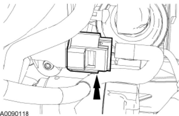
Fig. 451: Identifying Temperature Manifold Absolute Pressure Electrical Connector Courtesy of FORD MOTOR CO.
