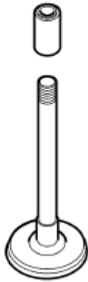
Fig. 114: Installing Valve Stem Seal Courtesy of FORD MOTOR CO.
