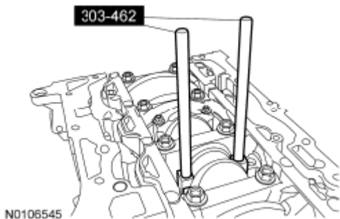
Fig. 341: Removing Piston/Rod Assembly From Engine Block Courtesy of FORD MOTOR CO.
