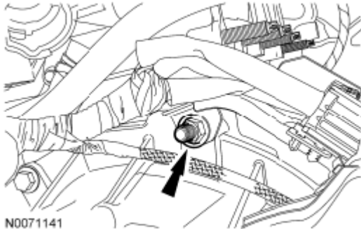
Fig. 263: Locating CMS Wire Connector Bracket And Nut Courtesy of FORD MOTOR CO.
