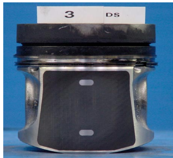
Figure 7: Piston after running for 3000 h
