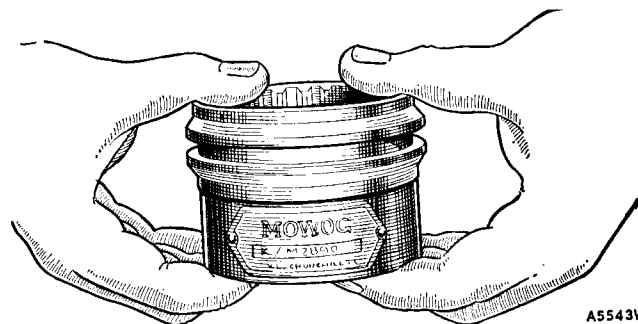
Fig. F.6 Assembling a synchromesh hub, using Service tool 18G 222
