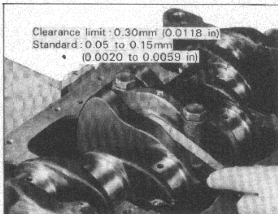
Fig. EM-64 Crankshaft end play check
