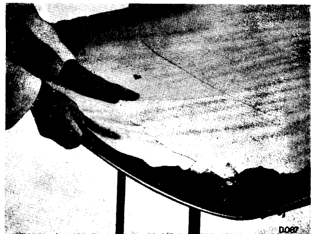
Fig. 51. Fitting front edge of lining
