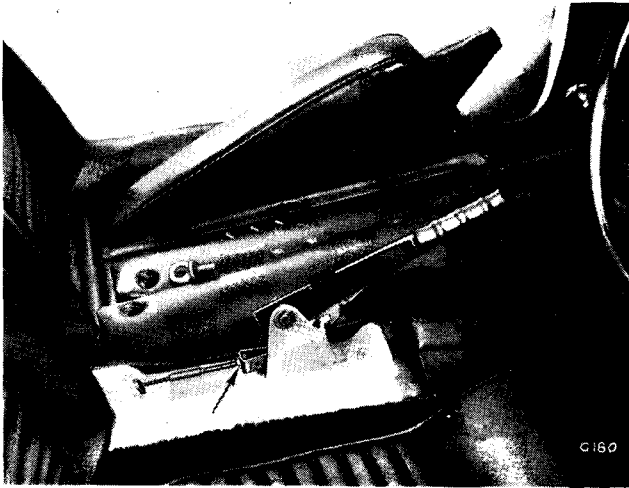
Fig. 23. Primary cable adjuster
