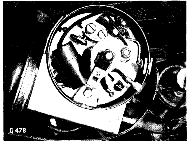
Fig. 66. Distributor rotor arm position at T.D.C. firing on No. 1 cylinder
