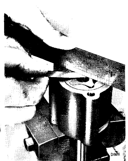
Fig. 37. Measuring rotor end-float
