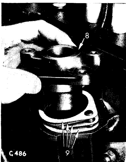
Fig. 64. Fitting packing washer and distributor adaptor
