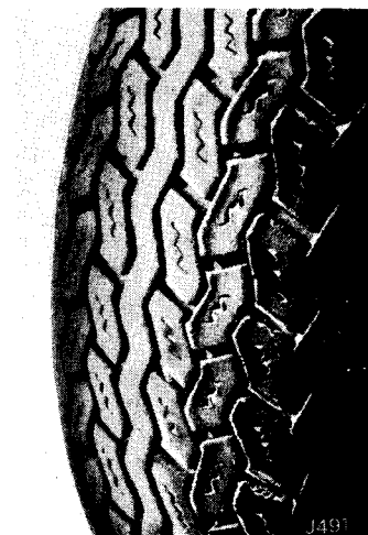
Fig. 11. Tyre wear resulting from wheel misalignment
