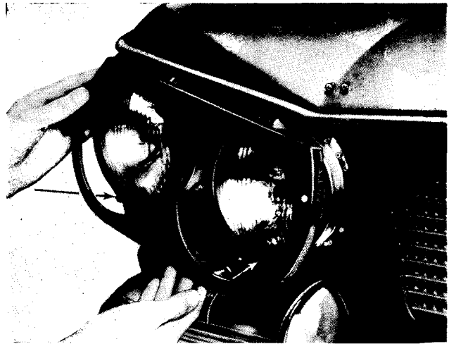
Fig. 24. Remove/install cover panel
