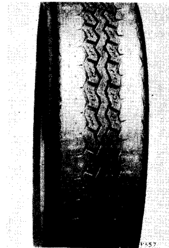
Fig. 9. Tyre wear resulting from under-inflation
