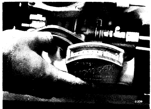
Fig. 13. Using a Crypton "Synchro Check" for balancing the air intake
