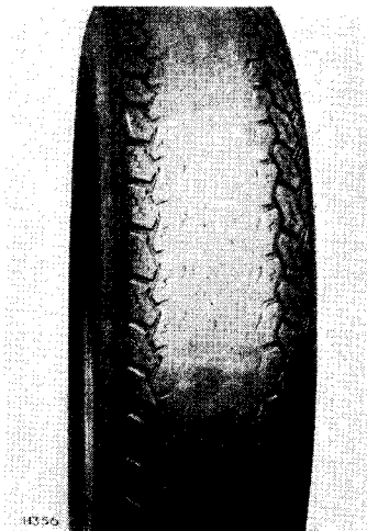
Fig. 10. Tyre wear resulting from over-inflation
