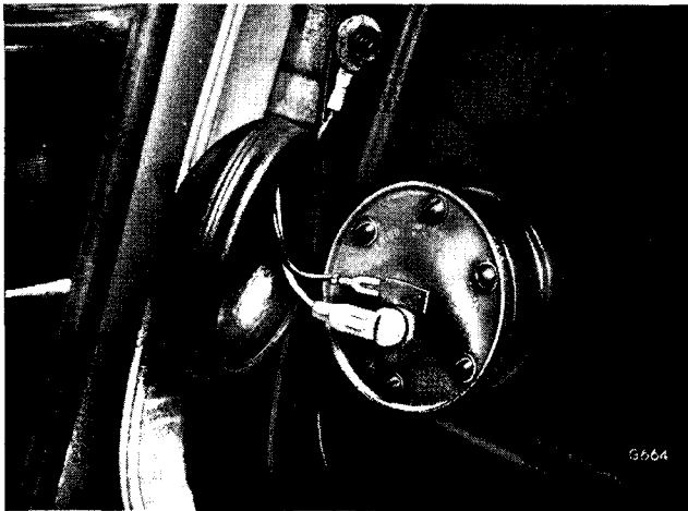
Fig. 46. Tank unit installed
