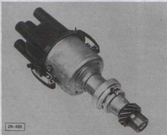
Hall TCI distributor for long cylinder head: for engines with code letters WC, Part No. 035 905 206 M
