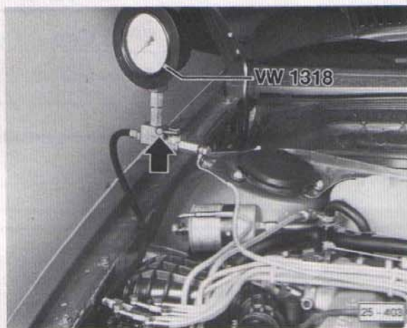
Fig. 3 Pressure gauge valve in closed position
