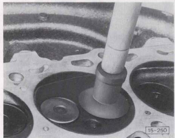
Fig. 5 Grinding valves in
