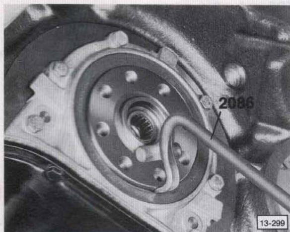
Fig. 8 Removing oil seal, flywheel end
