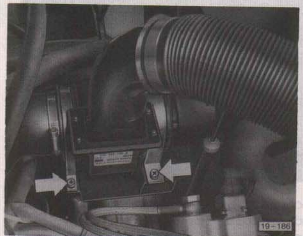
- Install blower motor on bracket. - Attach air hose and intake hose to blower motor.
