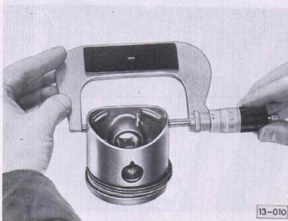
Fig. 6 Measuring piston Measure 10 mm from lower edge and at 90° to pin axis. Wear limit: 0.04 mm below nominal dimension (on crown) Fitting clearance 0.025 mm, wear limit 0.07 mm
