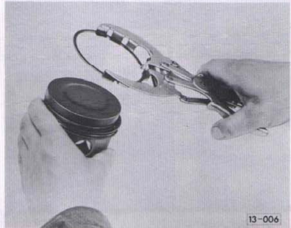
Fig. 10 Removing and installing rings
