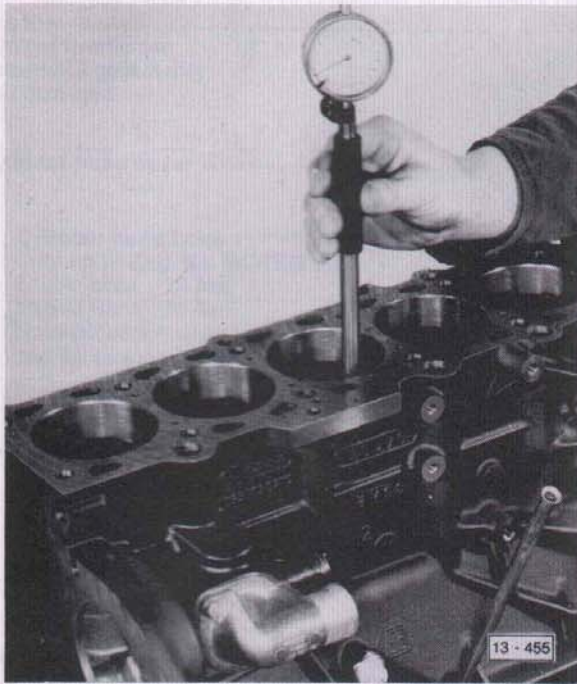
Fig. 13 Measuring bores - Measure with internal dial gauge
