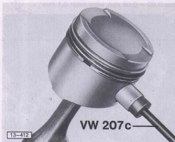
Fig. 5 Removing and installing piston pin
