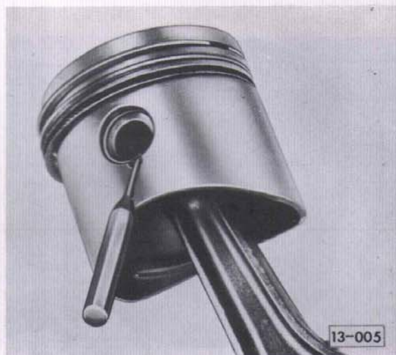
Fig. 4 Levering circlip out
