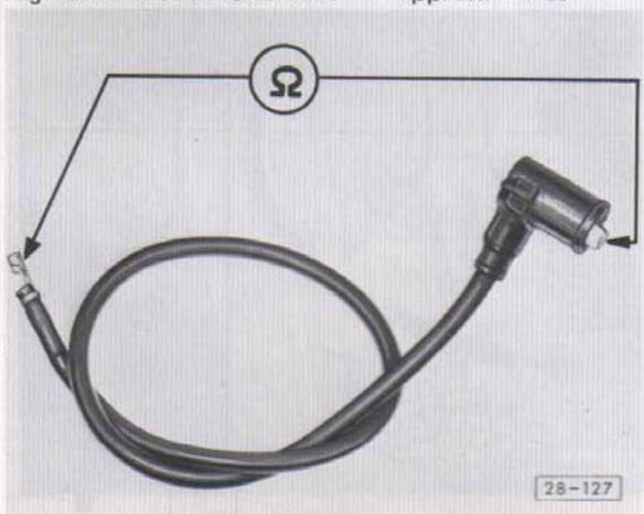
Fig. 3: Checking ignition leads
