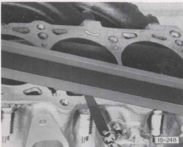
Fig. 2 Checking head for distortion
