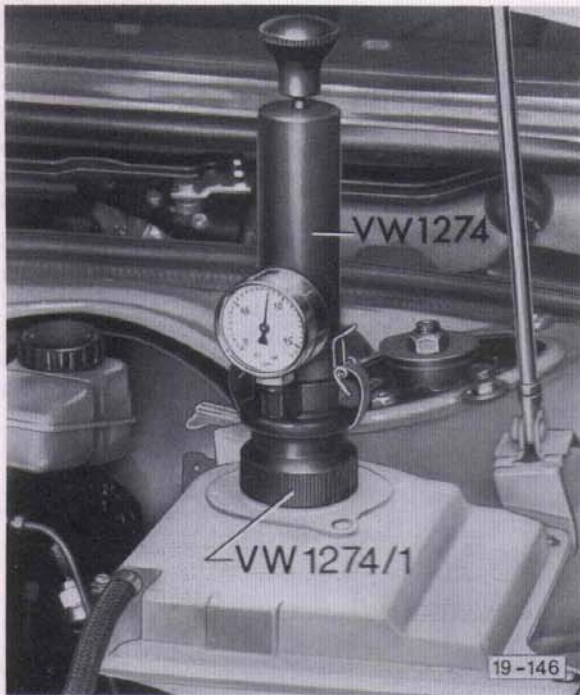
Fig. 1 Checking cooling system for leaks Always test with engine warm.
