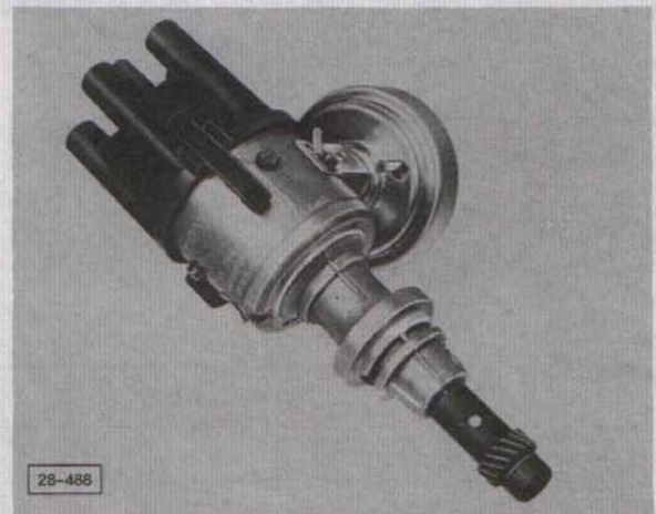
Hall TCI distributor for short cylinder head: for engines with code letters WC, Part No. 035 905 206
