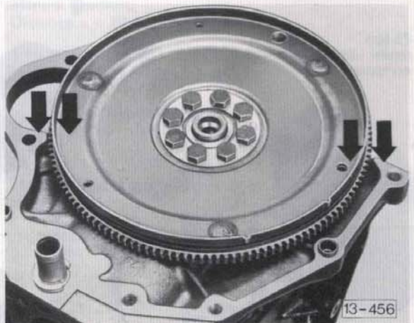
Fig. 5 Measure distance from drive plate to engine block in two places
