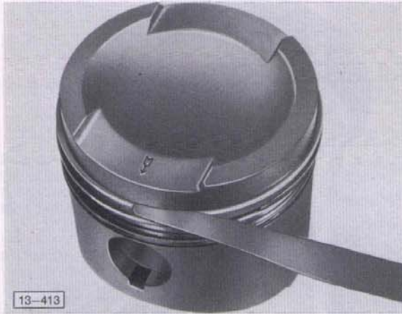
Fig. 7 Measuring ring clearance New 0.02 – 0.08 mm, wear limit 0.1 mm
