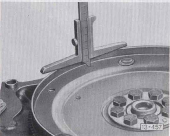
Fig. 3 Measuring distance from drive plate, inside
