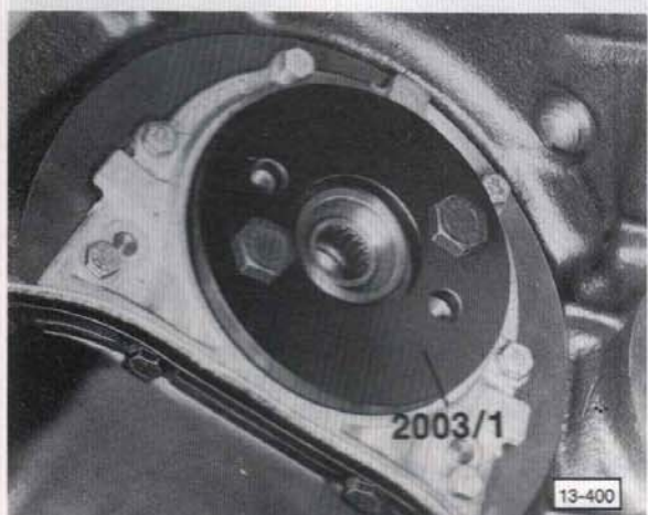
Fig. 9 Installing oil seal, flywheel end
