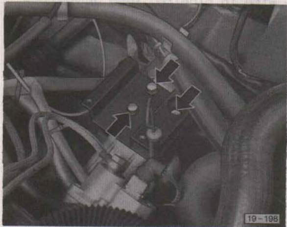
- Mount bracket for blower motor on left engine support (M 8 x 16 bolts, 8 x 16 x 2 washers). Tightening torque: 25 Nm
