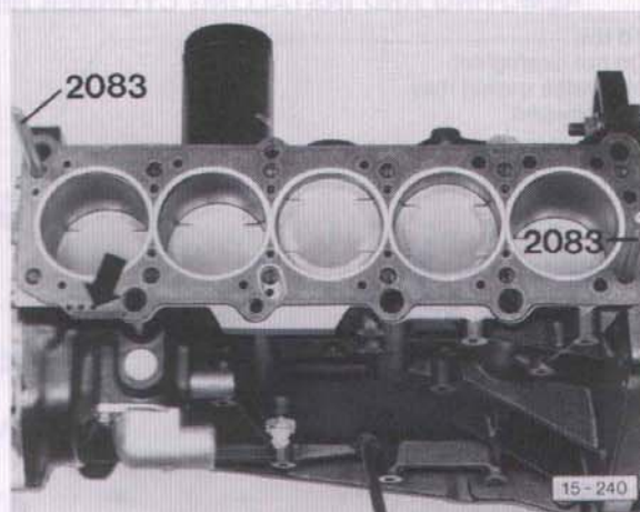
Fig. 3 Position of head gasket
