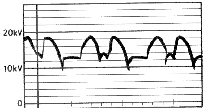
Positive diode short circuited.
