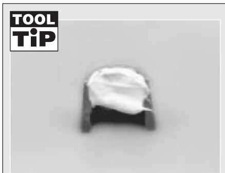
TOOL TIP Apply a small dab of grease to each collet to hold it in place, if necessary.
