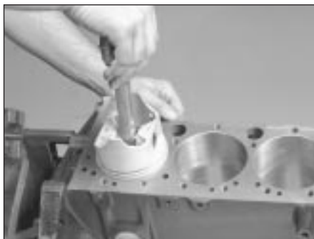
22.3 When checking piston ring end gap, the ring must be square in the cylinder bore (this is done by pushing the ring down with the top of a piston as shown)
