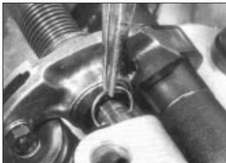
8.7 Remove the retaining clips from the rocker arms - the wire-type clip is shown here
