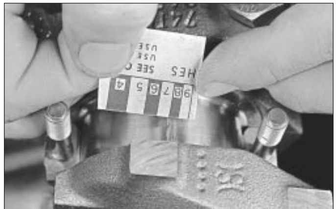
26.17 Measuring the width of the crushed Plastigage to determine the big-end bearing oil clearance (be sure to use the correct scale - standard and metric ones are included)
