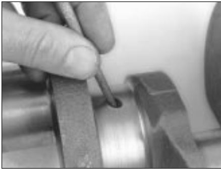
19.1 The oil holes should be chamfered so sharp edges don't gouge or scratch the new bearings
