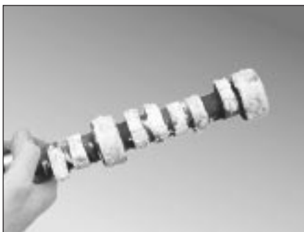
11.9 Lubricate the camshaft bearing journals and lobes with engine assembly paste or molybdenum disulphide ("moly") grease
