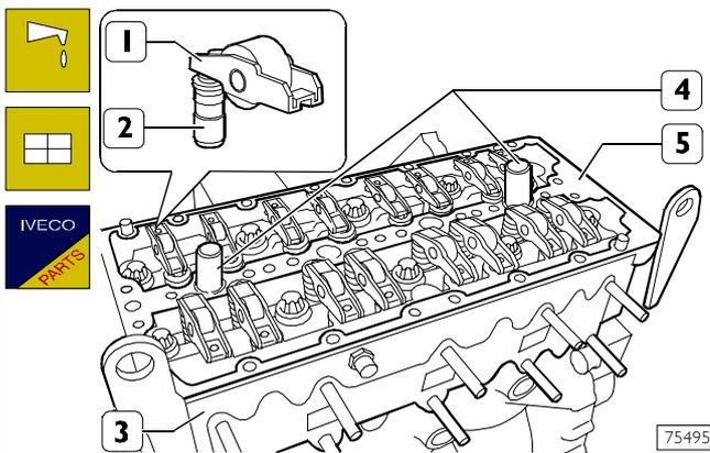
Thoroughly clean the hydraulic tappets (2), lubricate them and fit them in the cylinder head (3), positioning the rocker arms (1) on the valves correctly.
