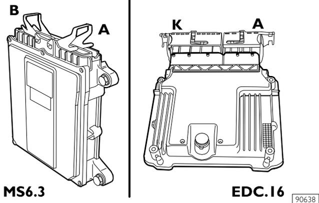
The control unit is a "flash EPROM" and so it can be reprogrammed from outside without changing the hardware. It processes the signals from the sensors by applying software algorithms and controls the actuators (especially the electro-injectors and pressure regulator).
