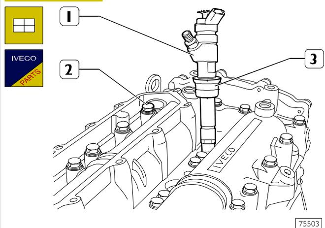
Fit a new seal (3) on the electro-injector (1) and mount this in the overhead (2).
