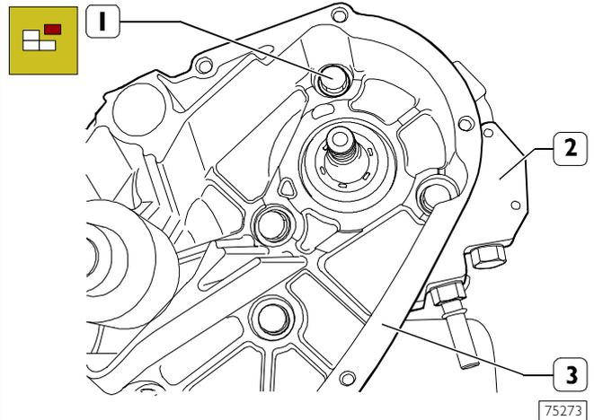
Take out the screws (1) and remove the high-pressure pump (2) from the water pump mounting (3).
