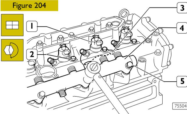
Mount the brackets (3) fastening the electro-injectors (1) and screw down the screws (2) without locking them. Mount the hydraulic accumulator (4) and tighten the fixing screws to the prescribed torque.
