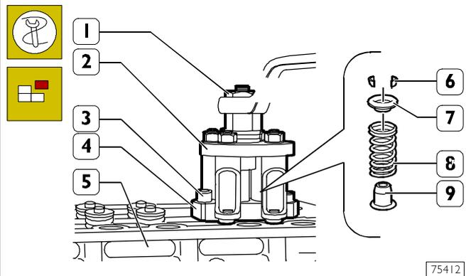
Fit part (4) of tool 99360260 onto the cylinder head (5) and secure it with the screws (3).
