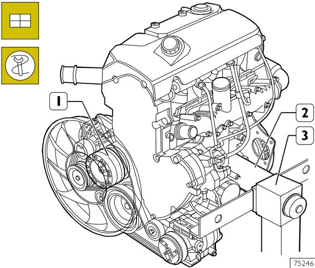
Fit the cooling fan (1) back onto the electromagnetic coupling. Fit the arm 99360549 onto the engine lifting hooks. Hook the arm onto the hoist and remove the engine from the rotary stand (3). Take out the brackets 99361028 (2).
