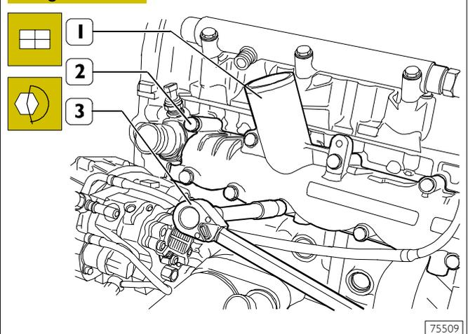
Mount the intake manifold (1) with a new gasket and, using a torque wrench (3), tighten the fixing screws (2) to the prescribed torque.
