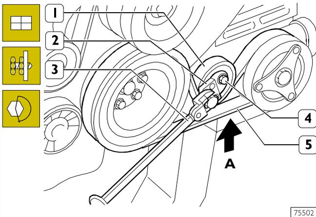
Mount the drive belt, taking care to position its ribs properly in the respective races of the pulleys.
