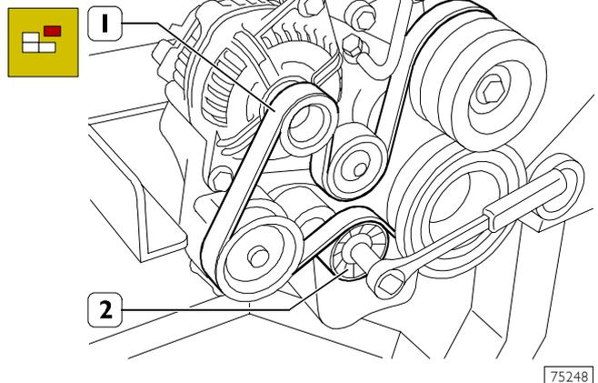
Disassemble the compressor drive belt, if there is one, as described under the relevant heading.
