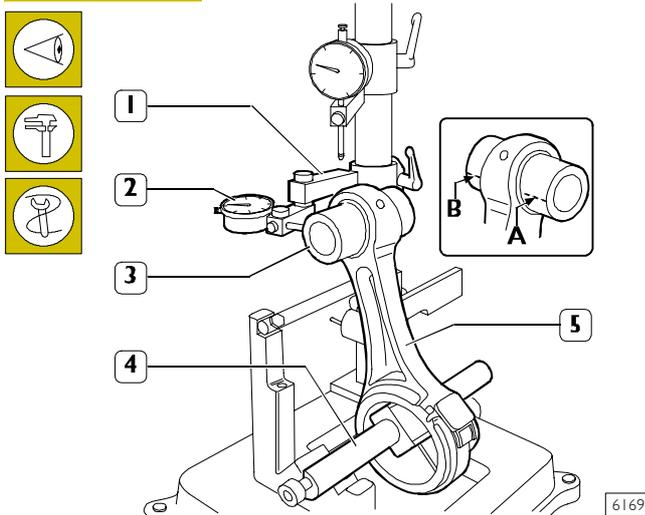
Check the torsion of the connecting rod (5) by comparing two points (A and B) of the pin (3) on the horizontal plane of the axis of the connecting rod.
