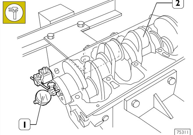
The end float is checked by setting a dial gauge (1) with a magnetic base on the crankshaft (2) as shown in the figure. The normal assembly clearance is 0.060 – 0.310 mm.
