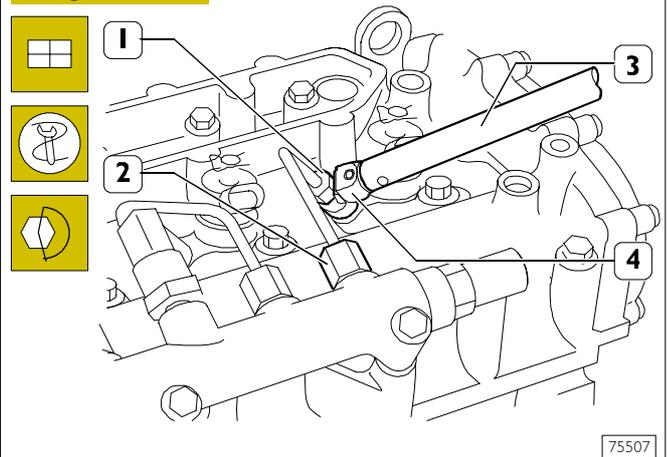
Using the wrench (4) of the 99317915 series and the torque wrench 99389829 (3), tighten the fuel pipe fittings (1) and (2) to the prescribed torque.
