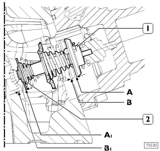
The by-pass thermostat (1) needs no adjustment. If there is any doubt about its operation, replace it. The thermostat casing is fitted with the thermometric switch/transmitter and water temperature sensor.
