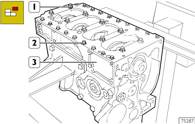
Using an appropriate wrench and a hex-fluted wrench, unscrew the screws (1) and (2) and remove the crankcase base (3).
