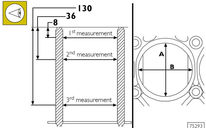
The measurements must be made for each single cylinder at three different heights up the liner and on two planes at right angles to each other: one parallel to the longitudinal axis of the engine (B) and the perpendicular (A); the greatest wear is generally found on this last plane with the first measurement.
