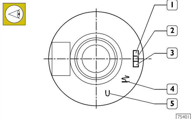
Etched on the top of the piston are: the type of engine (1), class selection (2) and supplier (3) as well as the direction of fitting the piston in the cylinder liner (4). The mark (5) is for passing the 1<sup>st</sup> slot insert adhesion test.
