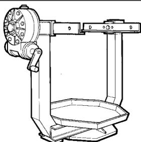
Rotary telescopic stand for overhauling assemblies
