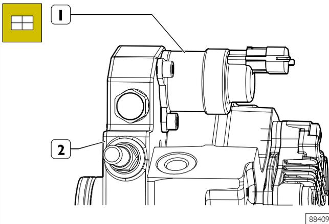
Mount pressure regulator (1) on high pressure pump (2).
