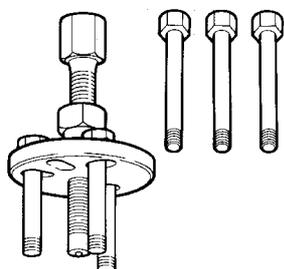
High-pressure pump toothed pulley extractor
