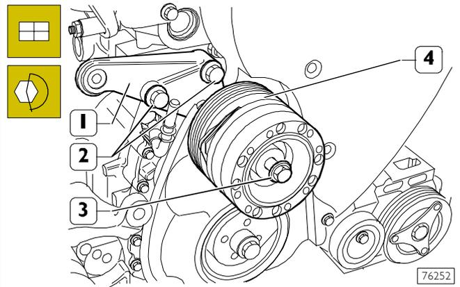
Fit on the mounting (1) together with the electromagnetic coupling (4) and tighten the fixing screws (2 and 3) to the prescribed torque.
