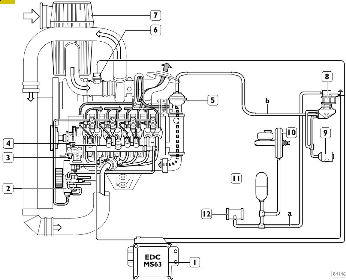
a. Brake booster vacuum circuit - b. EGR modulated vacuum circuit
