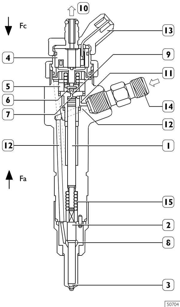
1 Pressure rod – 2 Pin – 3 Nozzle – 4 Coil – 5 Pilot valve –
