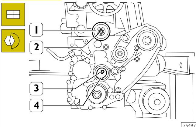
Mount the fixed tightener (1) and tighten the fixing screw (2) to the prescribed torque.
