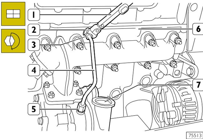
Connect the pipe (4) to the cylinder head (6) and to the turbocharger (7).
