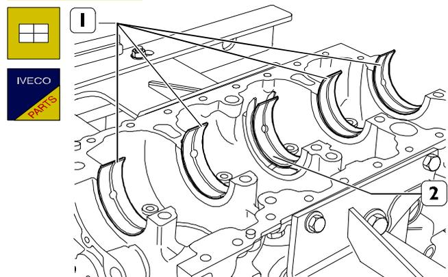
**NOTE** Not having found it necessary to replace the main bearings, they need to be fitted back on in the same sequence and position found upon disassembly.
