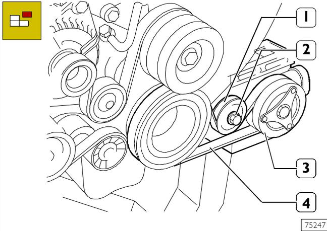
Set the vehicle on a lift or over a pit. From underneath the vehicle, detach the middle soundproofing guard. Loosen the screw (2) fixing the tightener (1) and remove the belt (4) driving the air-conditioner compressor (3).
