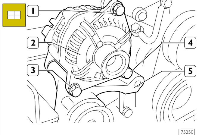
Position the alternator (2) on the mounting (5) and secure it with the bottom screws (3 and 4) and the bolt.
