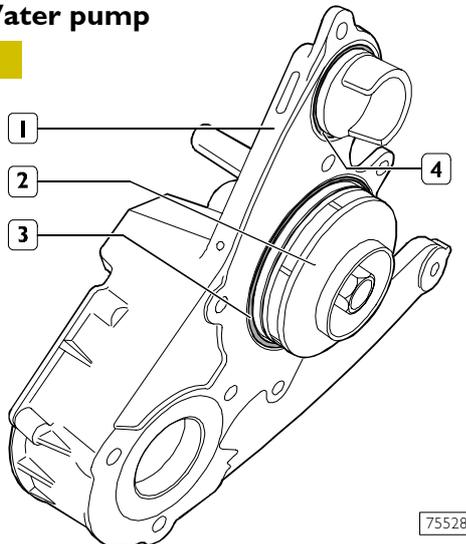
The water pump (3) cannot be overhauled. In case of coolant leaking from the seal or damage, it must be replaced. The water pump casing (1) is also used as a mounting for the high-pressure pump. The seals (3 and 4) must always be replaced.
