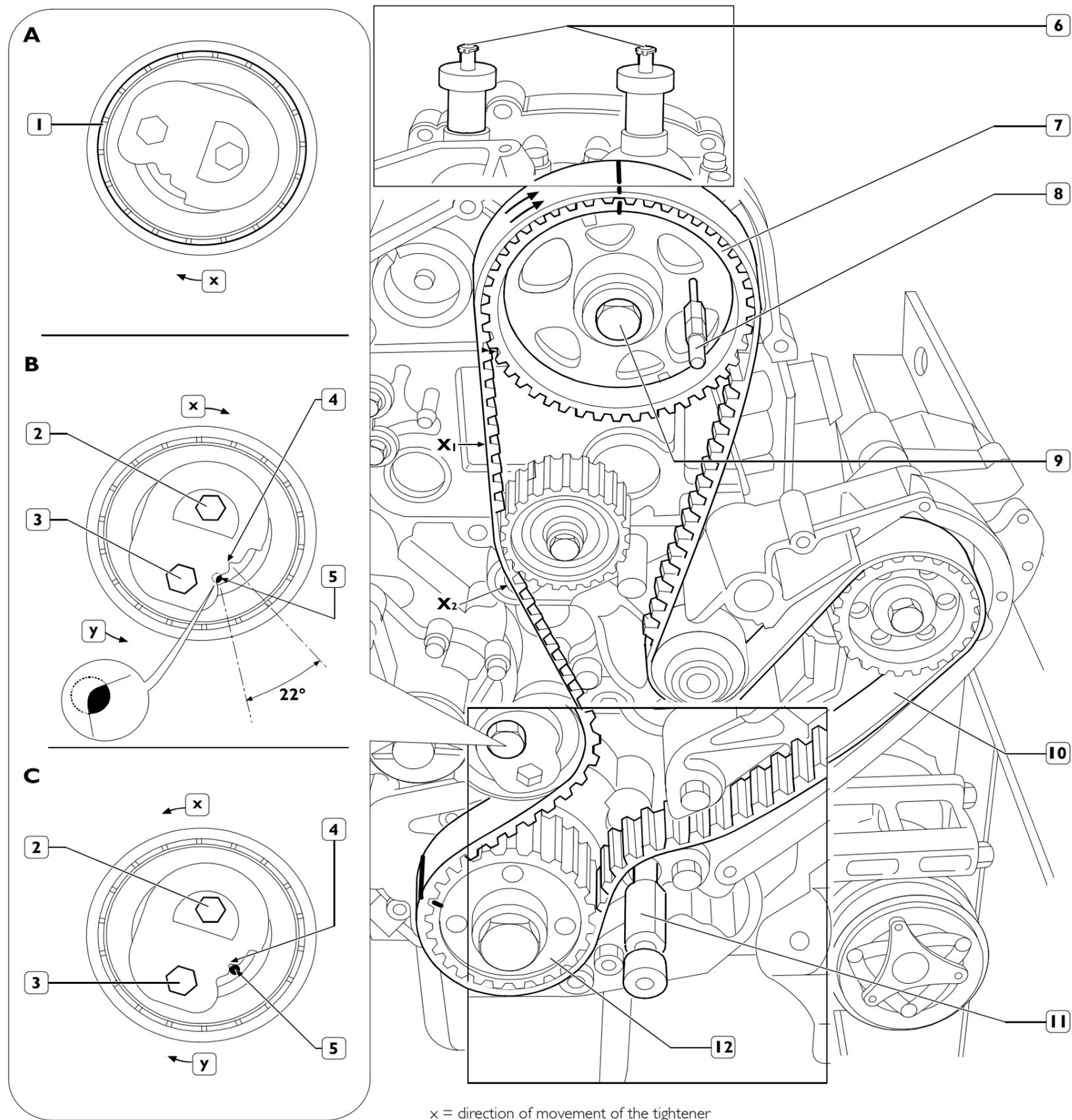
x = direction of movement of the tightener
