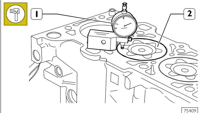
After mounting the connecting rod – piston assemblies, check the protrusion of the pistons (2) at the T.D.C. in relation to the top surface of the crankcase with a dial gauge (1).
