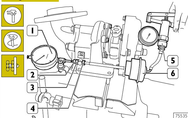
Rest the tip of the dial gauge (1) with a magnetic base on the end of the tie rod (2) and zero it. Using the device 99367121 (5), introduce compressed air into the valve casing (6) at the prescribed pressure and make sure this value stays constant throughout the check; replace the valve if it doesn't. In the above conditions, the tie rod must have made the prescribed travel. On finding a different value, use the nuts (3 and 4).
