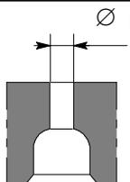
Guide valve seats on cylinder head                                                                                  | Ø 1                                                                                                                                                                                          |            | 9.980 ÷ 10.000                                                   |            |
