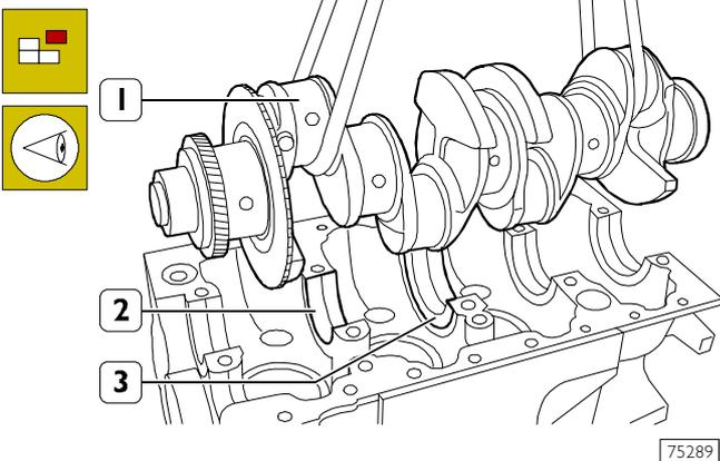
With the aid of a hoist and a rope, remove the crankshaft (1).
