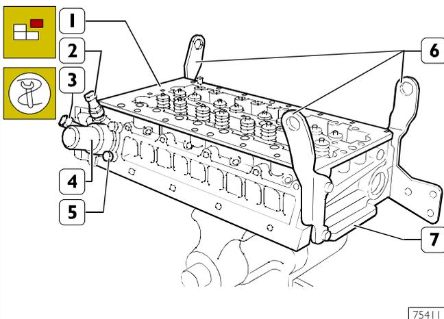
Place the cylinder head (1) on the mounting SP.2271 (7). Remove the brackets (6) for lifting the engine.
