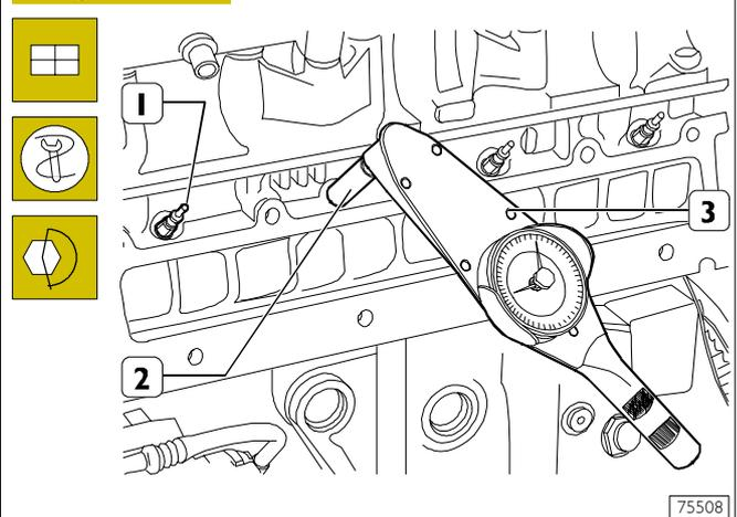
Mount the glow plugs (1) and, using the box-type wrench SP. 2275 (2) and torque wrench 99389819 (3), tighten them to a torque of  $8 \pm 10$  Nm.
