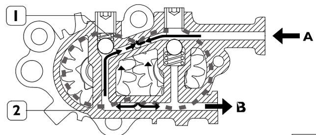
The by-pass valve (1) trips when overpressure is generated at the outlet B. The pressure, overcoming the elastic resistance of the spring of the valve (1), sets the outlet in communication with the inlet via the duct (2).
