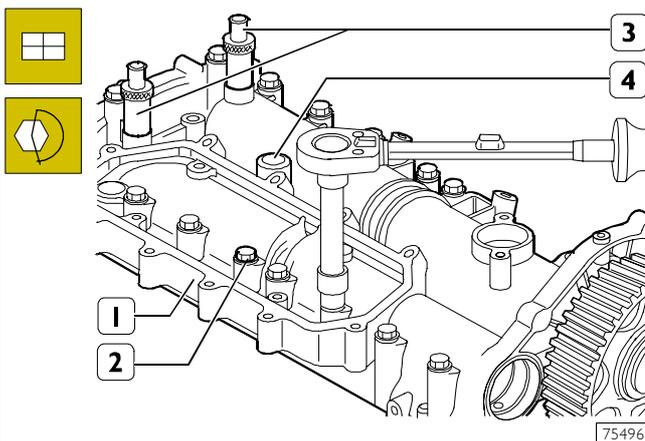
Mount the overhead (1) together with the tools 99360614 (3) for the timing and tighten the fixing screws (2) to the prescribed torque.
