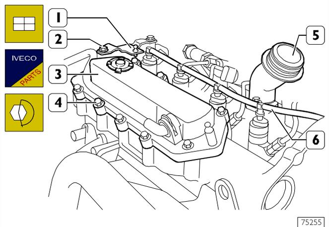
Mount the oil fillpipe (5) with a new seal and tighten the nuts (6) to the prescribed torque.
