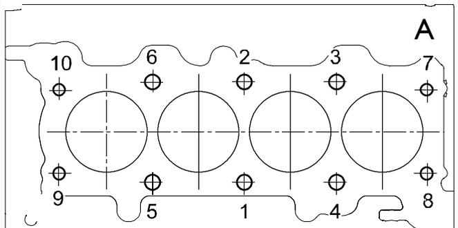
Diagram of the tightening sequence for the cylinder head fixing screws:
