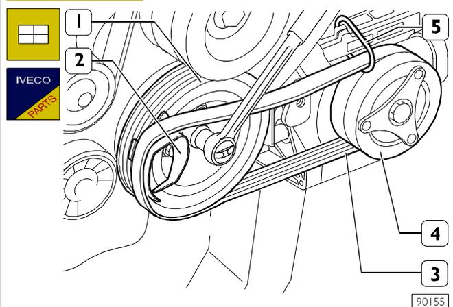
Fit the flexible belt (3) equipped with tool 99360191 (2) on the pulley (4) and apply the tool on the pulley (1).
