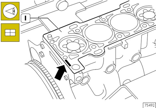
Check that the mating surfaces of the cylinder head and crankcase are clean.
