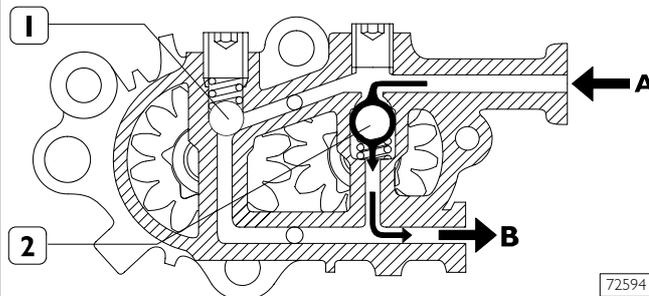
The by-pass valve (1) trips when, with the engine switched off, you want to fill the supply system via the priming pump. In this situation, the by-pass valve (2) opens, due to the effect of the inlet pressure, and the fuel flows out via the outlet B.
