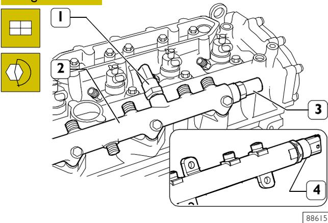
Forged version: on hydraulic accumulator (2), mount: pressure sensor (1) tightening it at  $35 \pm 5$  Nm torque, and pressure relief valve (3) tightening it at  $27 \pm 2$  Nm torque. Welded version: mount pressure sensor and tighten it at  $70 \pm 5$  Nm torque.
