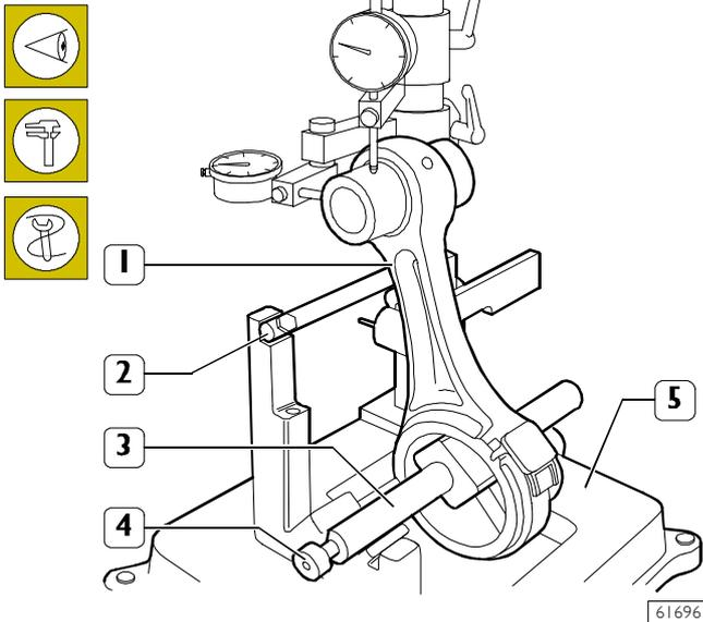
Check the alignment of the axes of the connecting rods (1) with device 99395363 (5), proceeding as follows:
