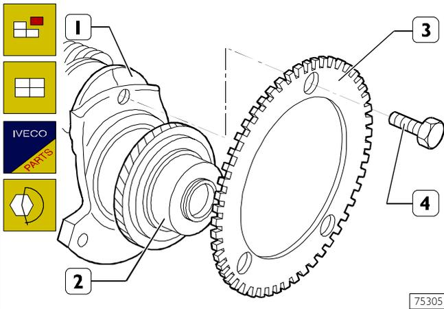
Take out the screws (4) and replace the phonic wheel (3). The screws (4) are coated with LOCTITE 218 and must be replaced with fresh ones after each disassembly. They must be tightened to a torque of 15 Nm.
