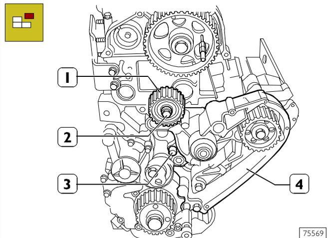
Take out the screw (2) and remove the fixed tightener (1). Take out the screws (3) and remove the water pump mounting (4).
