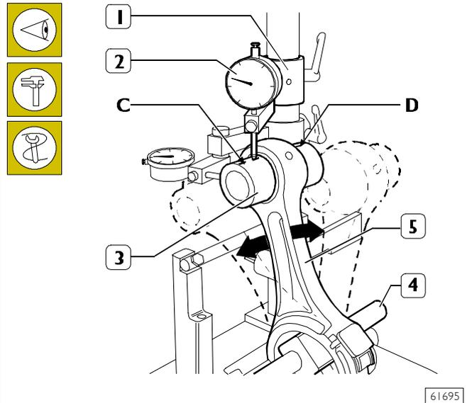
Check the bending of the connecting rod (5) by comparing two points C and D of the pin (3) on the vertical plane of the axis of the connecting rod.
