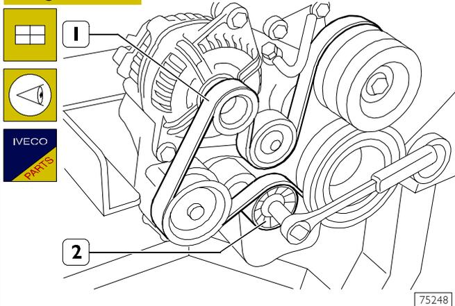
Using a wrench on the automatic tightener (2), mount the drive belt (1), taking care to position its ribs correctly in the respective races of the pulleys.
