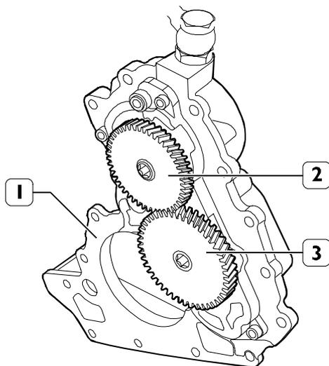
The oil pump (3) is a gear pump driven directly by the crankshaft.
