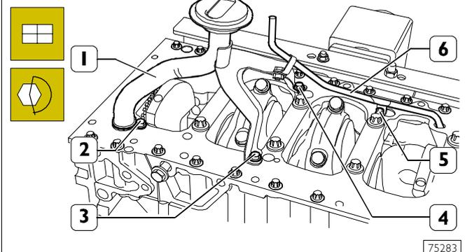
Mount the suction strainer (1) together with the pipe (6). Screw down the fixing screws (2-3-4-6) and tighten them to the prescribed torque.
