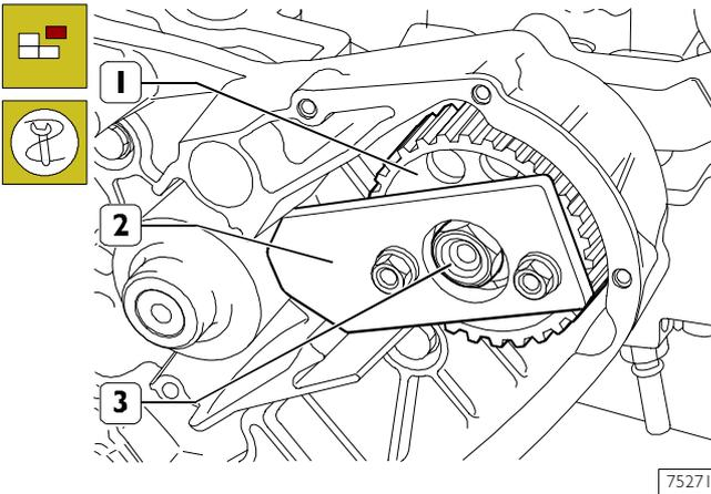
Lock rotation of the high-pressure pump gear (1) by applying tool SP. 2263 (2) as illustrated in the figure. Remove the nut (3) and take out the tool (2).
