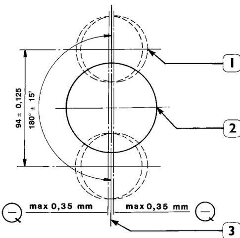
**NOTE** The checks on the tolerances indicated in the figures must be made after grinding the crankshaft pins.
