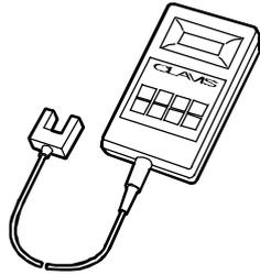
Device for checking belt tension
