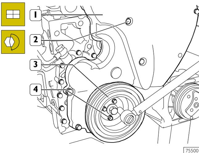
Mount the timing cover (1) and tighten the screws (2) to the prescribed torque.
