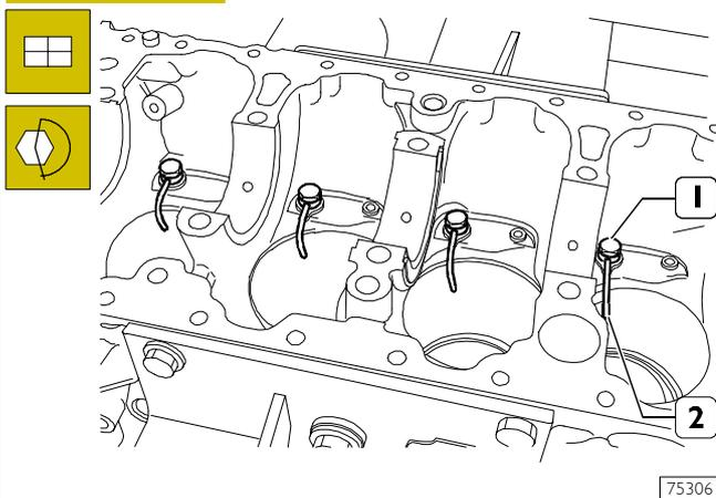
Fit on the oil spray nozzles (2) and tighten the couplings (1) to the prescribed torque.
