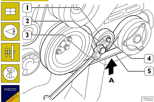
Fit the tightener (1) without tightening the screw (4).
