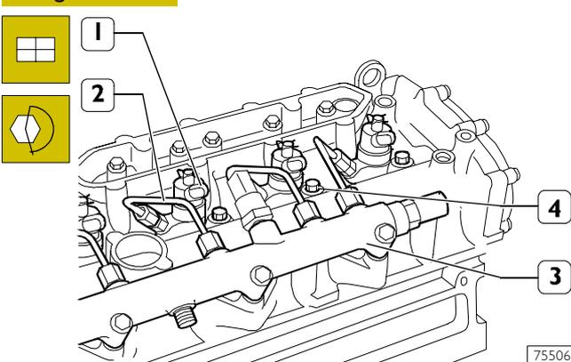
Connect the fuel pipes (2) to the electro-injectors (1) and to the hydraulic accumulator (3). Tighten the screws (4) fixing the electro-injector brackets to the prescribed torque.
