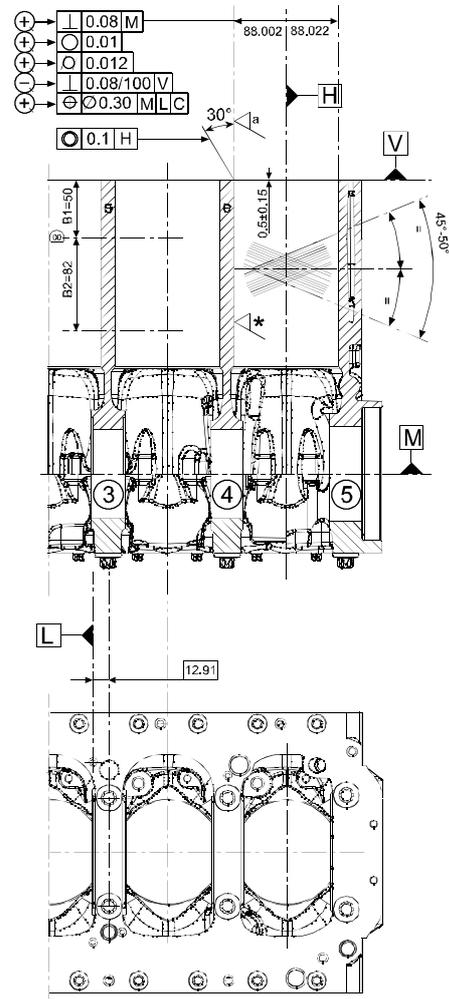
**Checking head mating surface on cylinder block**
