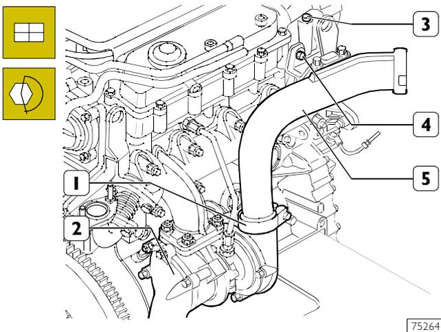
Connect the air duct (5) to the turbocharger (2) and to the overhead (3).
