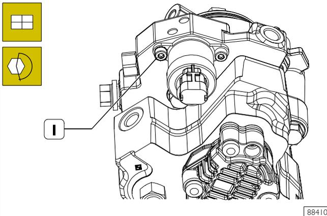
Screw up screws (1) and tighten them at  $6 \pm 7$  Nm ( $0.6 \pm 0.7$  kgm) torque.
