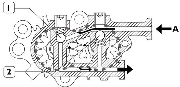
A. Fuel inlet from the tank – B. Fuel outlet to the filter –
