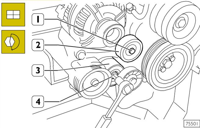
Mount the fixed tightener (2) and tighten the fixing screw (1).
