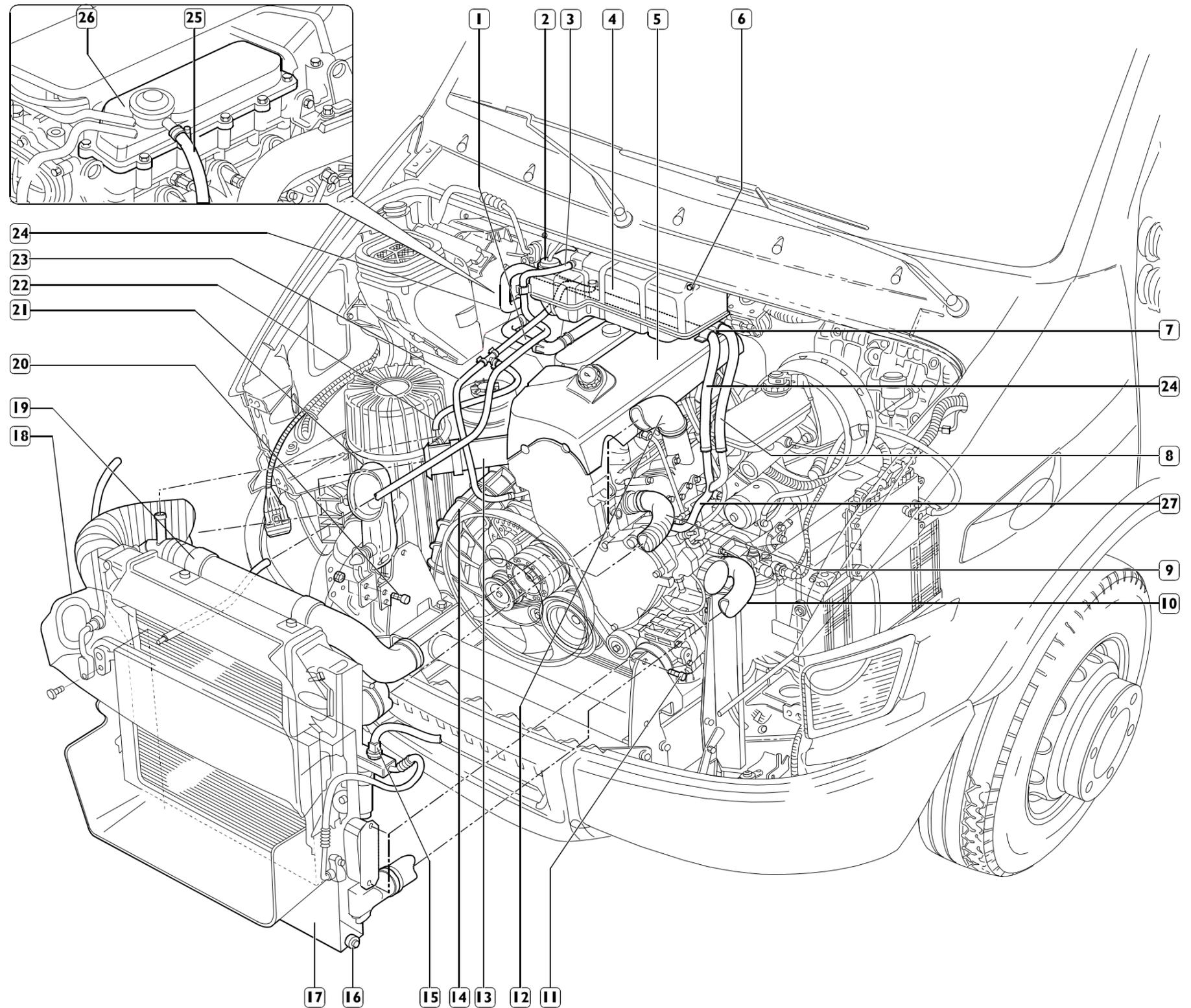
Place a container under the power steering pump to recover the oil from the system. Then disconnect the oil inlet and outlet pipes (16 and 17).
