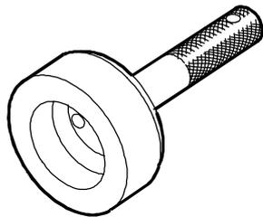
Centring ring for crankshaft front gasket cover
