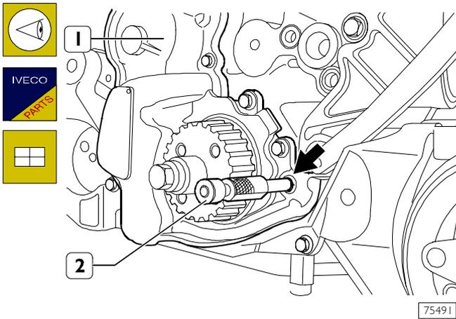
Check that tool 99360619 (2) inserted in the hole (→) of the oil vacuum pump assembly (1) blocks crankshaft rotation.
