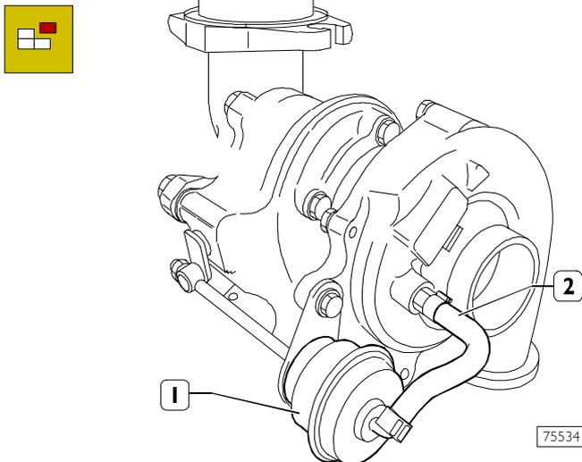
Cover the air, exhaust gas and lubricating oil inlets and outlets. Thoroughly clean the outside of the turbocharger using anticorrosive and antioxidant fluid. Disconnect the pipe (2) from the union of the pressure relief valve (1) and fit on it the pipe of the device 99367121 (1, Figure 239).
