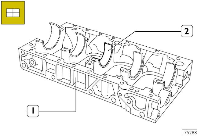
Thoroughly clean the bottom main bearing shells (2) and mount them in the crankcase base (1).
