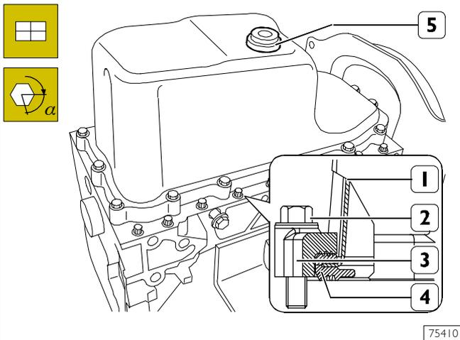
Fit the gasket (4) and the frame (3) onto the oil sump (1). Screw down the fixing screws (2) and tighten them to the prescribed torque. Screw down the oil drain plug (5) and tighten it to the prescribed torque.
