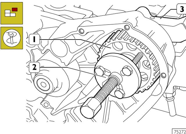
Using tool 99340035 (2) applied as shown in the figure, extract the gear (1) from the shaft of the high-pressure pump (3).
