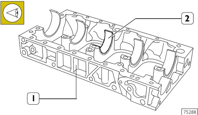
**NOTE** Note the assembly position of the bottom main bearing shells (1) since, if they are reused, they will need to be fitted in the position found during removal.
