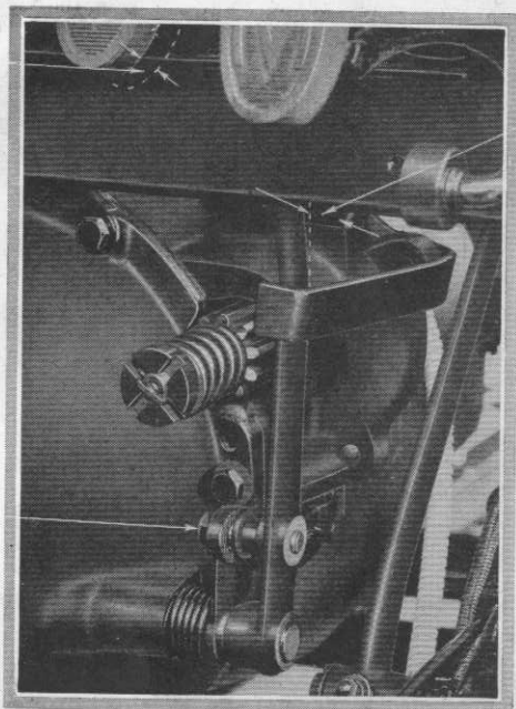
The clutch pedal adjustment on the Morris Eight consists of a slotted lever with serrated face and locating washer.
