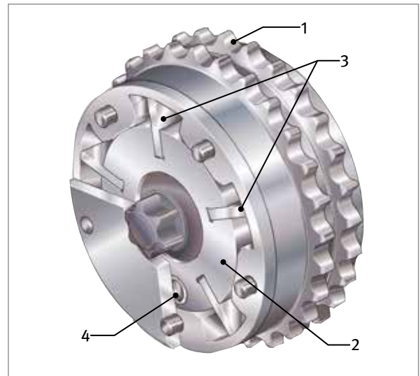
Fig. 54: Chain timing drives
