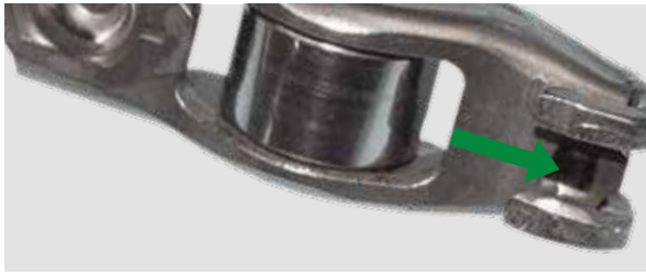
WEAR ON THE VALVE CONTACT FACE OF THE FINGER FOLLOWER
