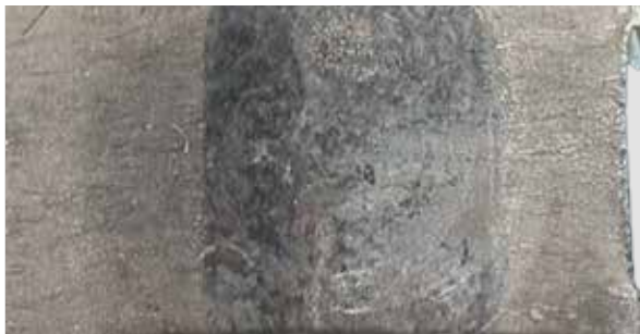
WEAR ON THE VALVE CONTACT FACE OF THE FINGER FOLLOWER
