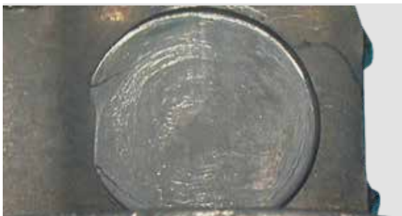
WEAR ON THE OUTER RING OF THE CAM ROLLER
