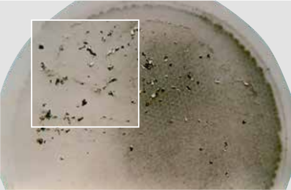
COMBUSTION RESIDUES FROM A DIESEL ENGINE
