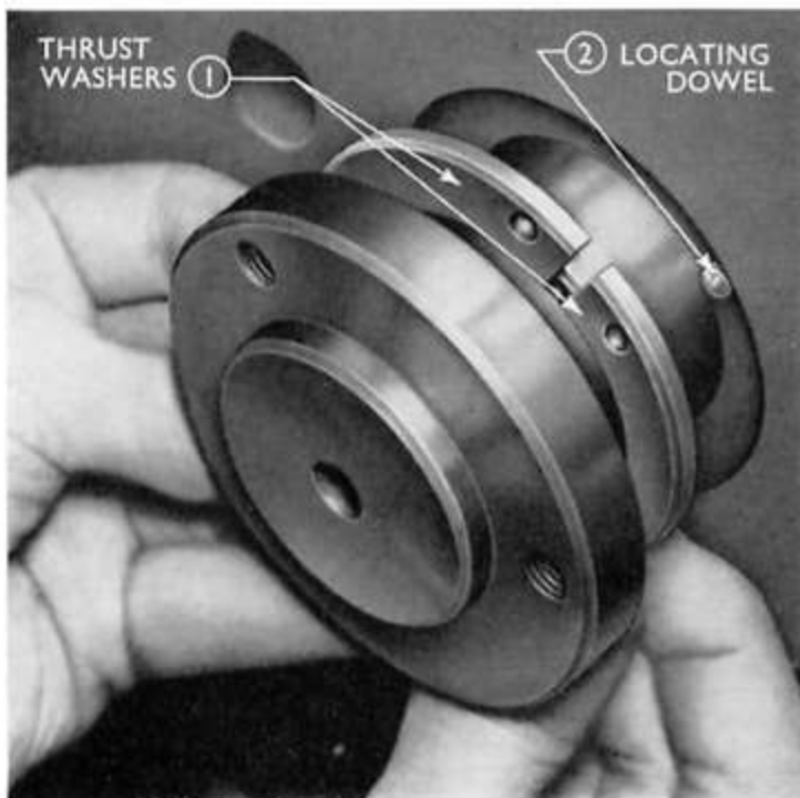
Fig. 51 Camshaft Thrust Washers
