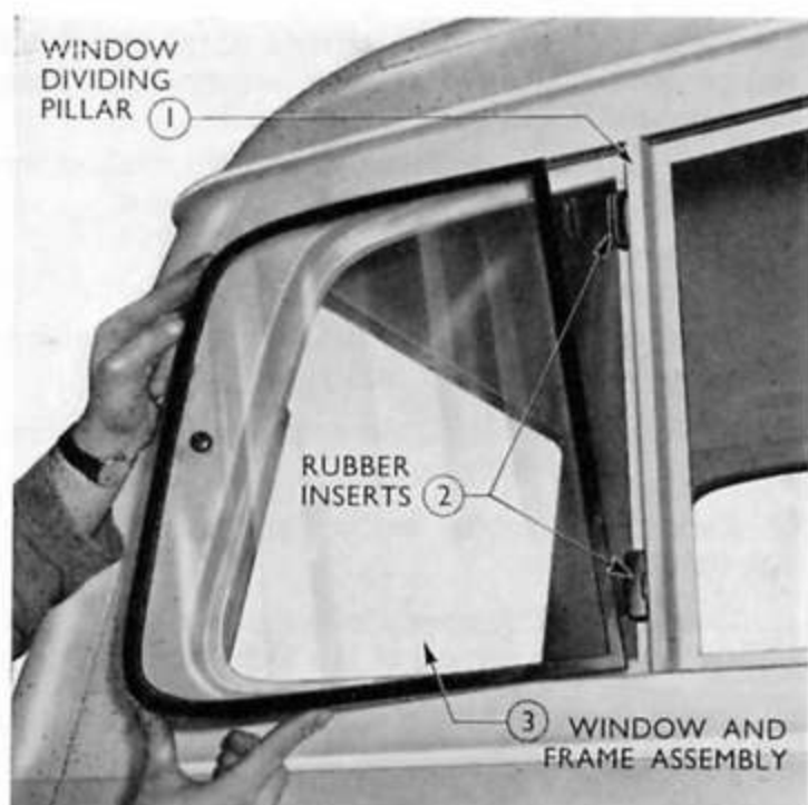
Fig. 11 Hinged Window and Frame Assembly
