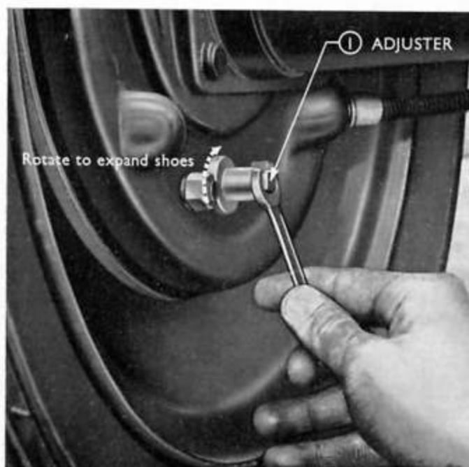
Fig. 8 Adjusting Rear Brakes 75 — 115
