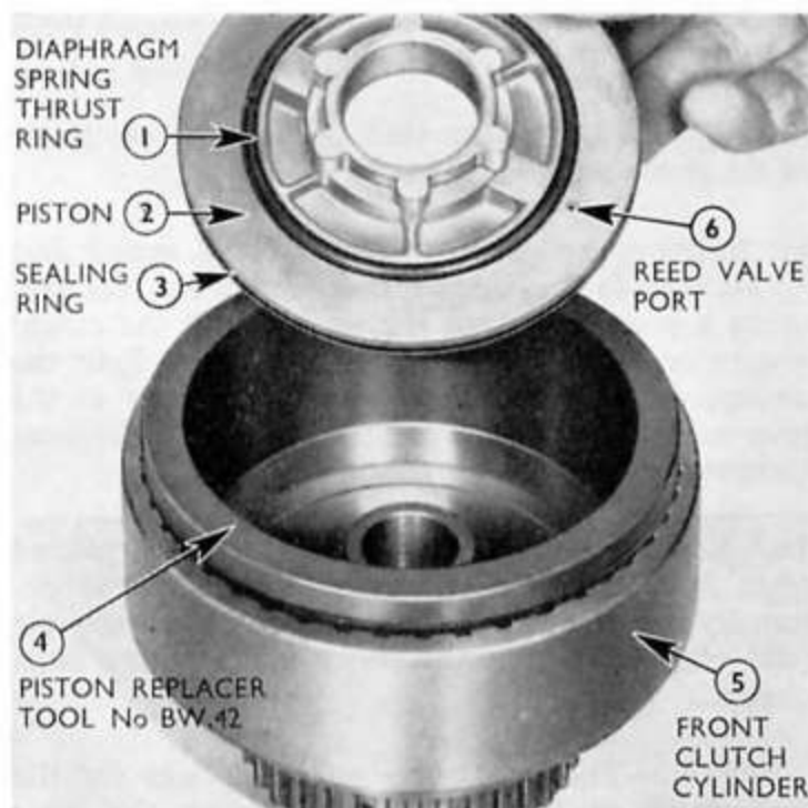
Fig. 45 Replacing Front Clutch Piston
