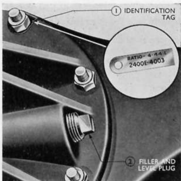
Fig. 1 Filler and Level Plug
