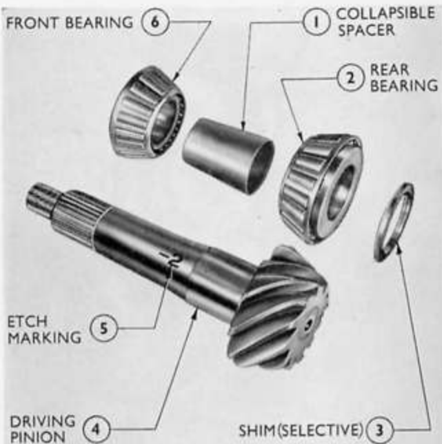
Fig. 13 Drive Pinion Components
