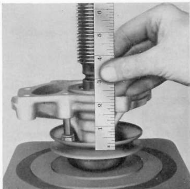
Fig. 6 Fitting the Pump Pulley
