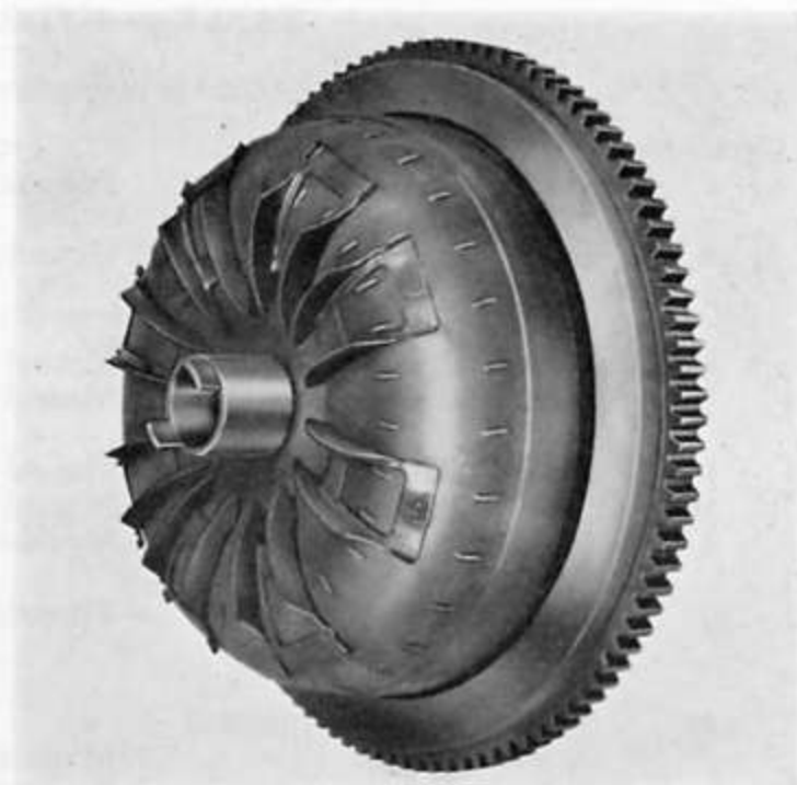
Fig. 39 Torque Converter and Ring Gear Assembly
