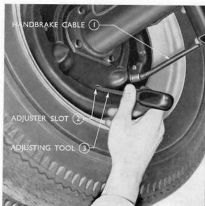
Fig. 9 Adjusting Rear Brakes 125 — 175
