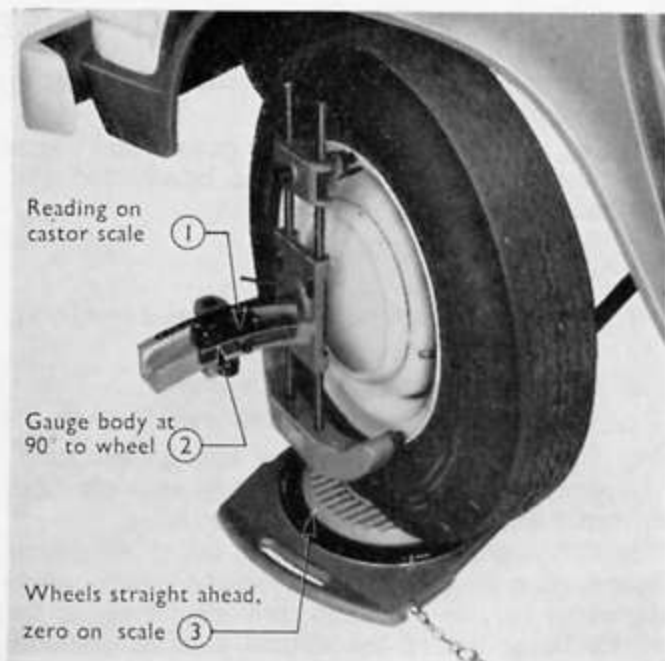
Fig. 16 Castor Angle
