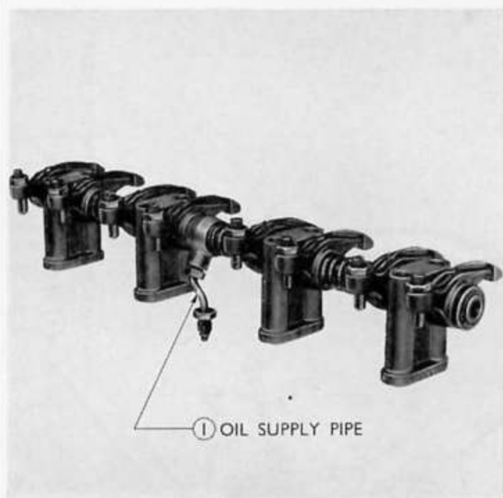
Fig. 38 Rocker Shaft Assembly
