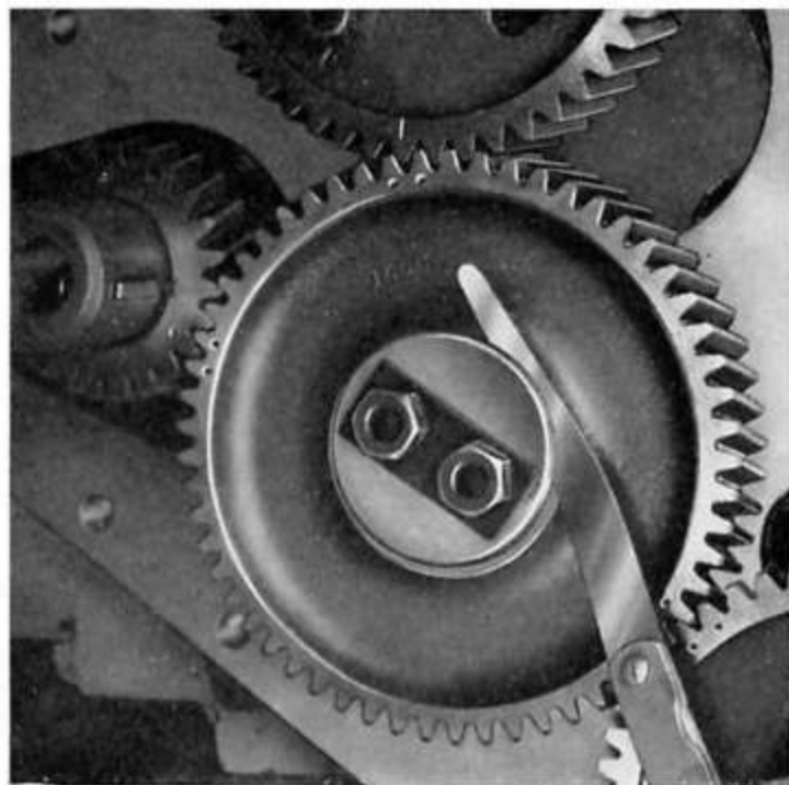
Fig. 53 Idler Gear End-float
