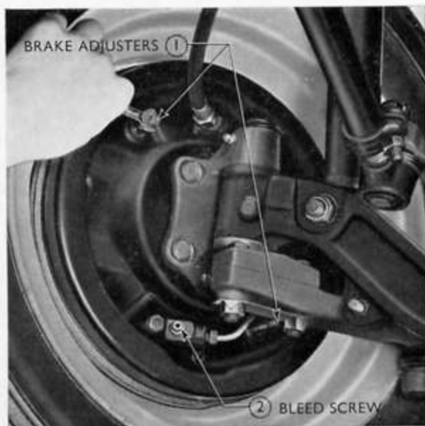
Fig. 7 Adjusting the Front Brakes
