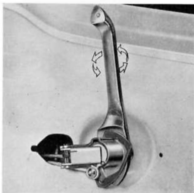
Fig. 2 Removing the Door Handle
