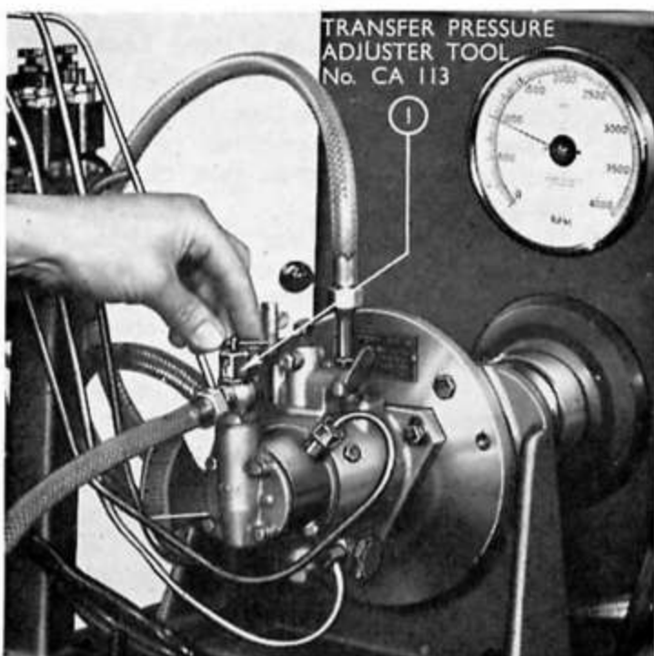
Fig. 47 Adjusting Transfer Pressure
