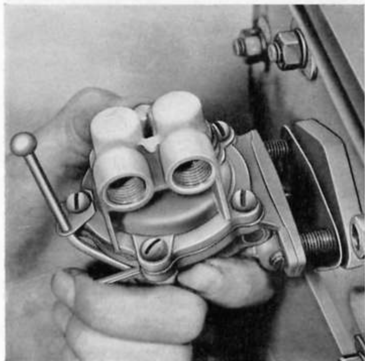
Fig. 45 Fuel Lift Pump
