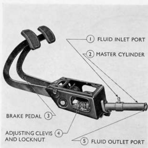
Fig. 17 Pedal Assembly (Floor mounted pedals)
