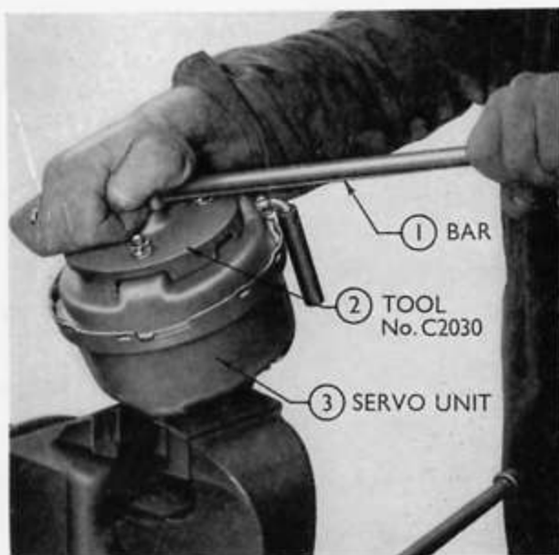
Fig. 25 Separating the Shell
