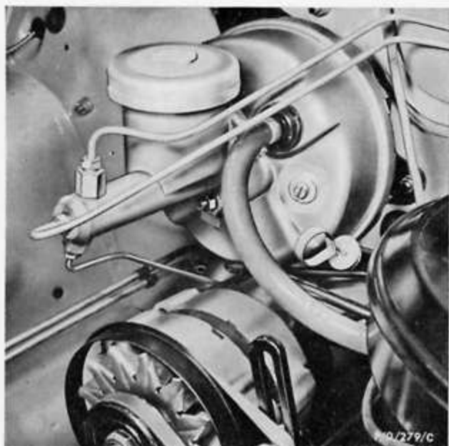
Fig 4 Fluid Reservoir Location (Pendant Pedal Vehicles)
