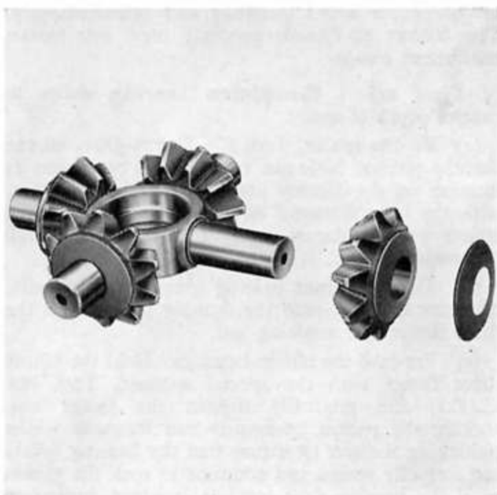
Fig. 23 Pinion Gears and Spider
