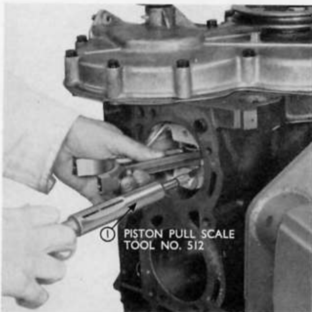
Fig. 17 Checking Piston Fit
