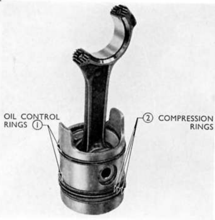
Fig. 43 Piston and Connecting Rod
