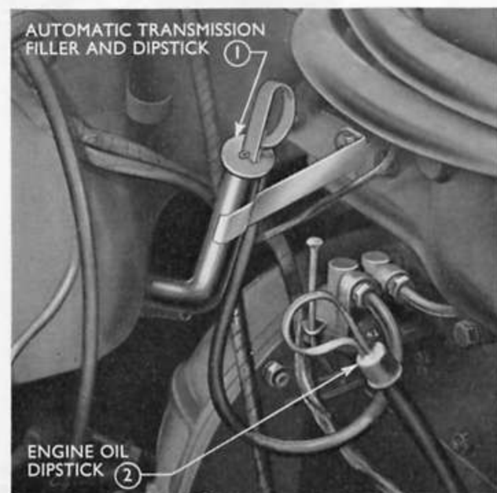
Fig. 30 Dipstick and Filler Tube (Diesel shown)
