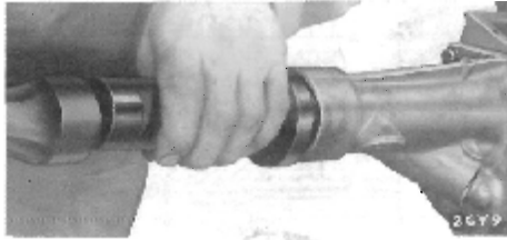
Fig. 47. Fitting the rear oil seal
