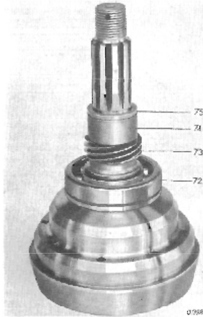
Fig. 21. Annulus prior to fitting to rear casing
