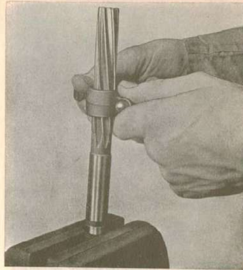
Fig. 1-39. Reaming a new bushing
