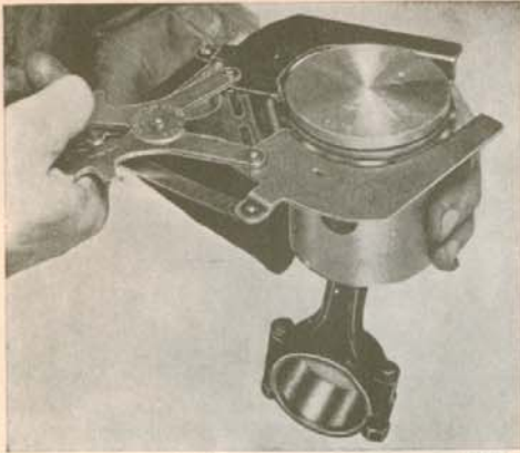
Fig. 1-47. Fitting the piston rings
