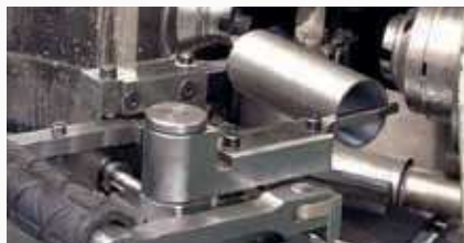
Grinding the piston ring sliding surface
