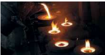
Casting process for piston ring castings (die casting)
